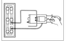
Since disconnecting the motor lead opens the pull-in coil of the solenoid, it will be necessary to assist the movement of the plunger by hand. Make sure the plunger reaches its extreme travel position, closing the switch contacts. The cranking motor armature will not revolve with the motor lead disconnected. The pinion travel can be checked by pushing the pinion back against the spring pressure with a scale and measuring the relative movement between the pinion and the casting.
