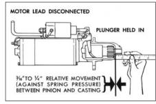
The adjustment can be changed by turning the plunger stud in or out of the solenoid plunger as necessary. One-half turn of the stud will change the adjustment 1/16 of an inch. On manually shifted units, the travel of the pinion against the pinion spring may be adjusted by loosening the locking nut and turning the adjusting stud on the shift lever as required.
