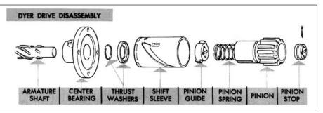
Engagement of the pinion while in motion would be impossible because of the high horsepower developed and the acceleration of the armature when the cranking circuit is completed.
