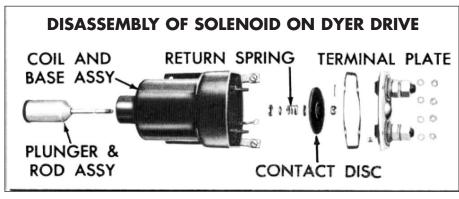
cranking motors have a replaceable contact disc which is adjustable. The location of the disc when assembled should be 1 1/32 inches below the edge of the housing with the plunger in a retracted position. This position is important to assure proper pressure between the contact disc and the terminal contacts while cranking.
