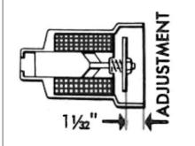
Since the Dyer drive is designed to engage the pinion with the flywheel ring gear before the cranking circuit is completed, the pinion travel adjustment is very important. This adjustment was covered under the subject of Dyer drives.
