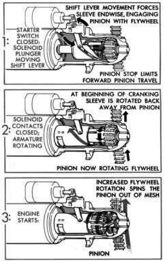
It is impossible to start another cranking cycle without completely releasing the shift lever. The lever must drop all the way back to the at-rest position. With pedal operated shift levers it takes a few seconds to perform this operation. Solenoid operated shift through the solenoid to hold the shift lever in the forward position.
