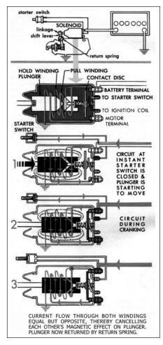
When the circuit is completed to the solenoid, current from the battery flows through two separate windings, designated as the "pull-in" and the "hold-in" windings (1). These windings produce a combined magnetic field which pulls in the plunger so the drive pinion is shifted into mesh and the main contacts in the solenoid switch are closed.
