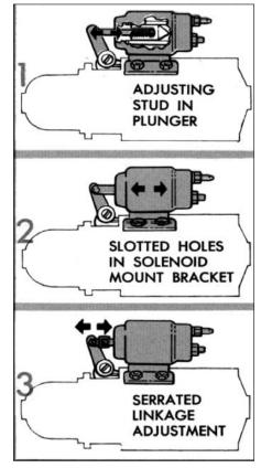
The pulling power of a solenoid increases at an increasing rate as the air gap of the plunger is reduced. Locating the pinion adjustment to the high limit, on either the clutch or Dyer drive type motors, will, in effect, reduce the air gap and a more powerful magnet is obtained. Never replace a solenoid on a motor without checking pinion clearance. Satisfactory performance depends upon this adjustment.
