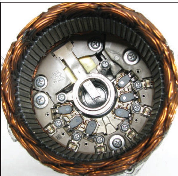
Figure 9 – There are no soldered connections. #2 Phillips machine screws are used. A worn Phillips bit will not break them loose.
