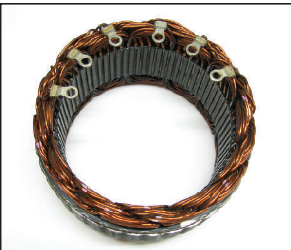
Figure 10 – They use a double wound stator, common on many other Mitsubishi alternators.
