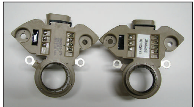
Figure 5 – The regulators appear to be identical but note the different part numbers.
