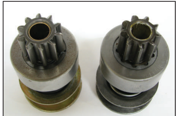
Figure 1 – The drive on the right is a common 207, while the Jammit drive's pinion on the left has an extra tooth and is 1/10th of an inch larger to solve “too much clearance” problems on 10MT pad mount starters.
