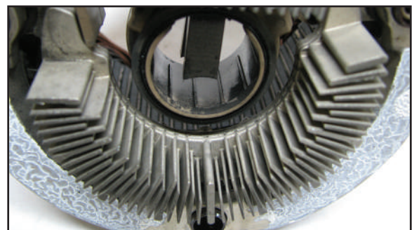
Figure 12 – Notice the number, size and design of the positive heat sink.
