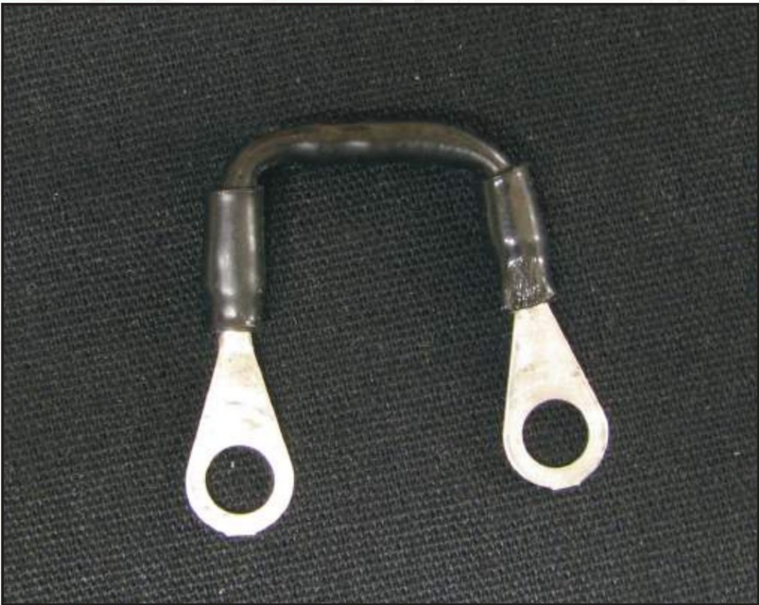
Figure 2 – Black 560ohm resistor used in 34SI alternators.
