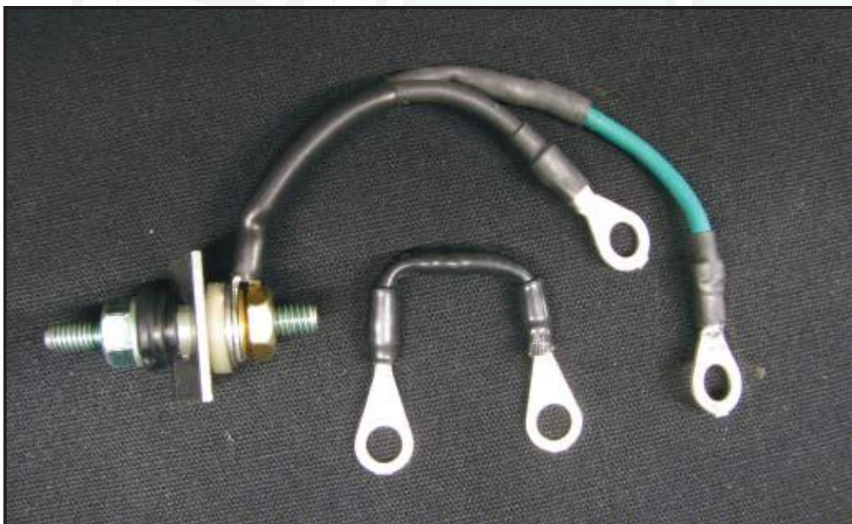
Figure 3 – New 36SI sense terminal package above the 34SI resistor.
