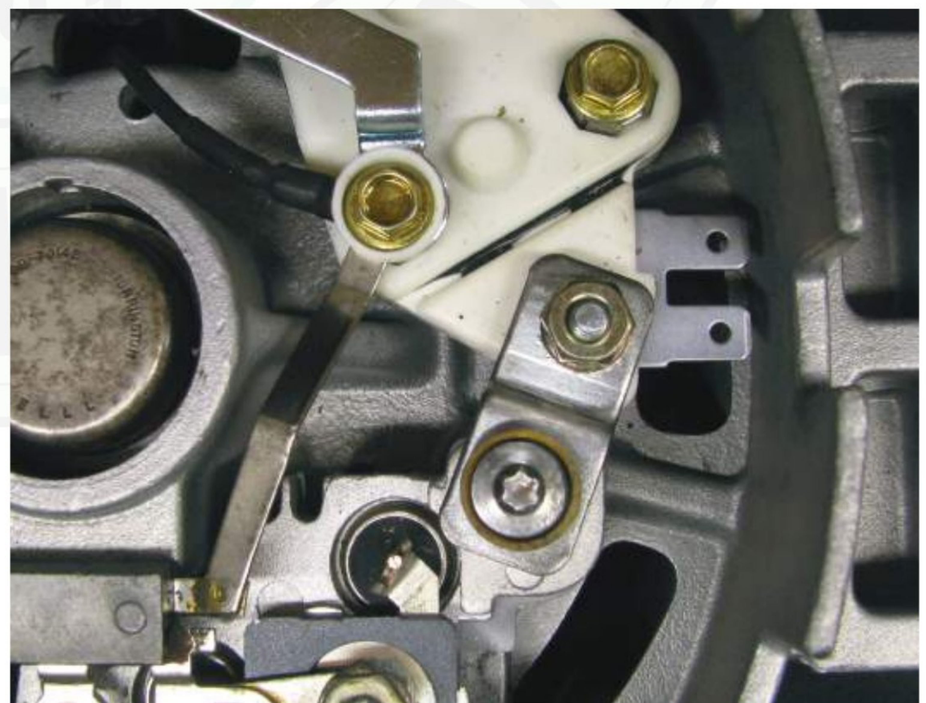
Figure 5 – B+ strap can be used only when voltage drop to batteries is minimal.
