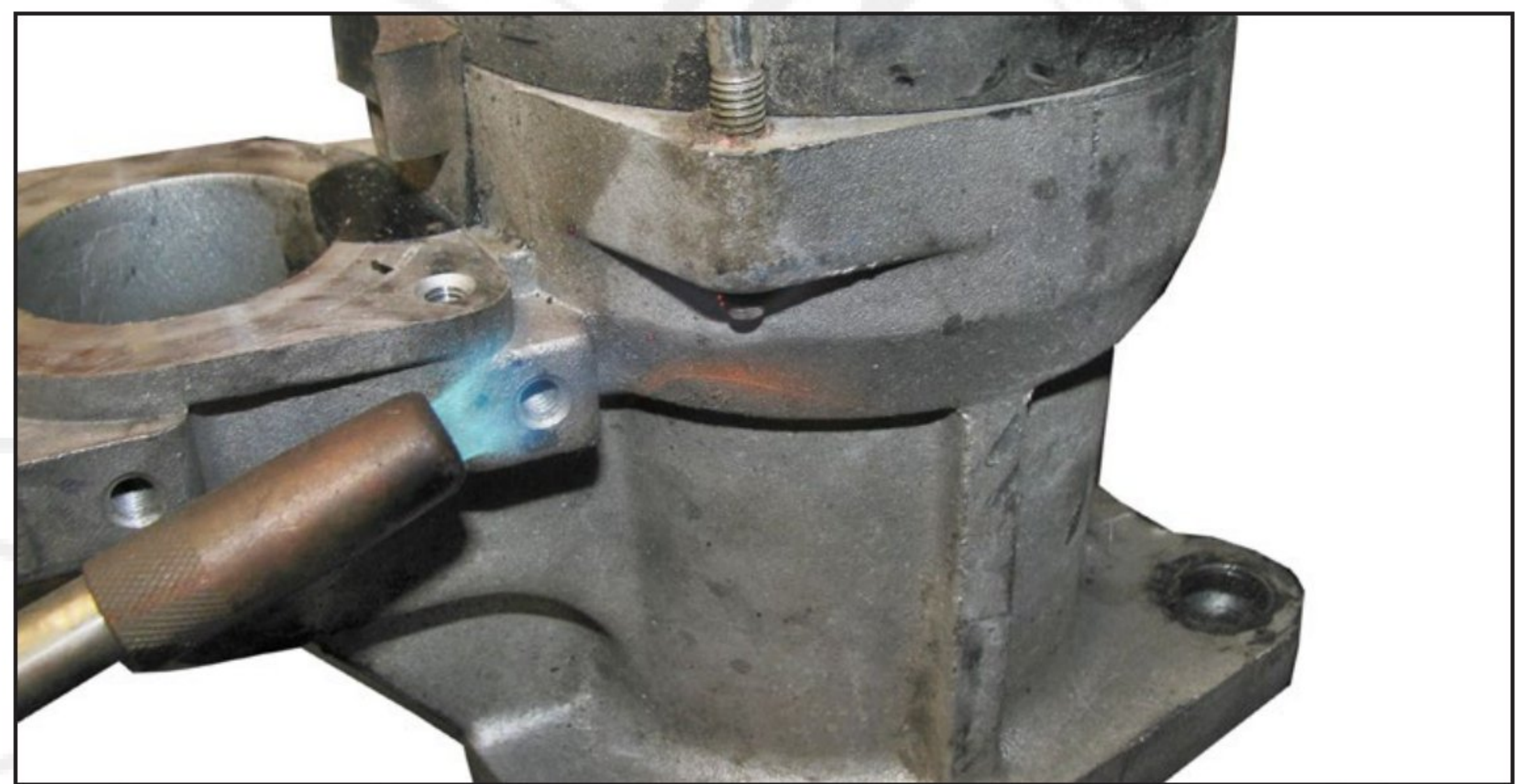
Figure 9—Permanent thread-locking compound must be heated prior to removal of the through bolts during disassembly.
