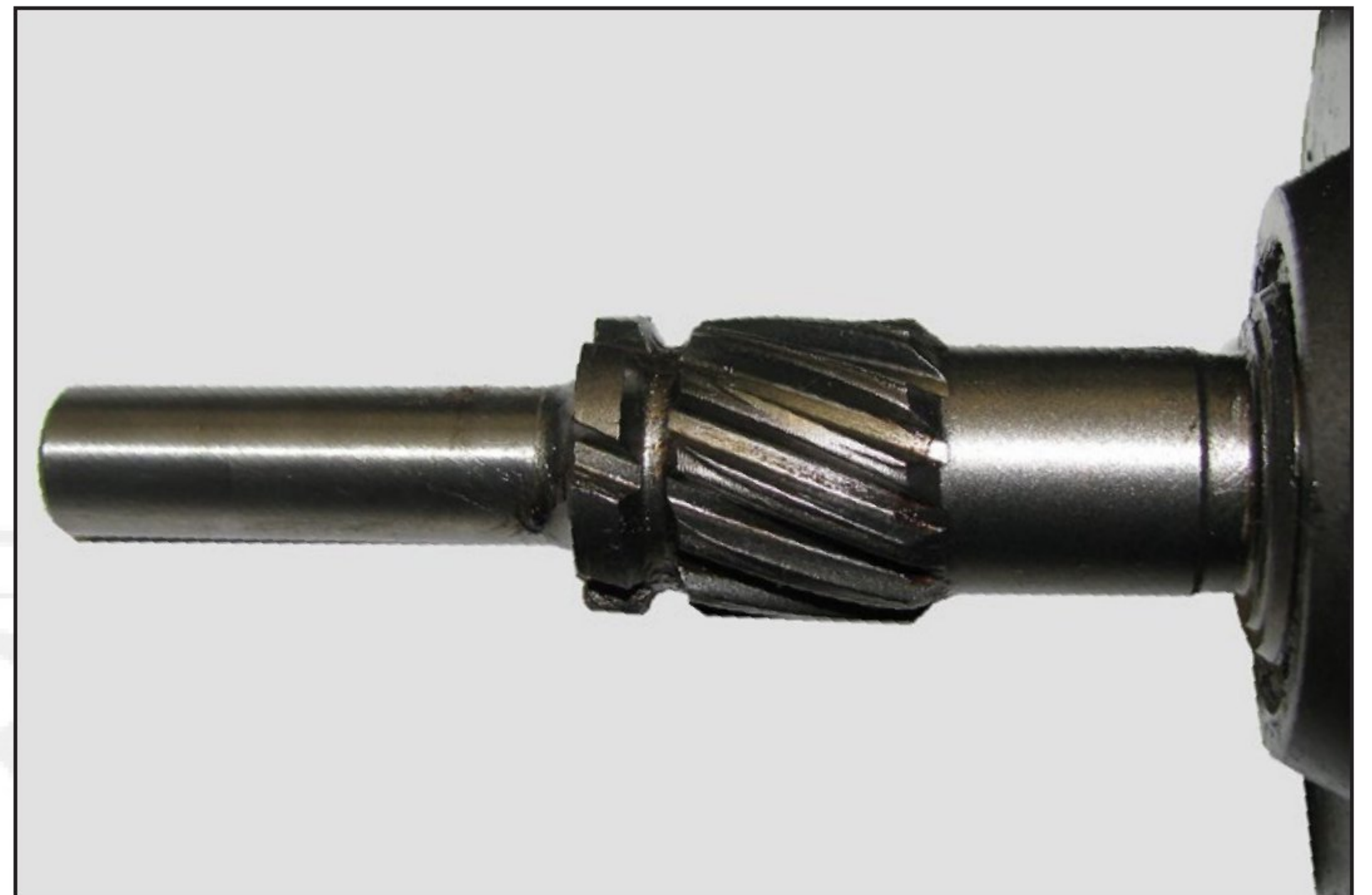
Figure 15—Note that every other spline on the 39MT shaft is blind. The drive must be on a blind spline when it is reassembled.
