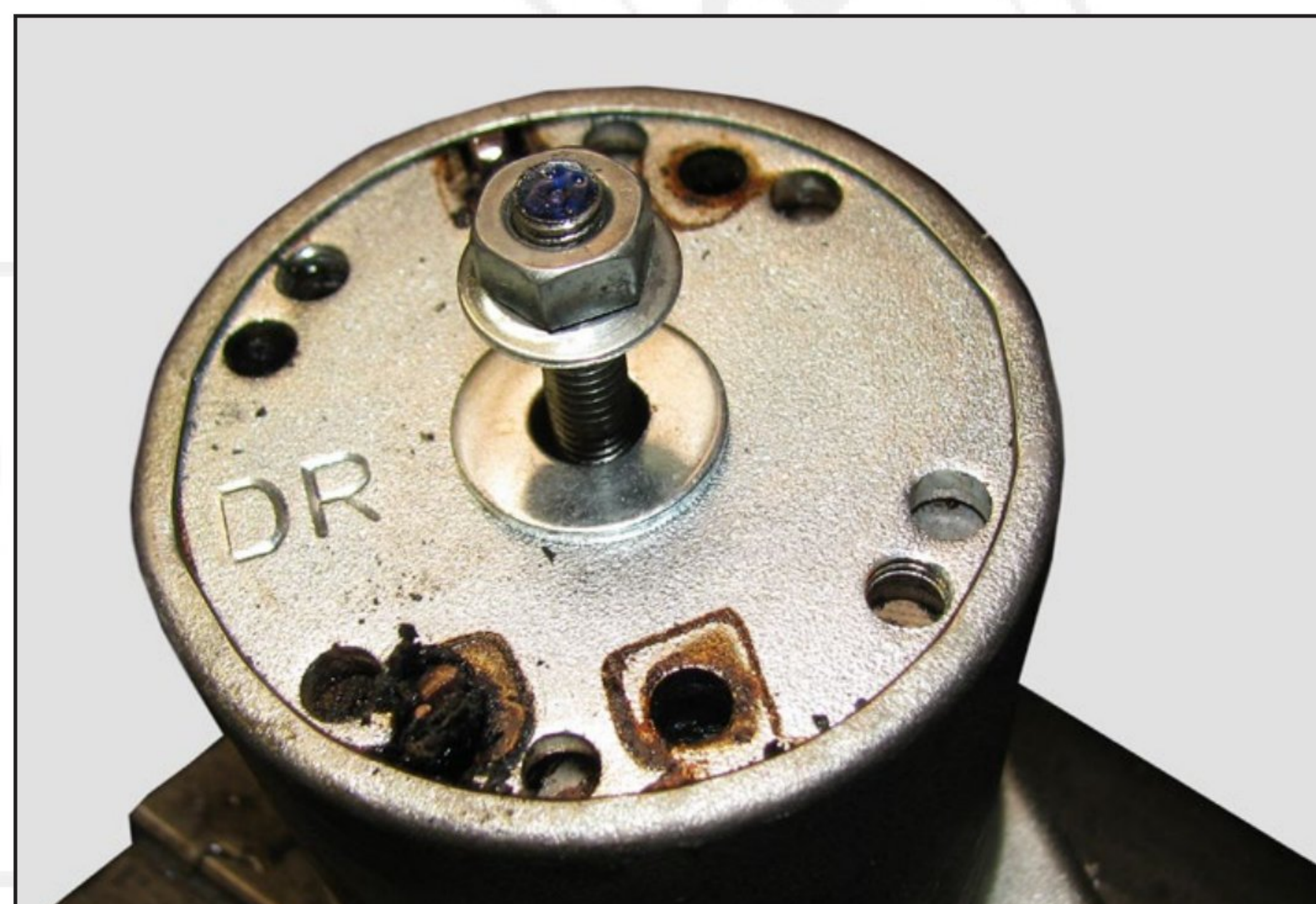
Figure 14—The large flat washer and nut complete the tool. You can now install it on a starter and tighten the nut to extend the drive for pinion removal.
