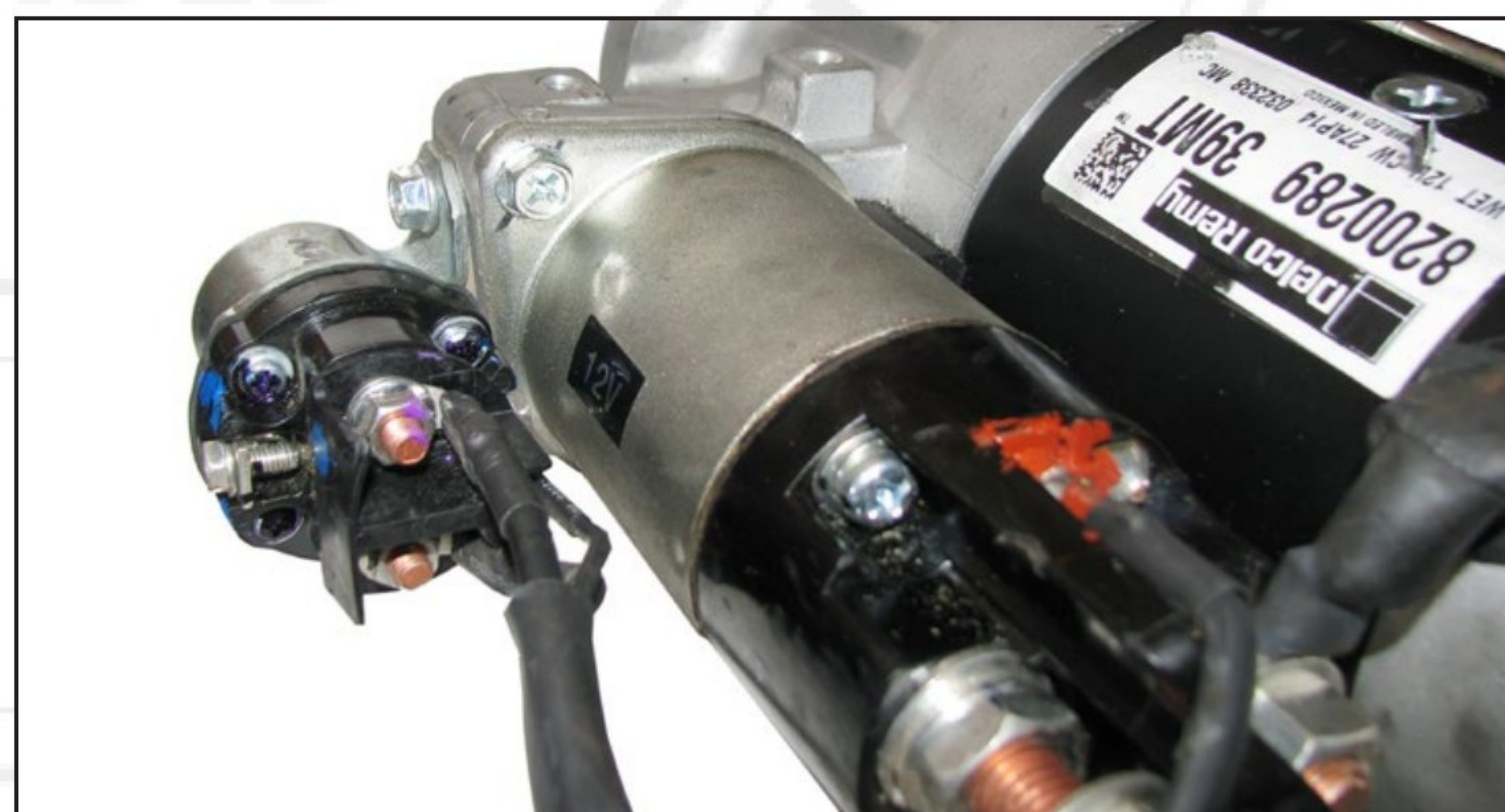
Figure 4—Generation II, III and IV starters use the same solenoid. Mounting screws thread into the DE housing.
