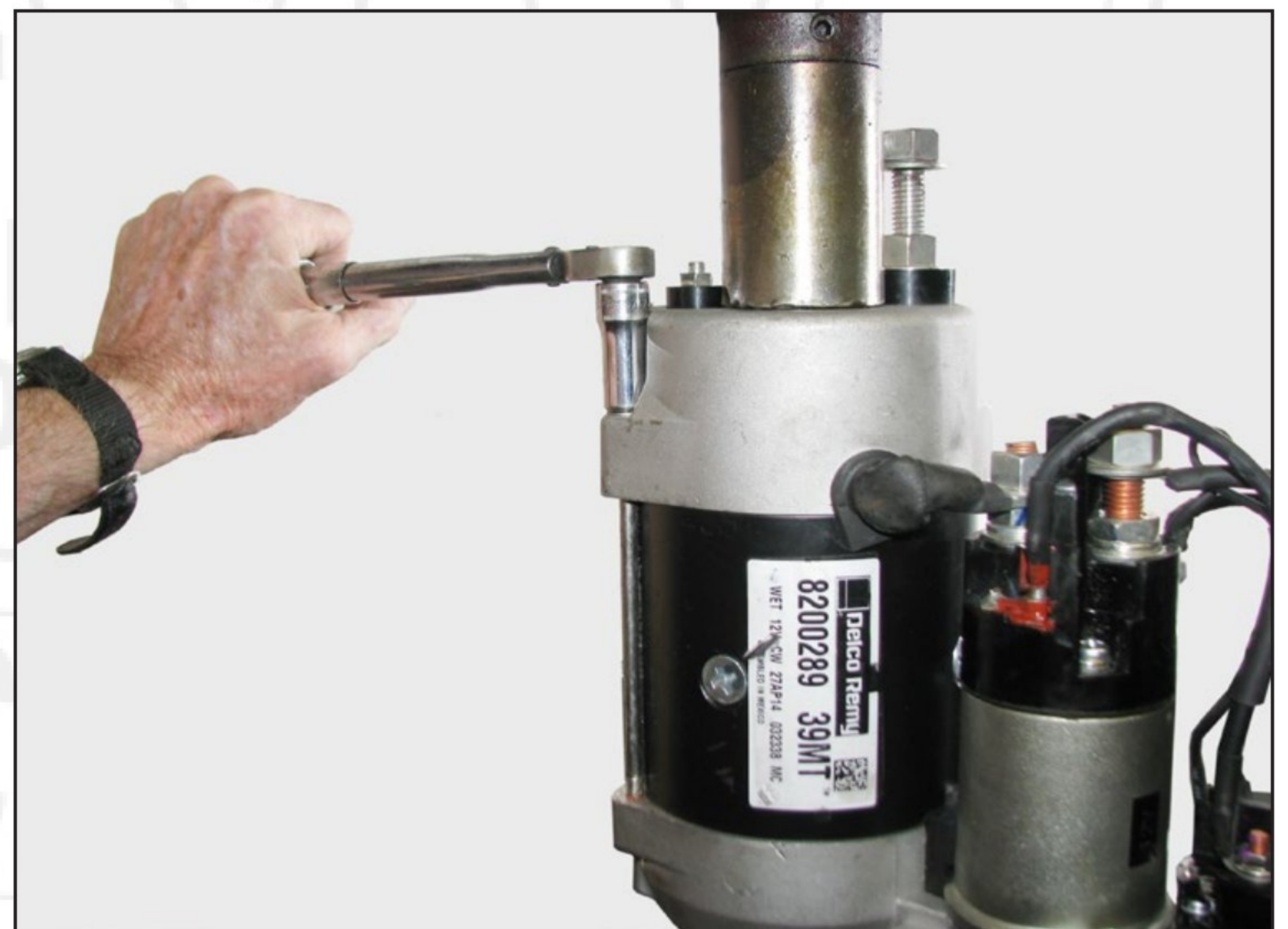
Figure 9—Permanent thread-locking compound must be heated prior to removal of the through bolts during disassembly.
