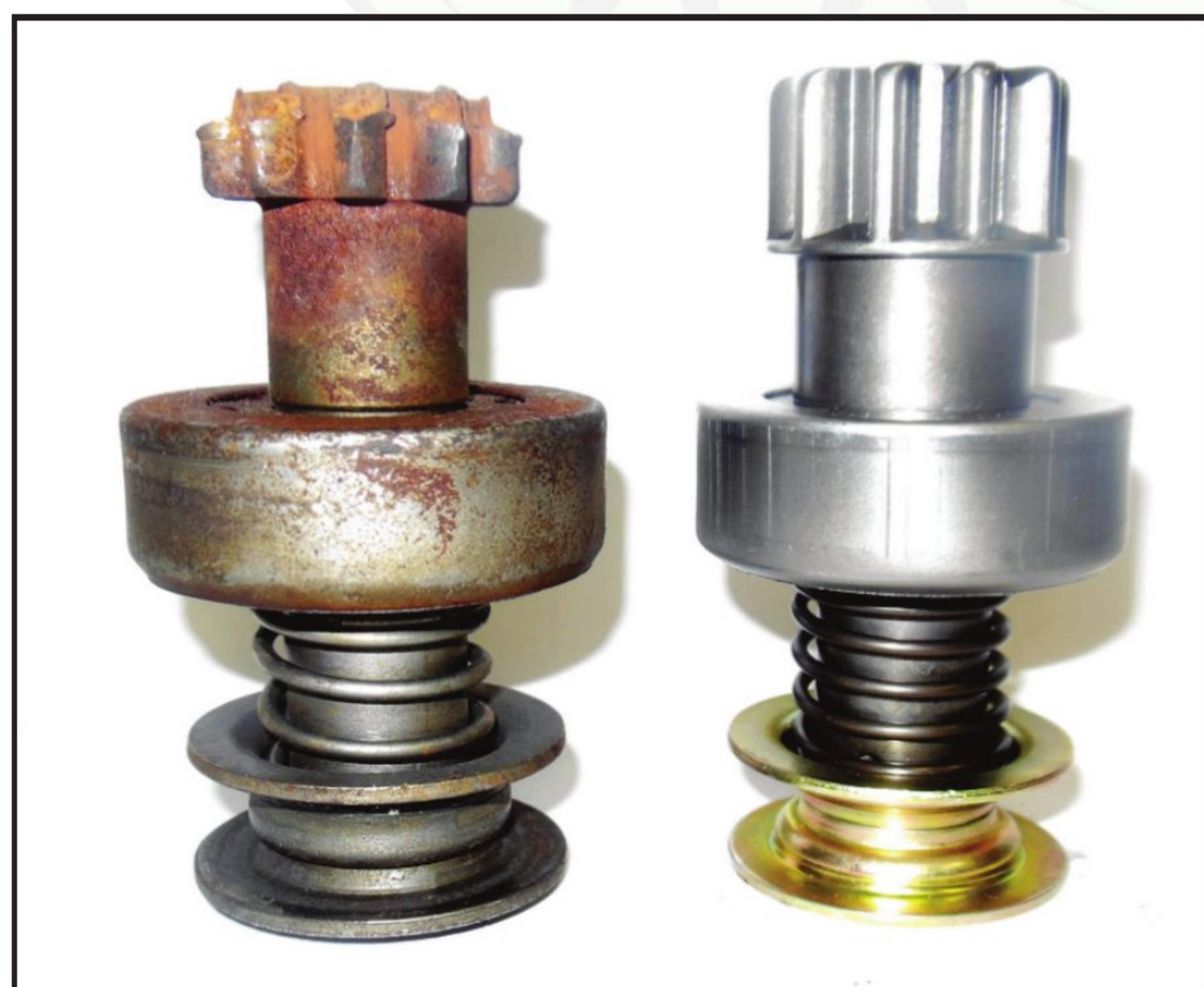
Figure 1 – The old Prestolite drive and the replacement from "The Drive Doctor"
