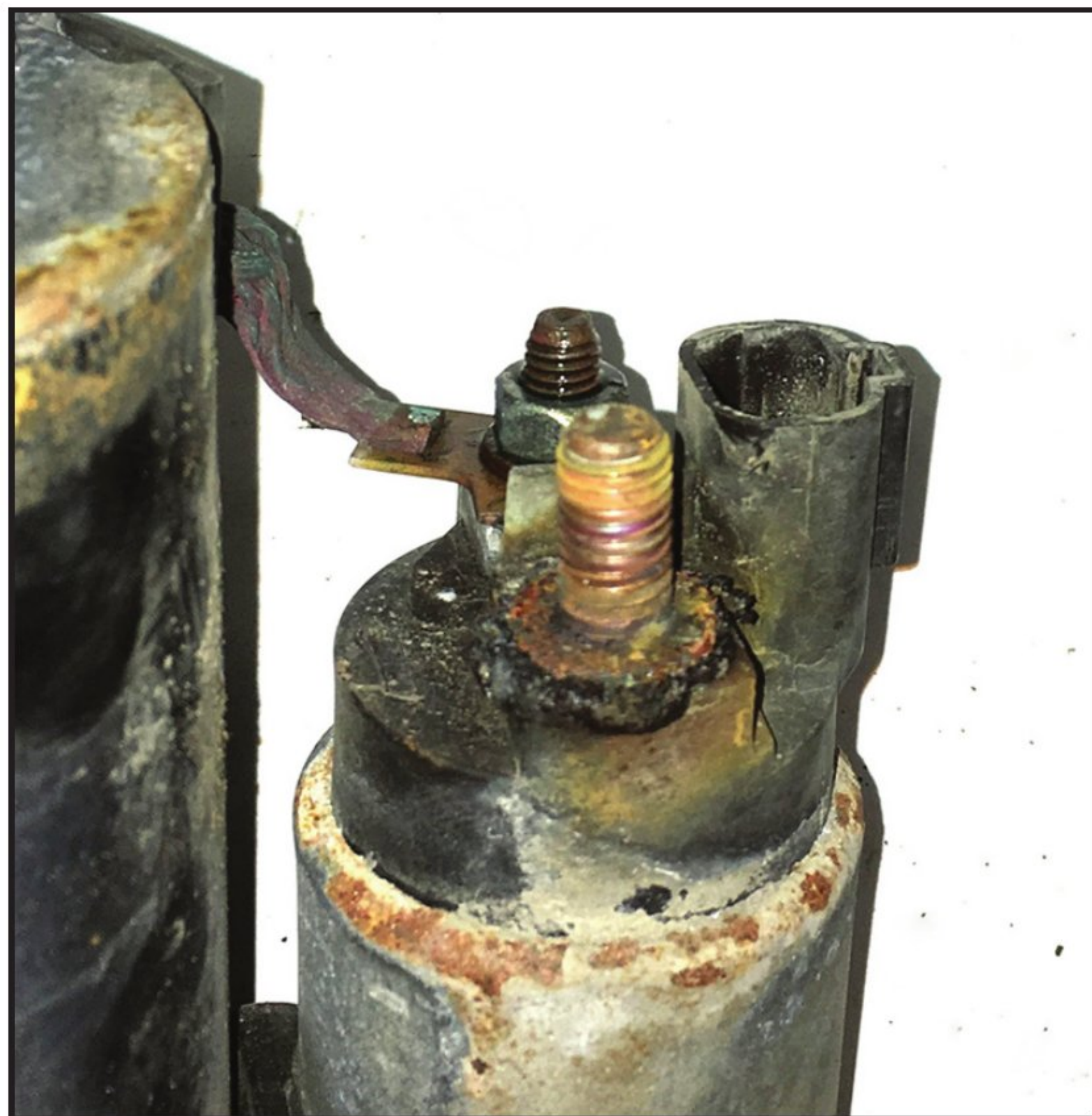
Figure 3 – Deteriorated 17935 starter post due to corrosion and poor connection
