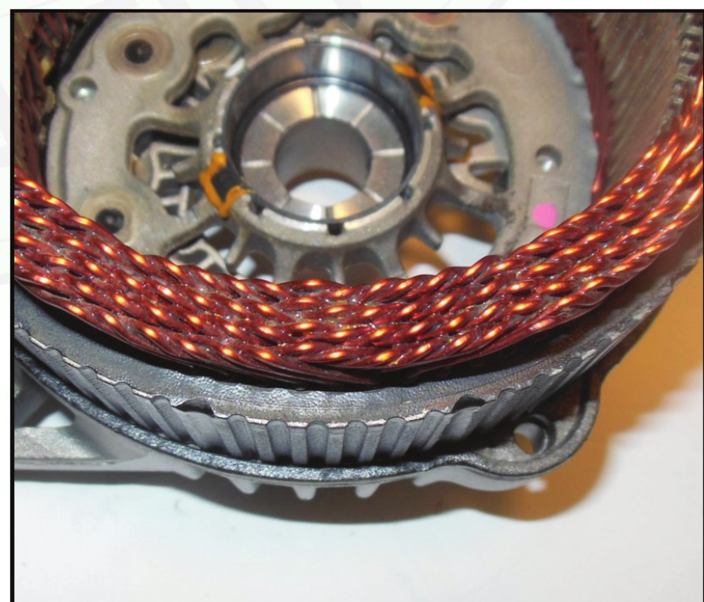
Figure 6 – Multi-row and heavily wound 8487 alternator's stator
