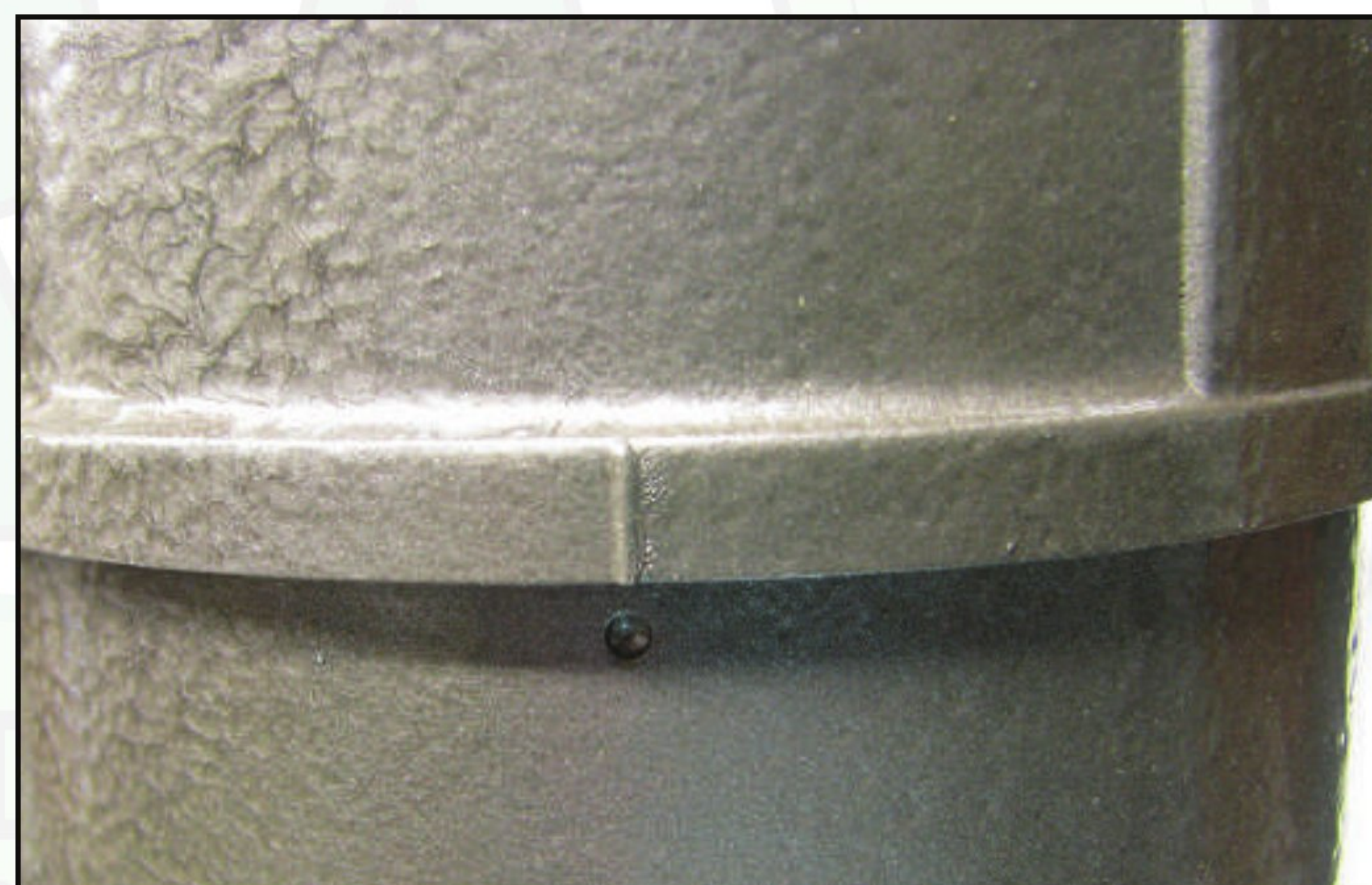
Figure 7 – Some aftermarket 28MT starters employ similar or identical timing marks.
