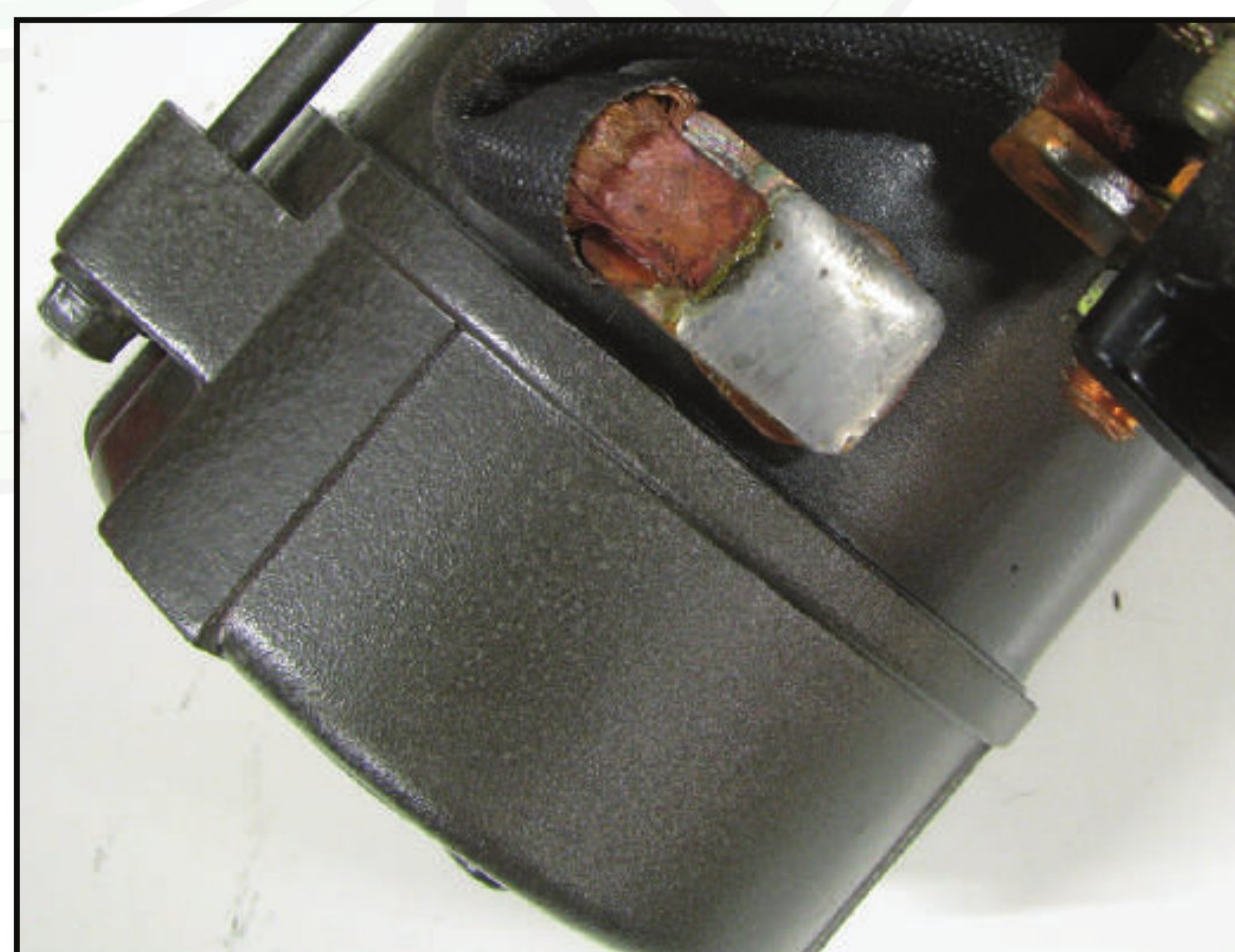
Figure 8 – Many other 28MT replacement starters have no timing marks at all.
