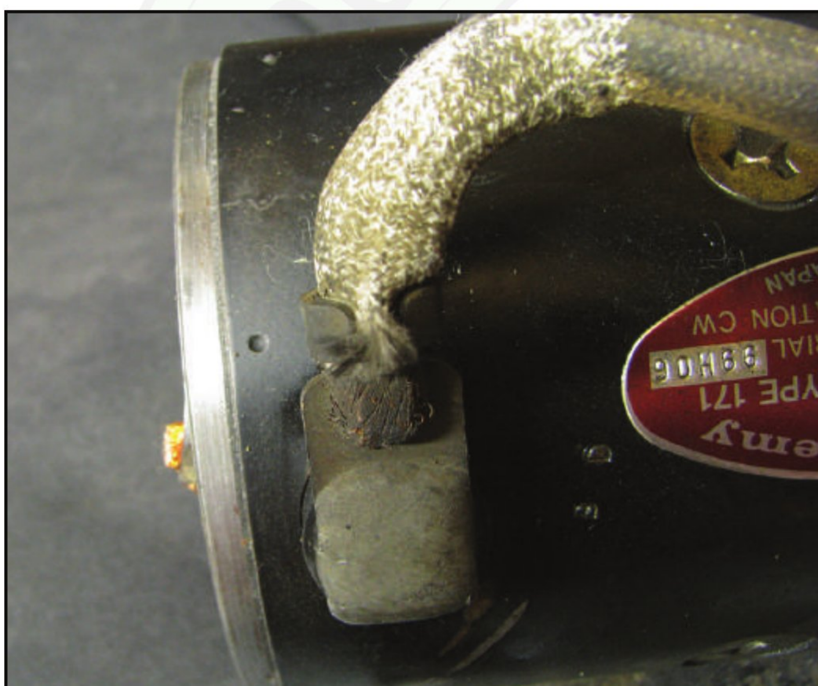
Figure 5 – Original Delco 28MT starters have locator marks on their field cases to achieve perfect brush timing.
