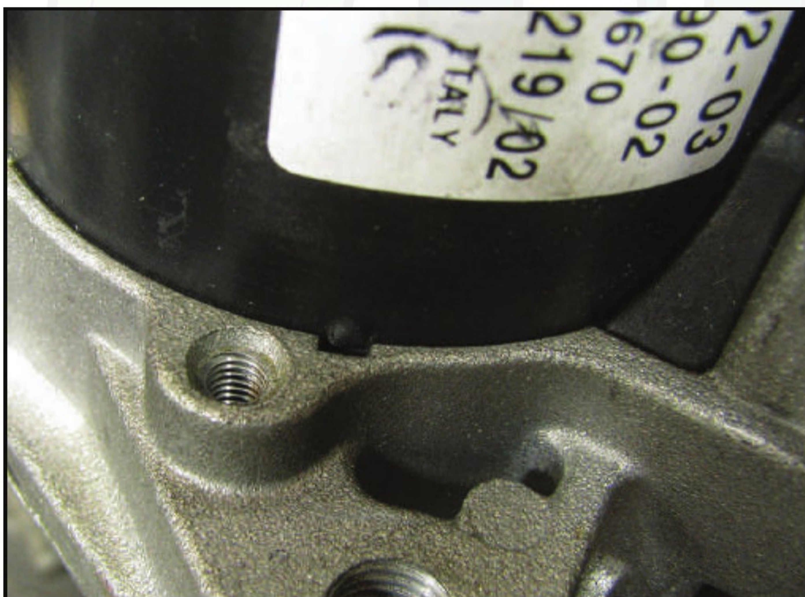
Figure 1 – This Denso starter has protrusions on the field case, here fitting tightly into the drive end housing's indentation.
