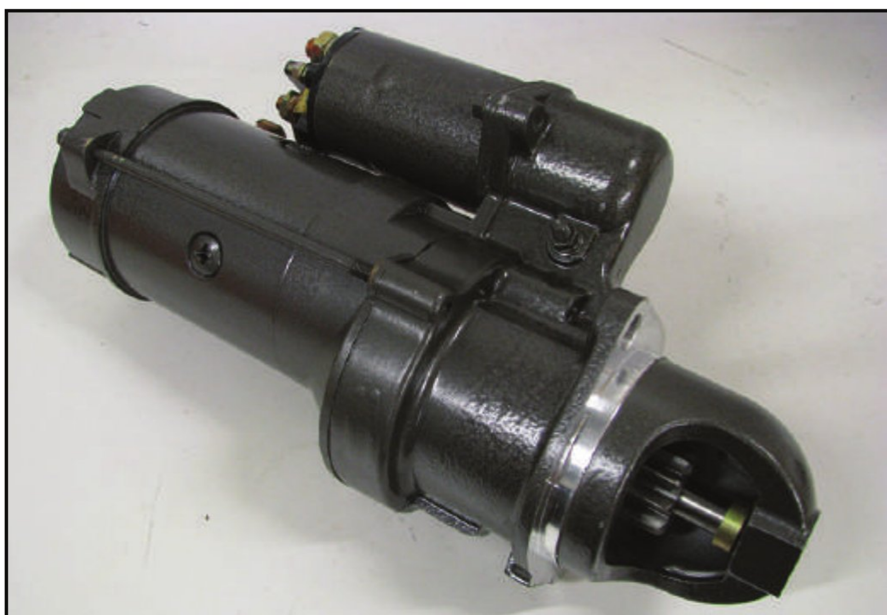
Figure 4 – Some aftermarket 28MT starters present a unique challenge whether inspecting, repairing or rebuilding them.
