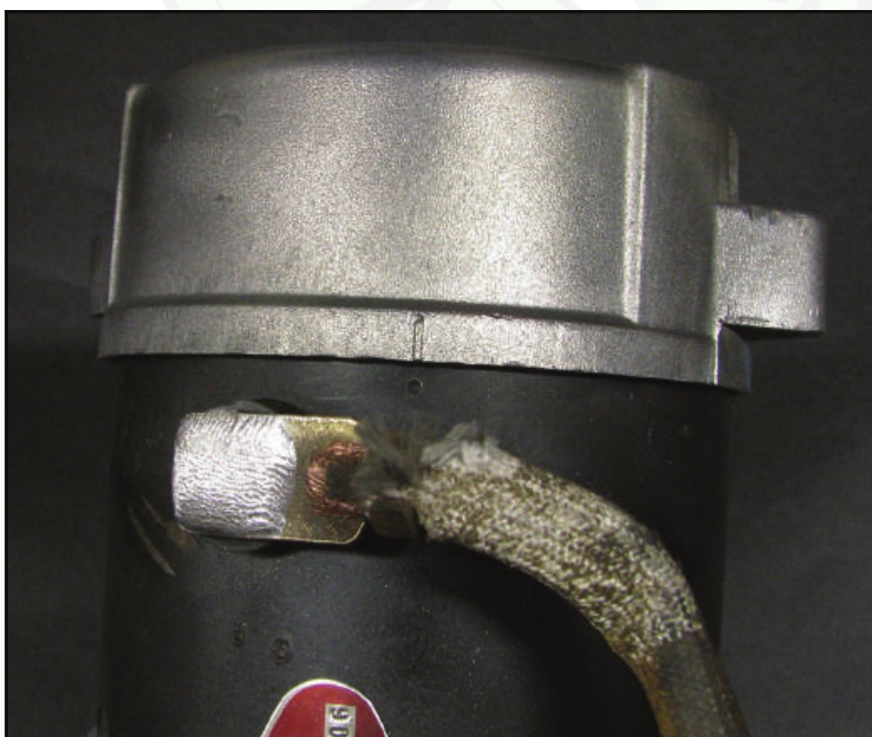
Figure 6 – A raised line cast on the open end of the commutator end housing must be aligned with the case's mark.
