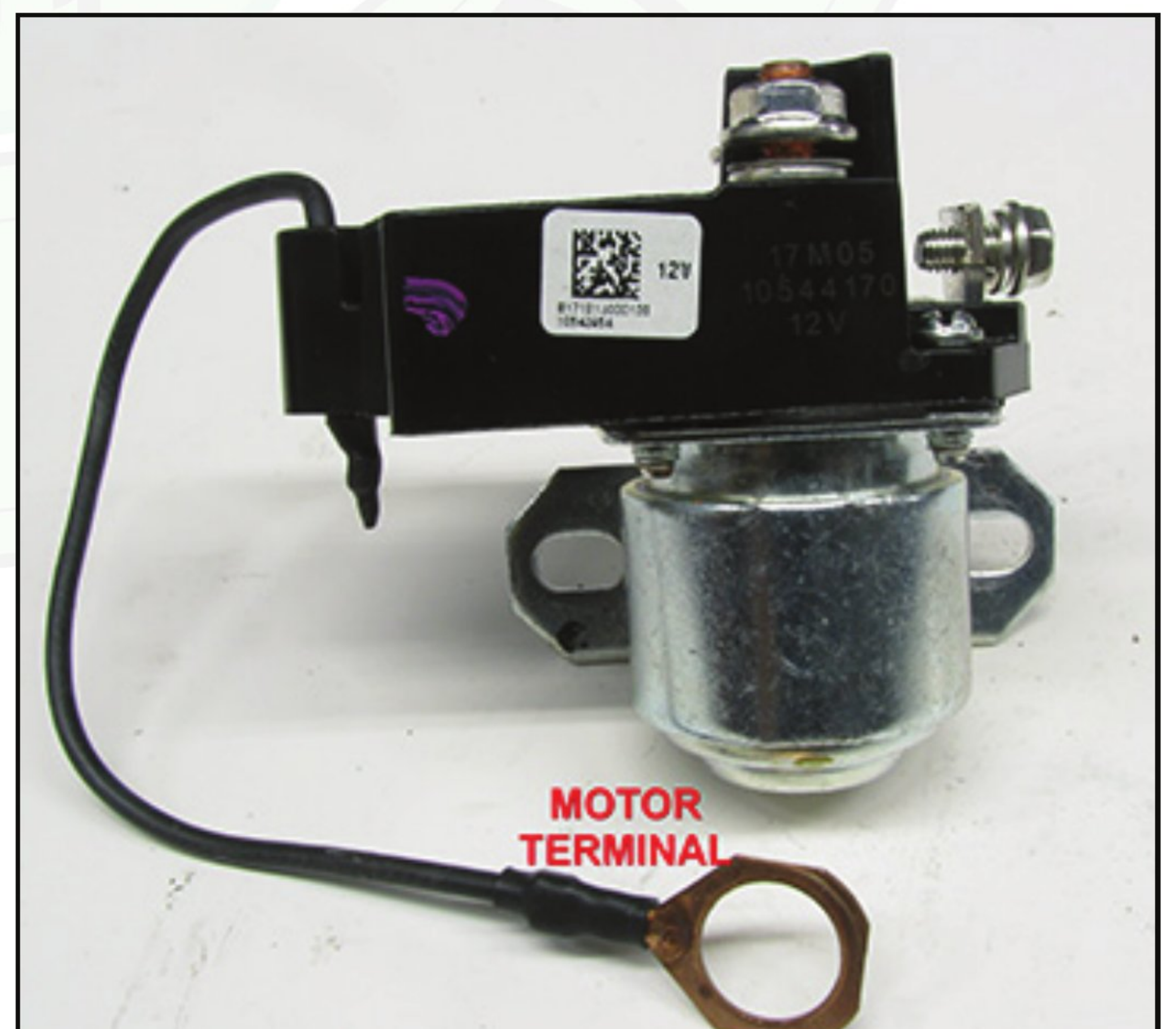
Figure 4 – Smart IMS with motor terminal connection.
