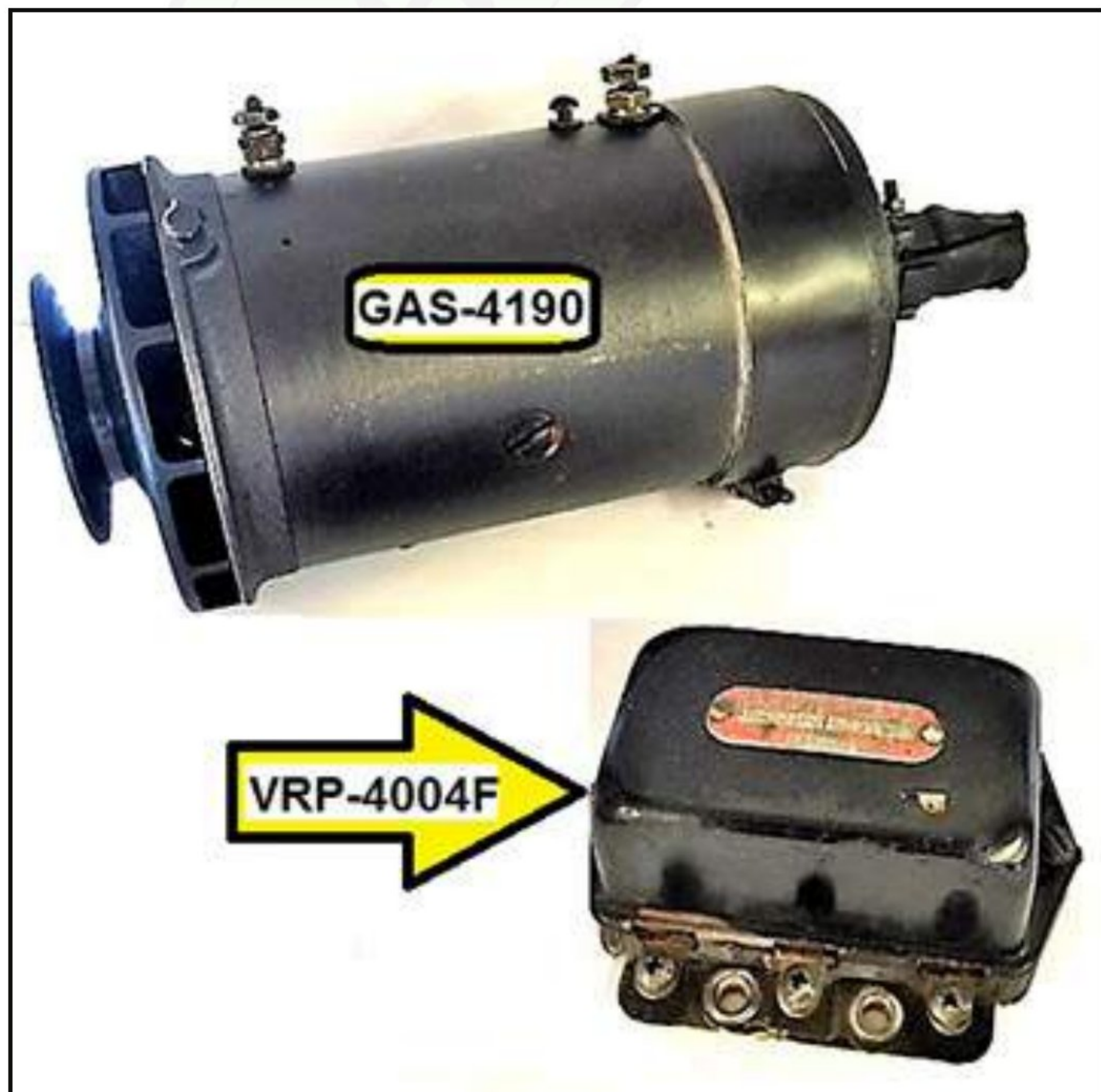
Figure 3 – Crosley's generator and regulator
