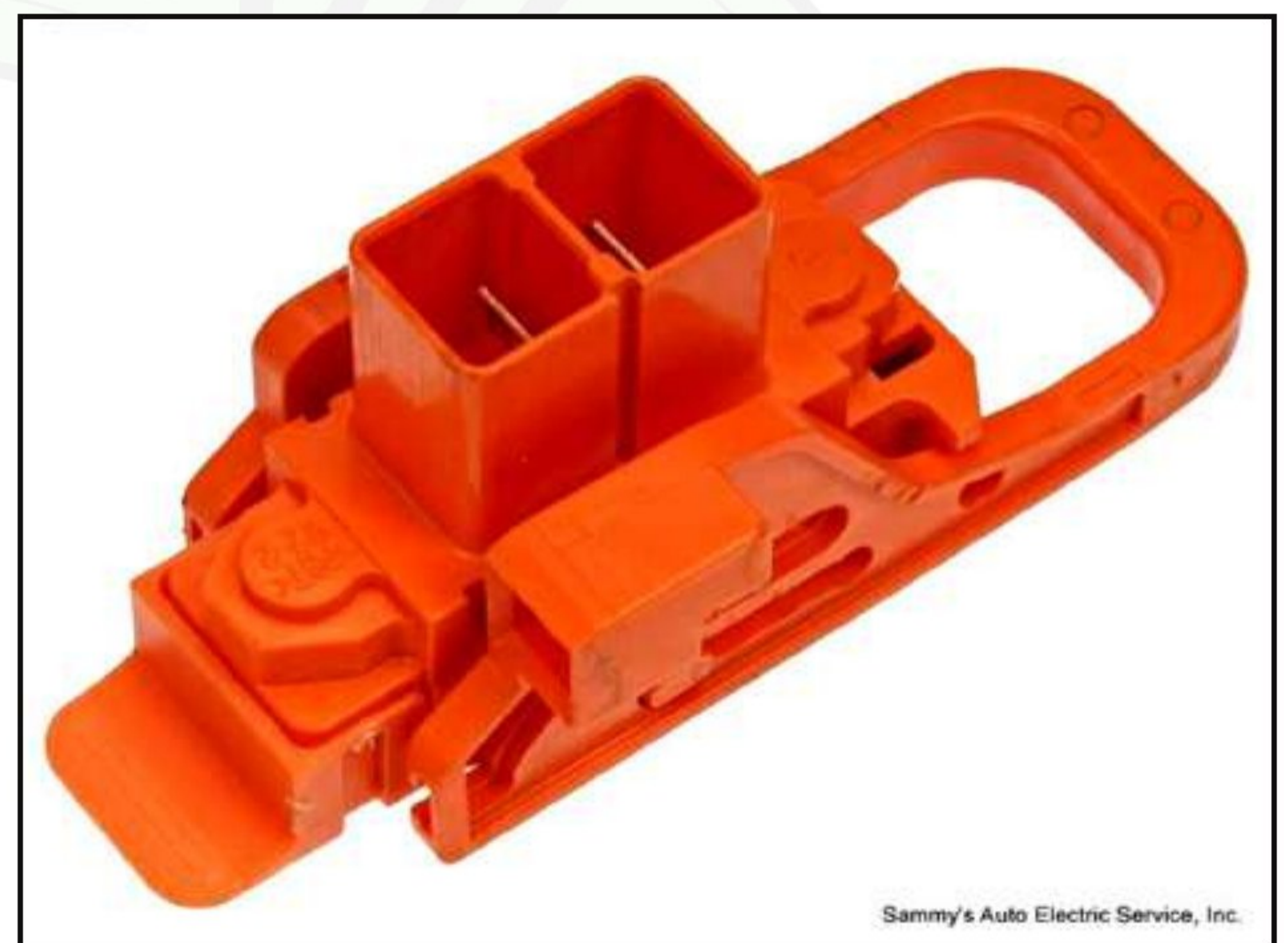
Figure 10 – Service Plug, Removed for any HV Battery Service
