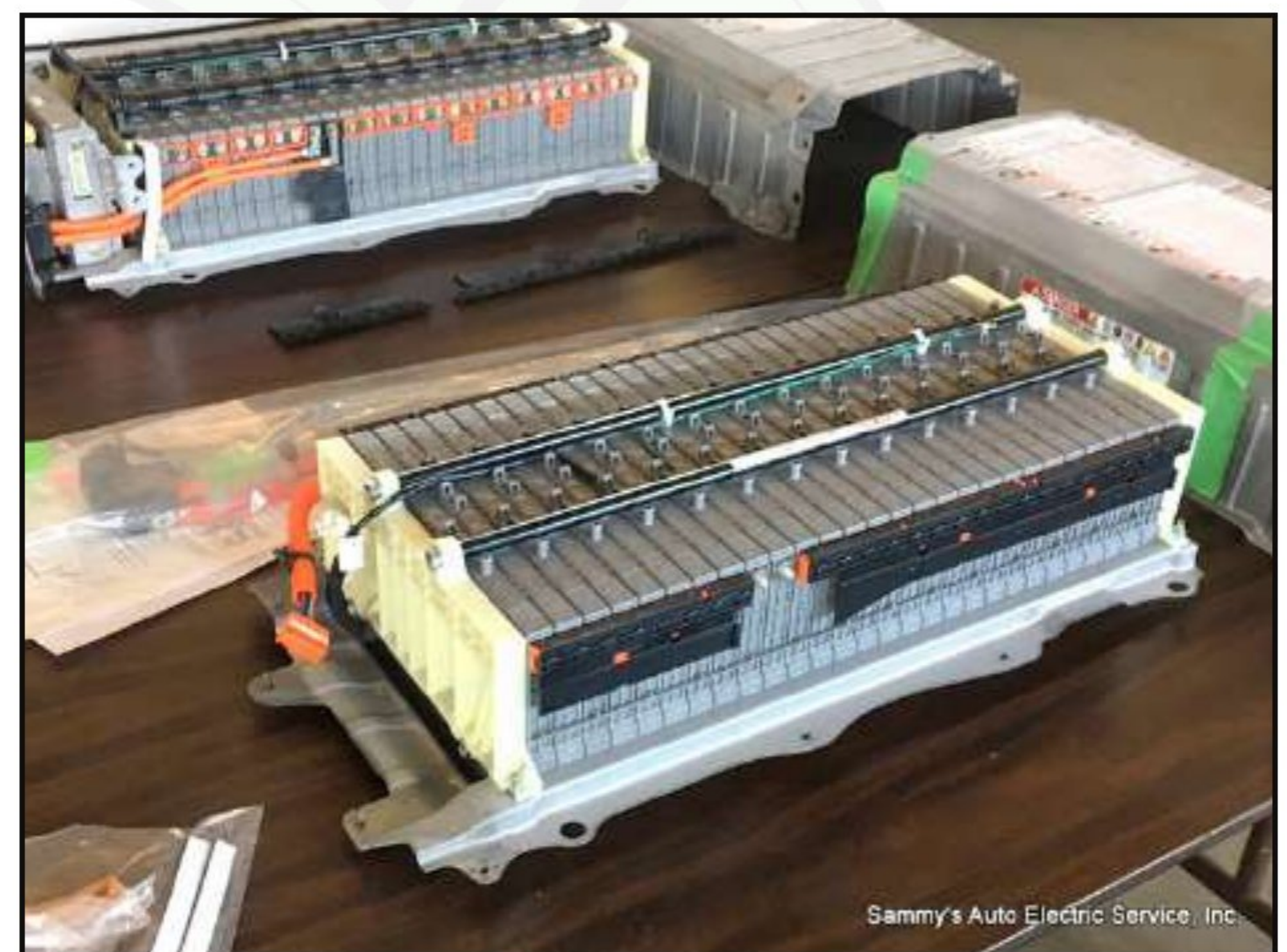
Figure 2 – Old and New Batteries with Covers OFF
