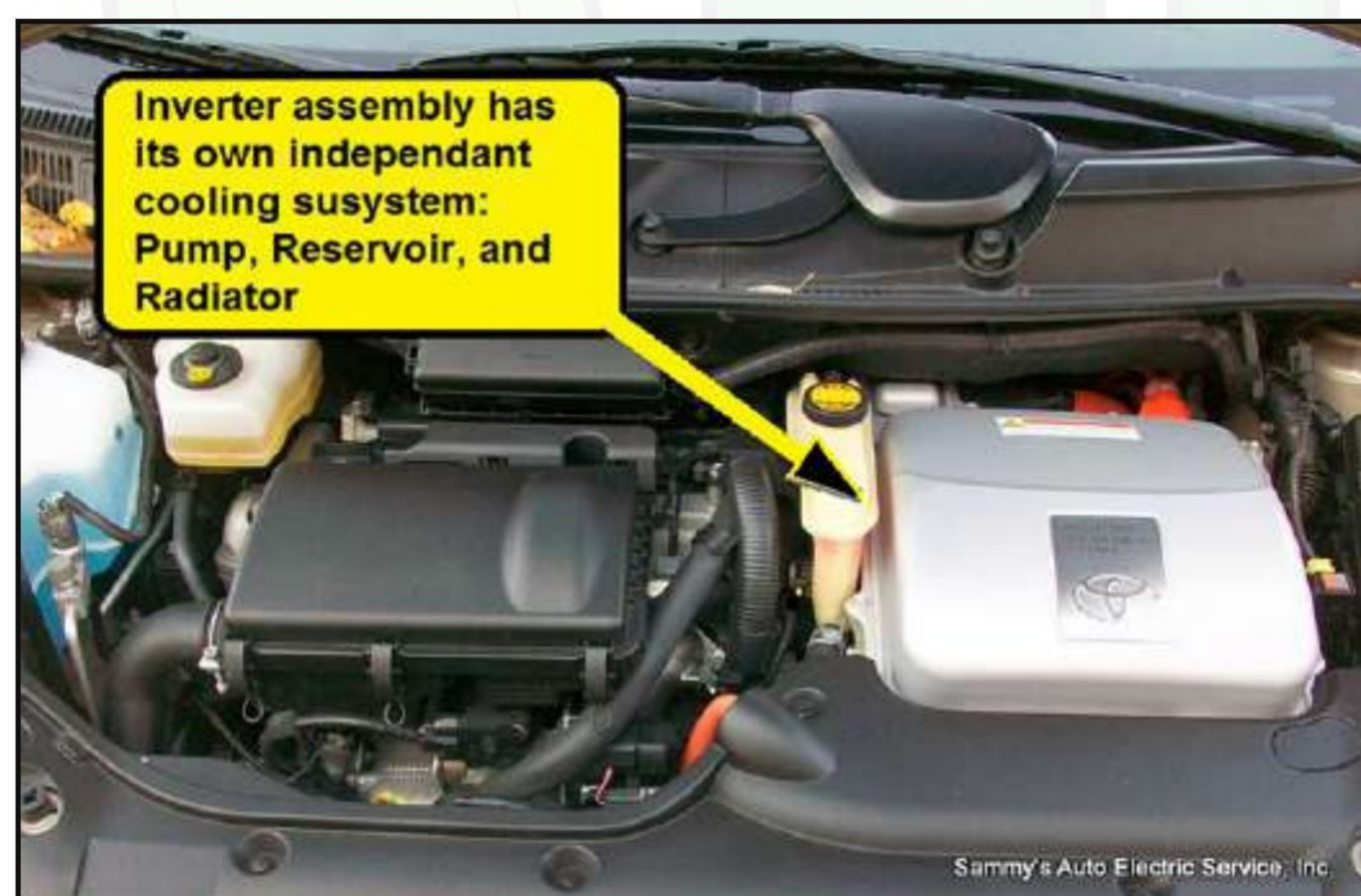
Figure 4 – Inverter Assembly in Engine Compartment
