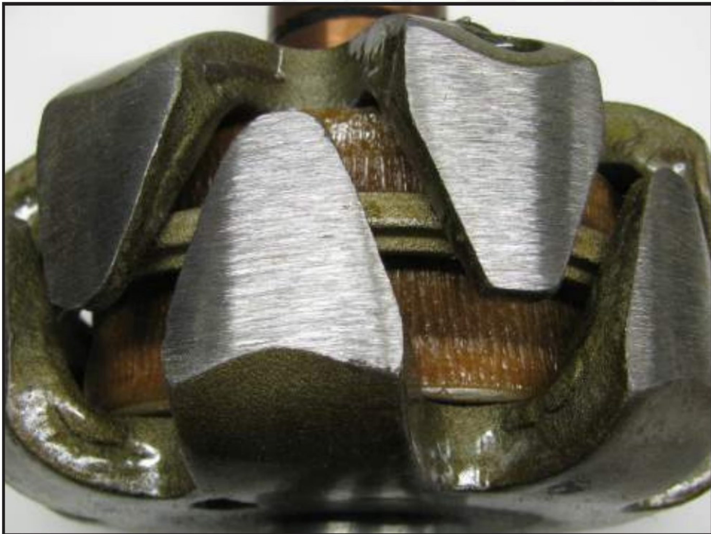
Figure 3 – Rotor poles are machined from soft iron, which is a carbon free alloy with a high iron content. It will retain magnetism.
