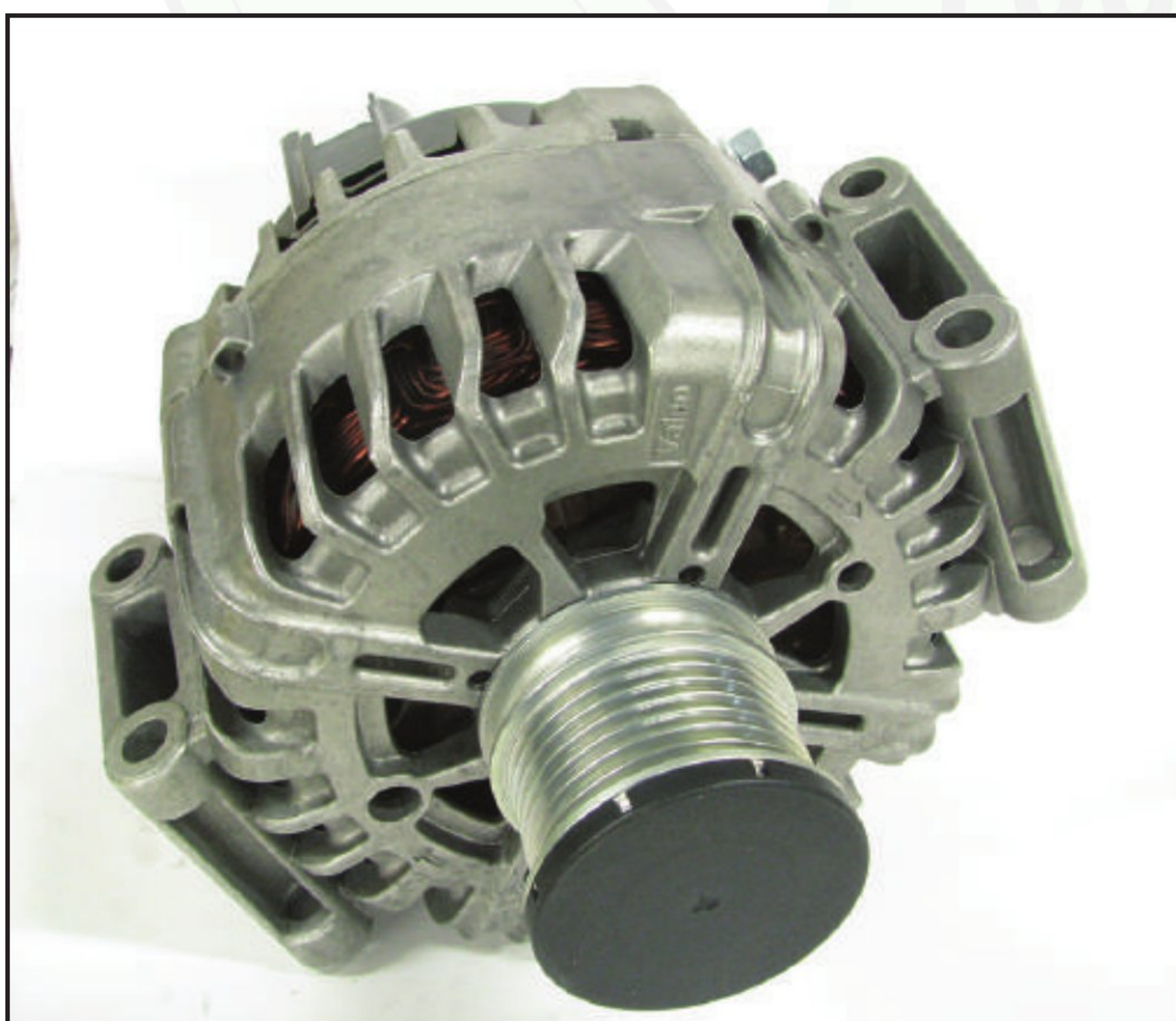
Figure 1 – This Valeo alternator (TG23C019) for Sprinter vans can provide up to 220 amps of power. It uses a 7-groove clutch pulley.
