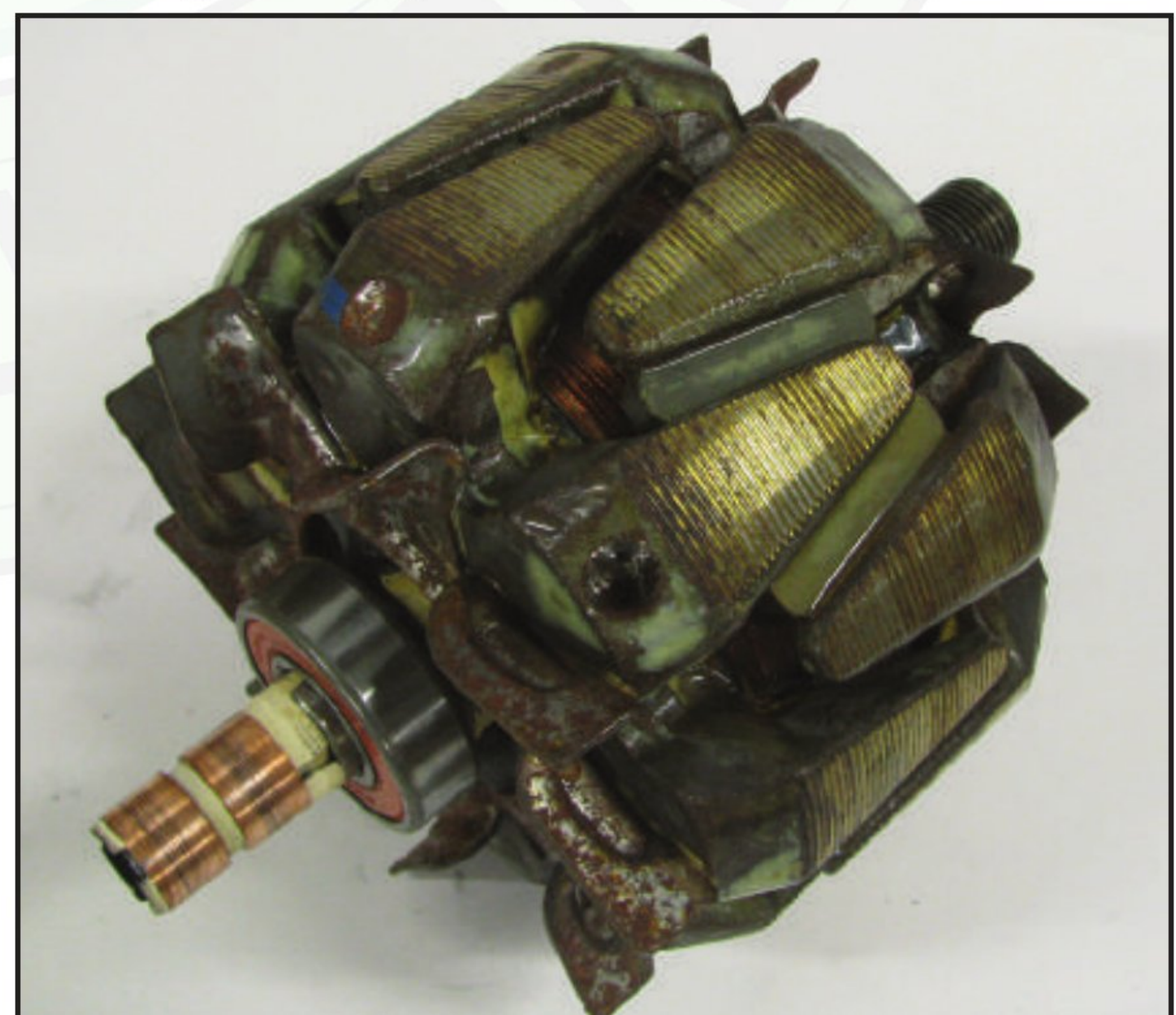
Figure 4 – This Valeo rotor has eight permanent magnets that are epoxied in four evenly spaced locations around the rotor.
