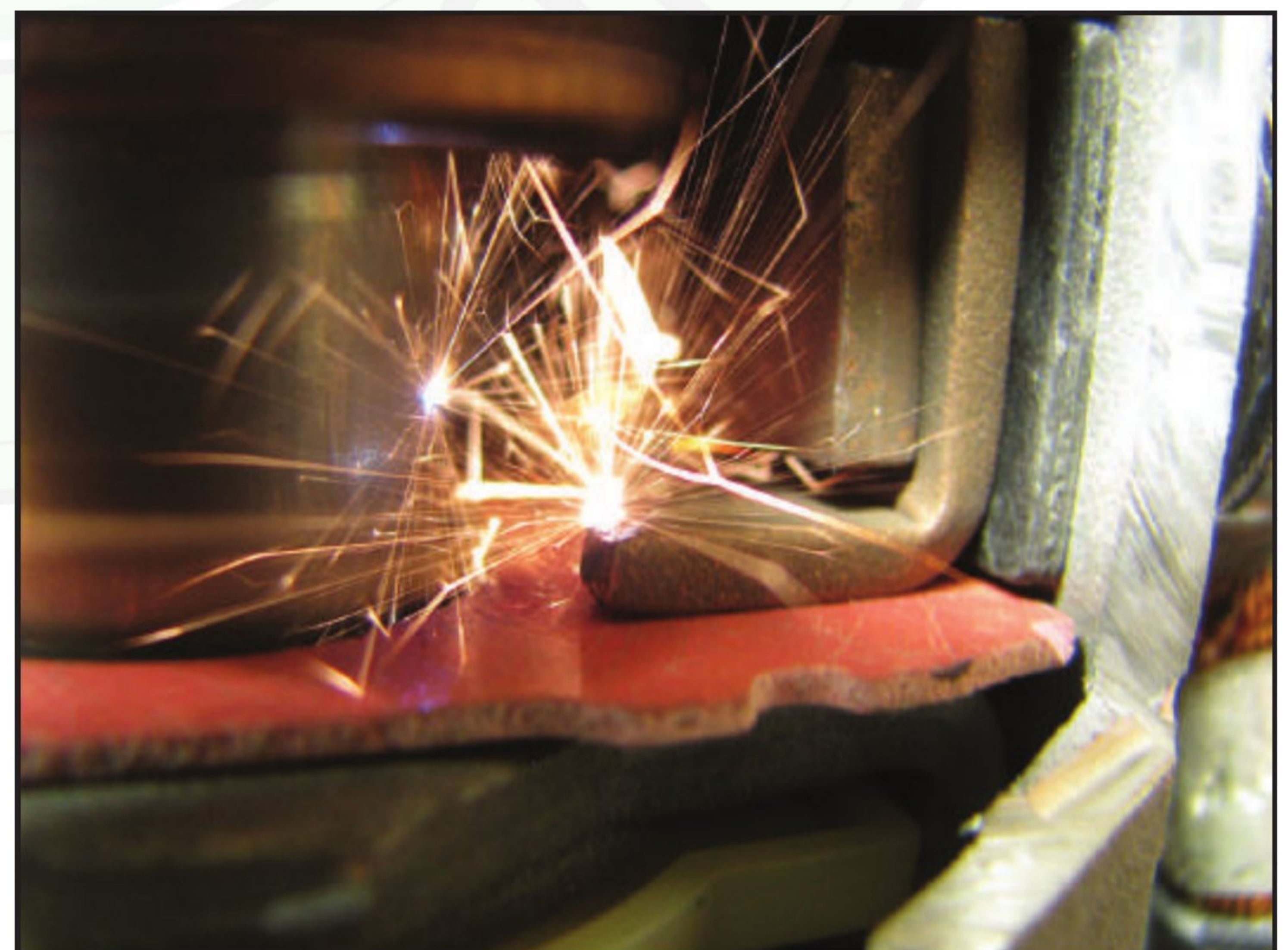
Figure 6 – This is an actual breaking arc on the battery side contacts of the same Denso starter during a free spin test.
