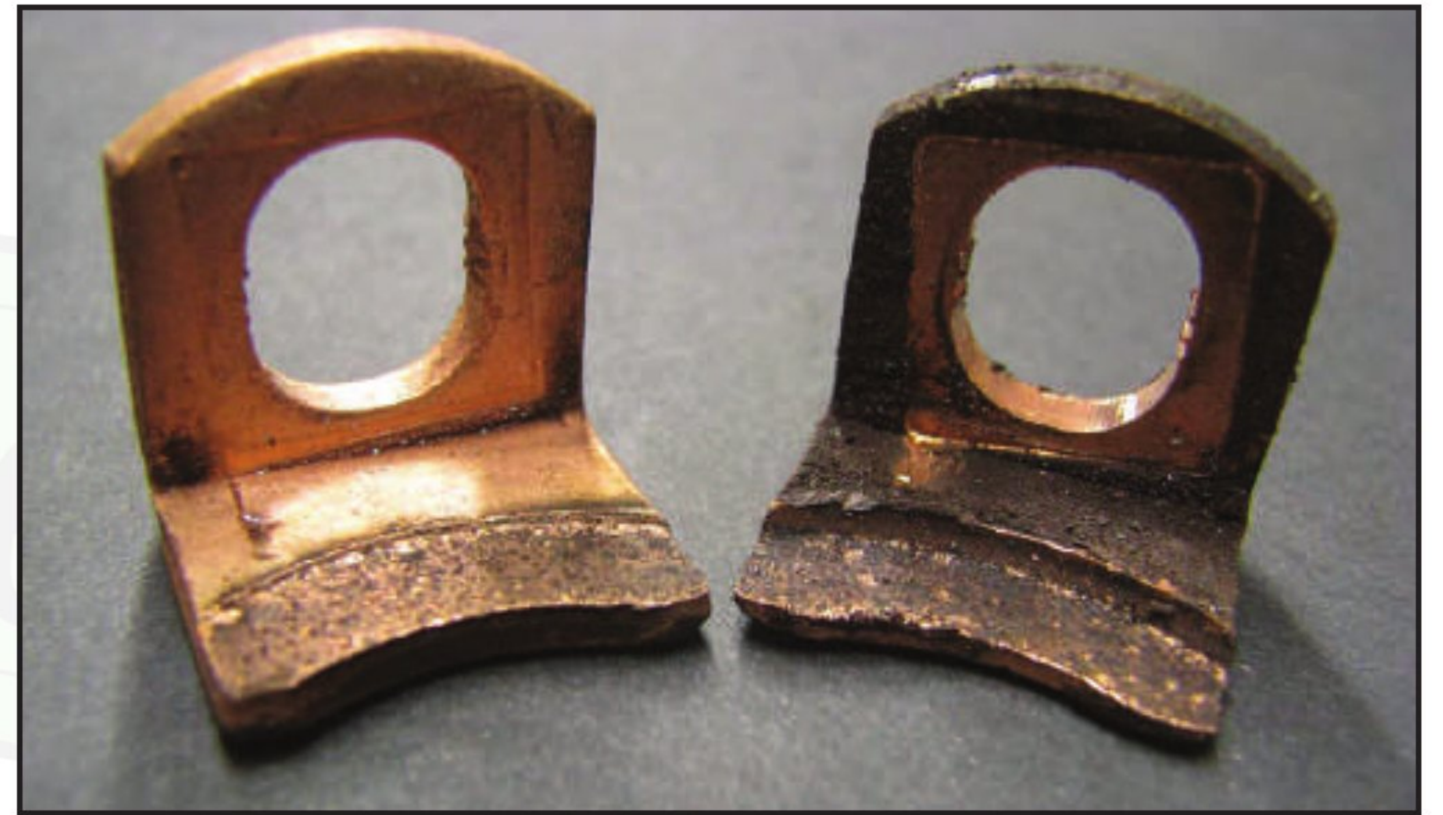
Figure 1 – Used Denso 2.5 kW solenoid contacts, motor terminal (negative) on the left and battery (positive) on the right.
