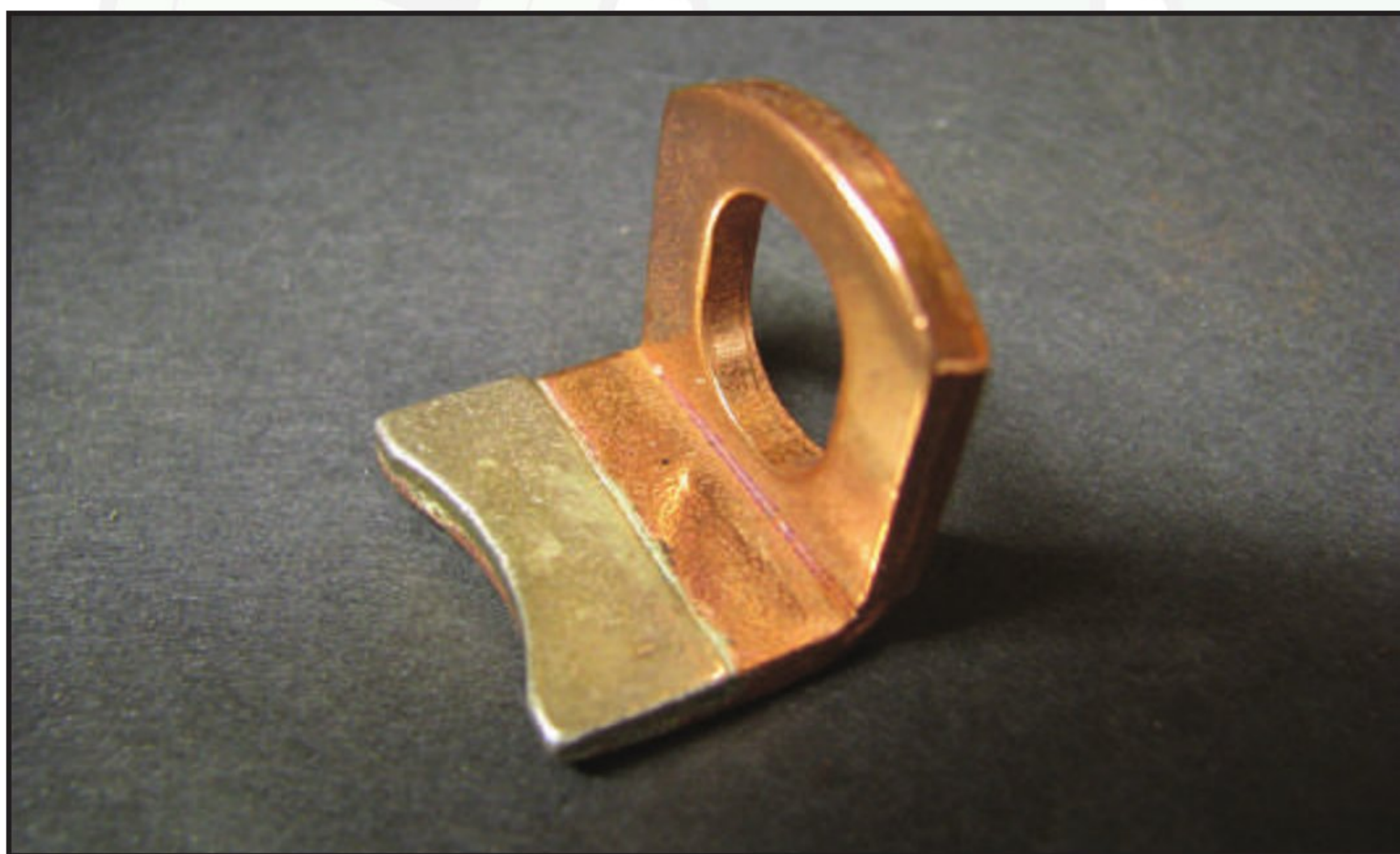
Figure 9 – This 24 volt Denso contact has a silver inlay to reduce arcing under the higher voltage.
