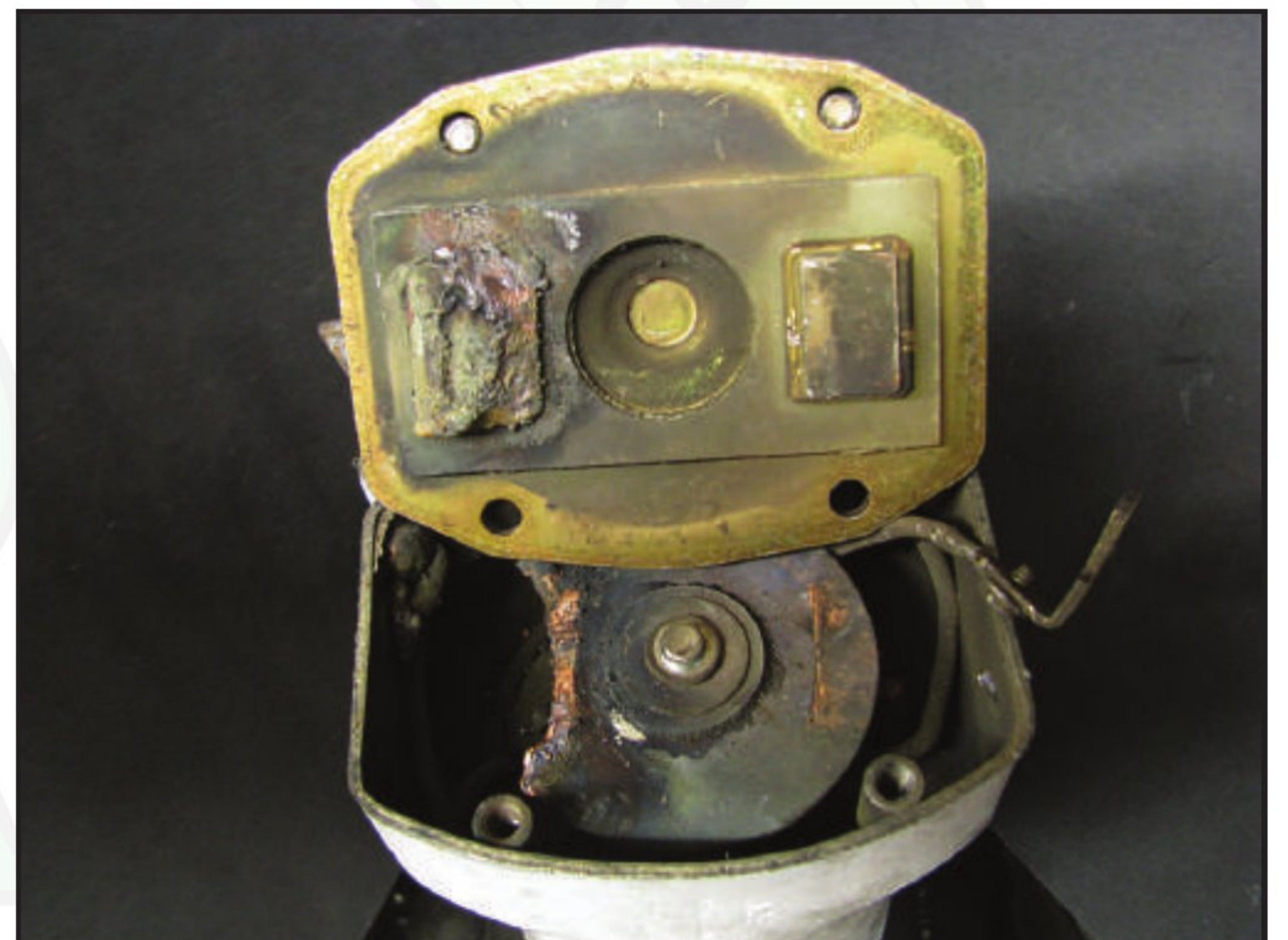
Figure 2 – This 32 volt 40MT starter solenoid was destroyed by severe arcing. Notice that nearly all damage is on the battery contact (left) – positive side.
