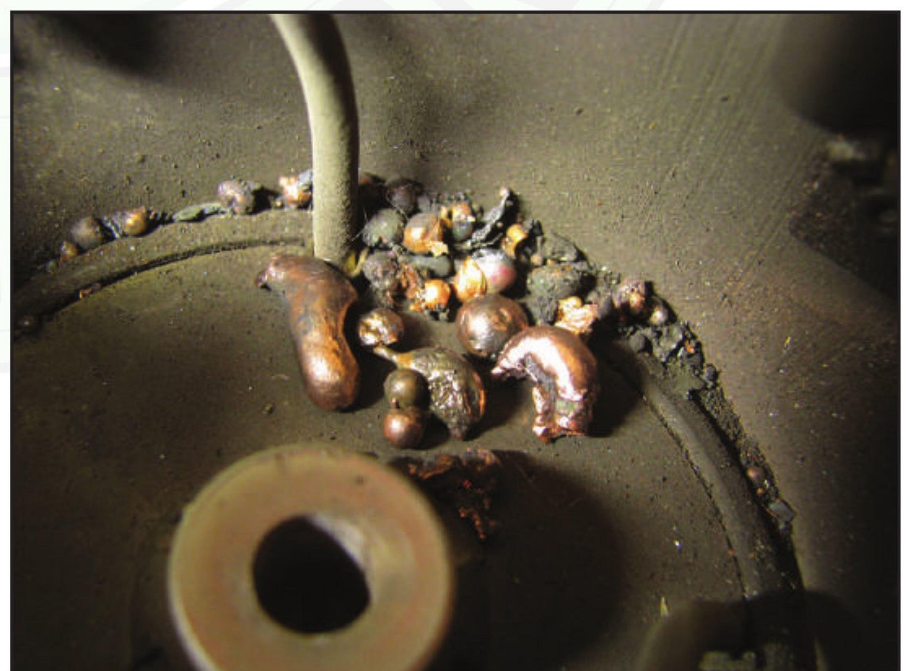
Figure 16 – This copper residue was once part of the moving contact where it last touched the battery contact.
