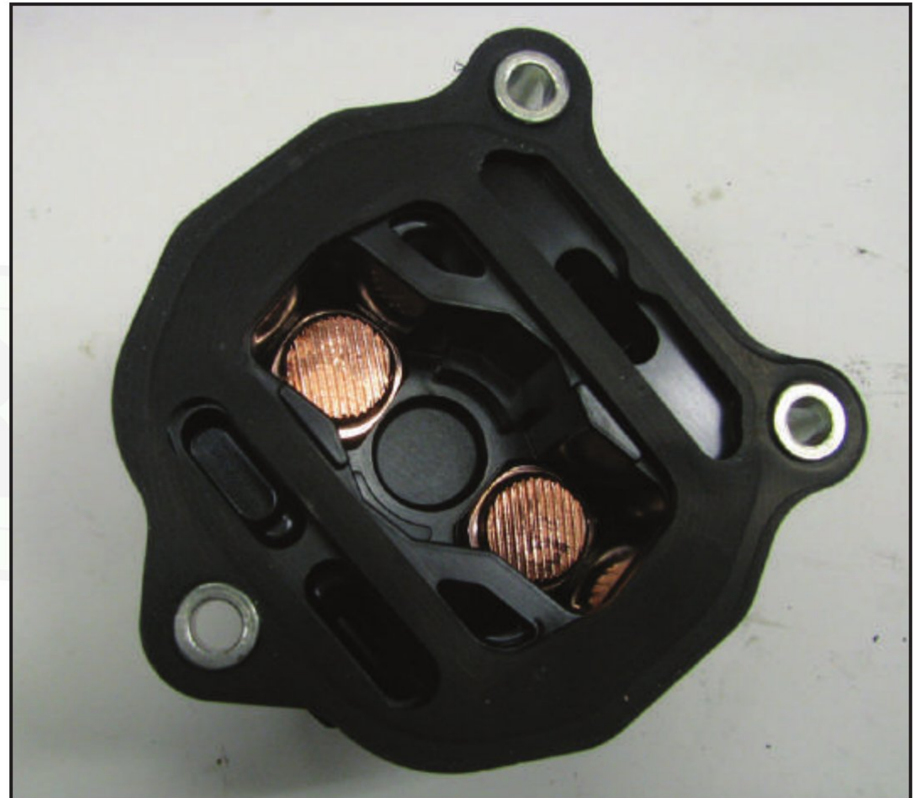
Figure 11 – This Denso PA90S solenoid utilizes straight ridges to limit arcing.
