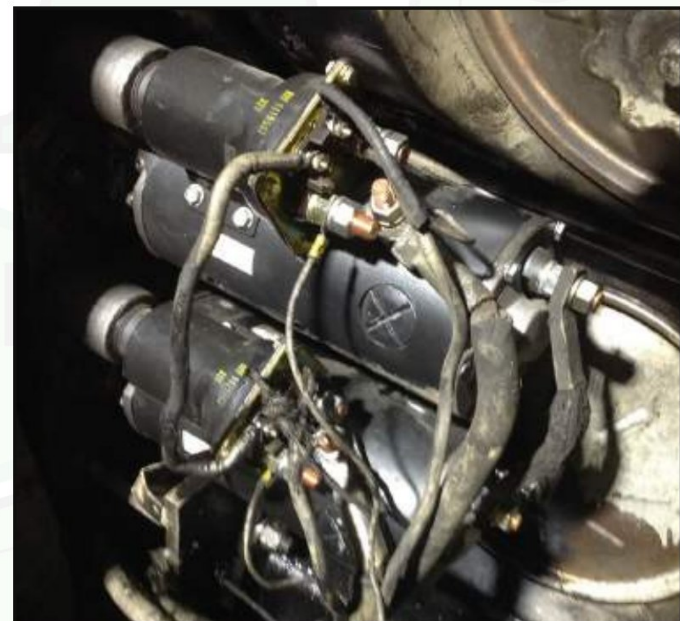
Figure 1 – A team of 32v 50MT starters, mounted on a Detroit Diesel engine in a locomotive.
