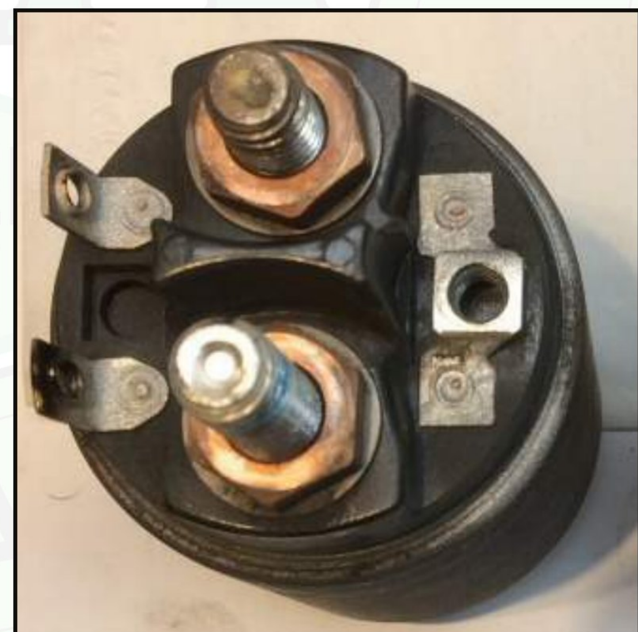
Figure 9 – The spade terminals on the left are grounds for the two coils inside.
