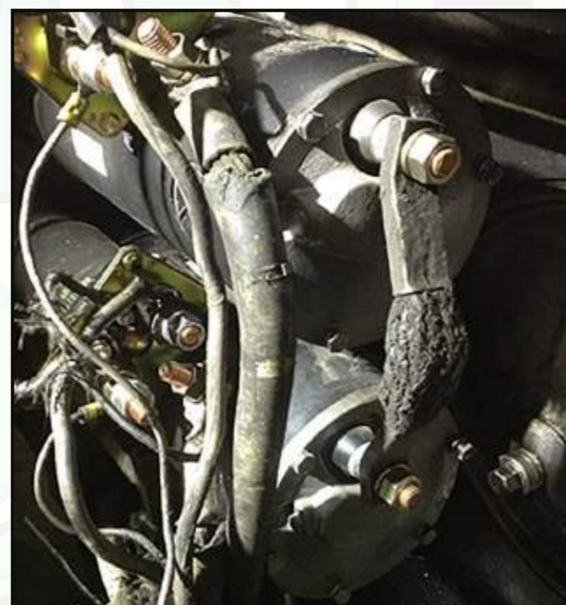
Figure 5 – Note the heavy strap that connects the two starter "ground" terminals in opposing polarity.
