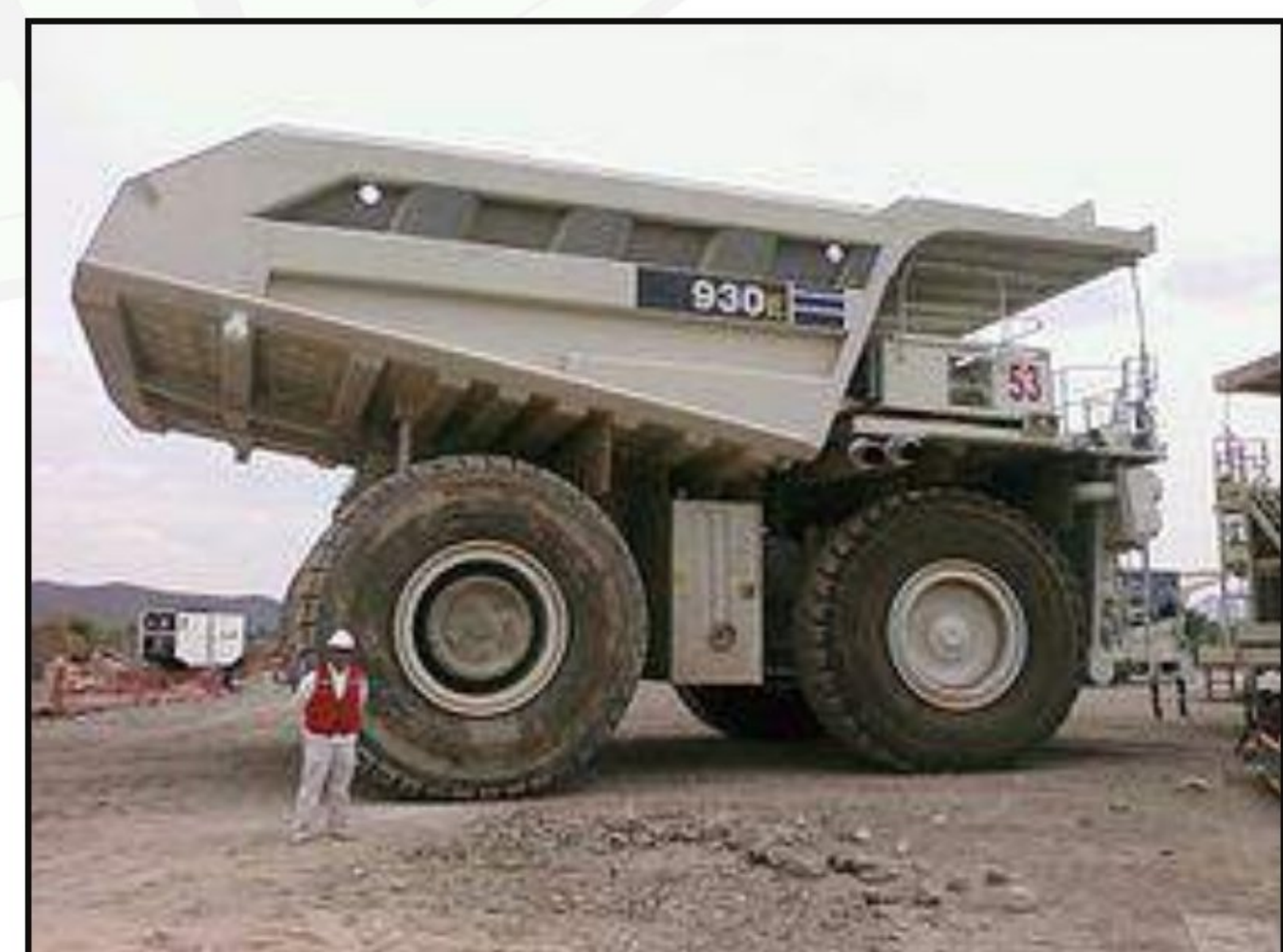
Figure 6 – Komatsu 930E haul truck powered by a 4000 HP MTU diesel engine.
