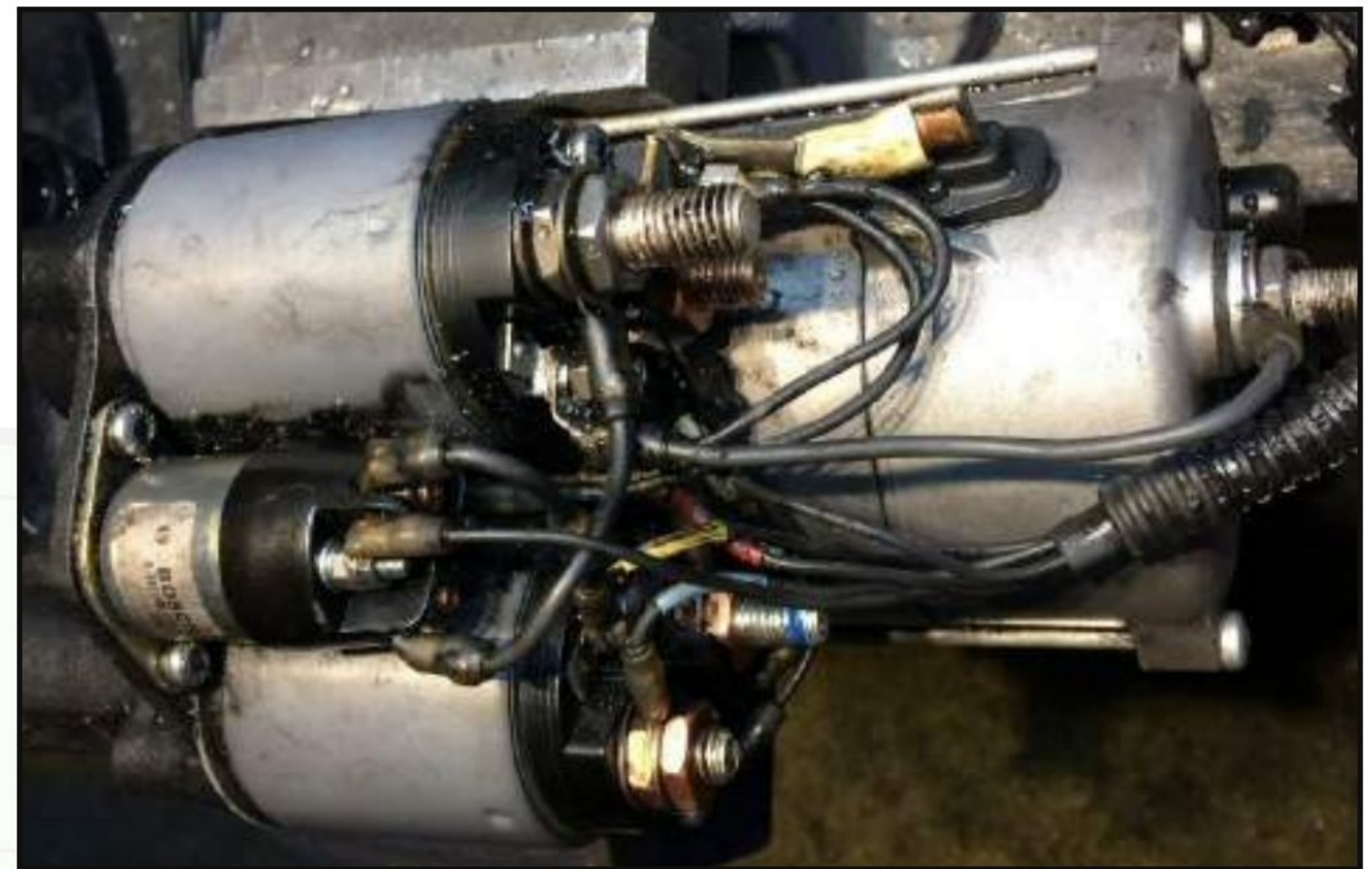
Figure 7 – Bosch 0-001-340-501, one of a pair used to crank the mammoth MTU diesel.
