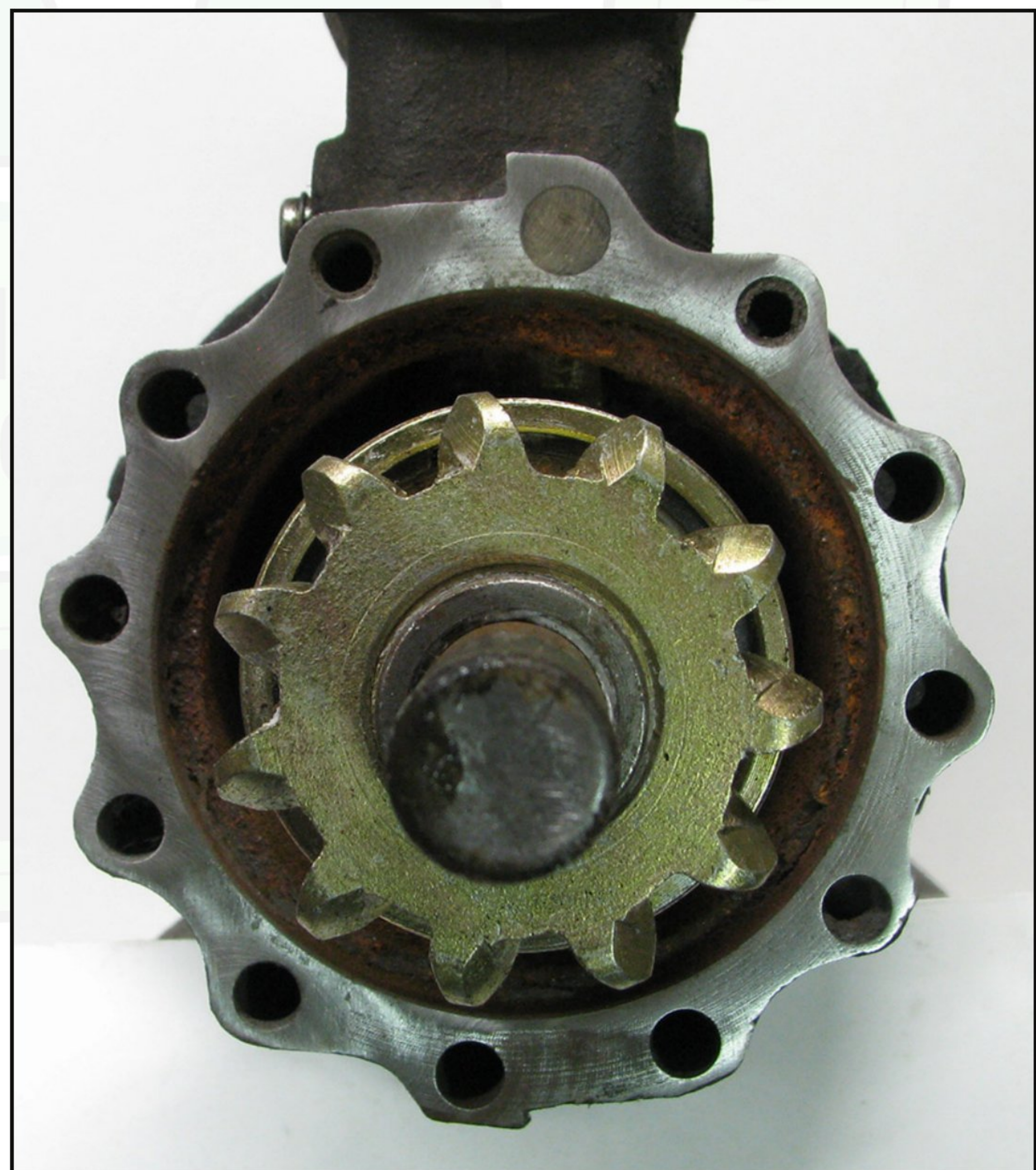
Figure 6 – “P” lever housing with mounting holes shifted to the right
