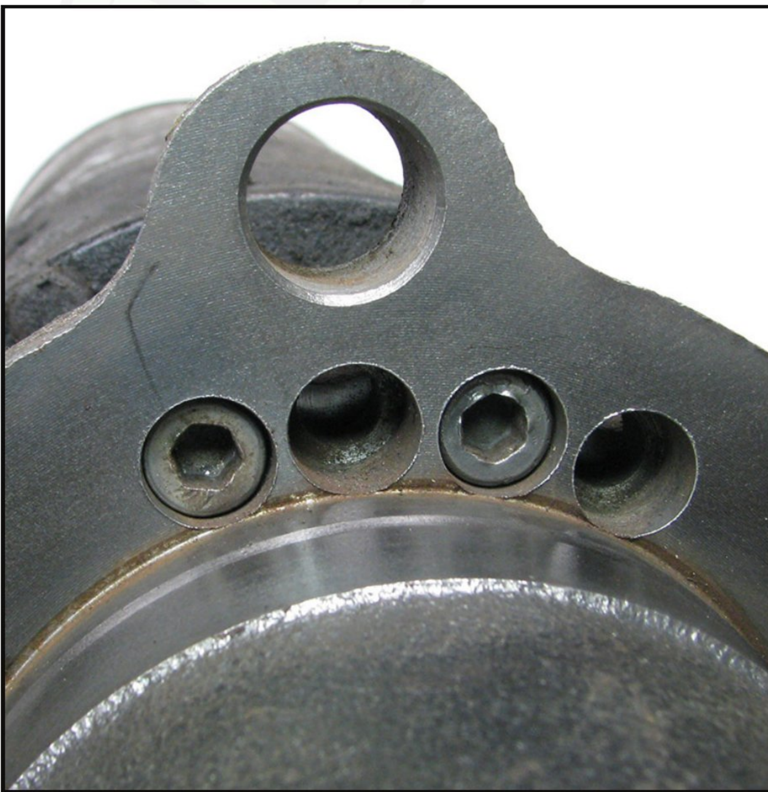
Figure 4 – 4-hole DE housing allows for 24 possible positions
