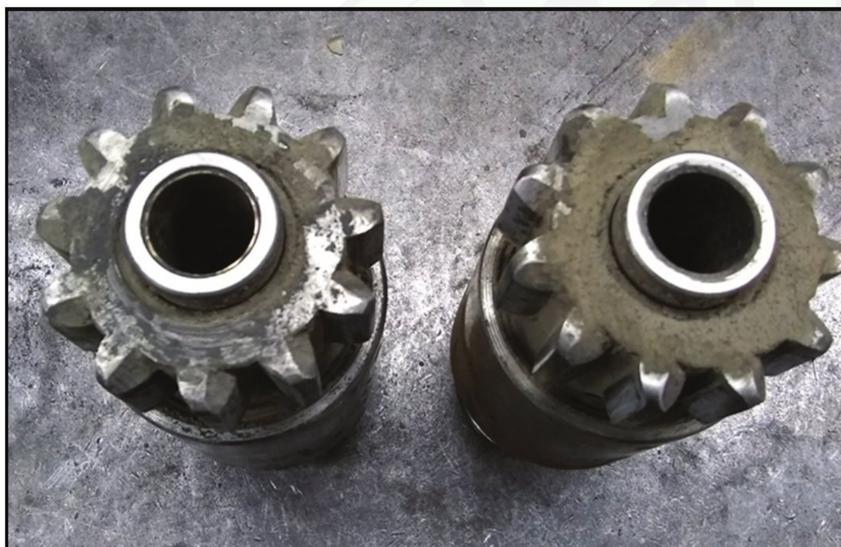
Figure 3 – As you can see from the original pinion gears, there is no sign of milling.
