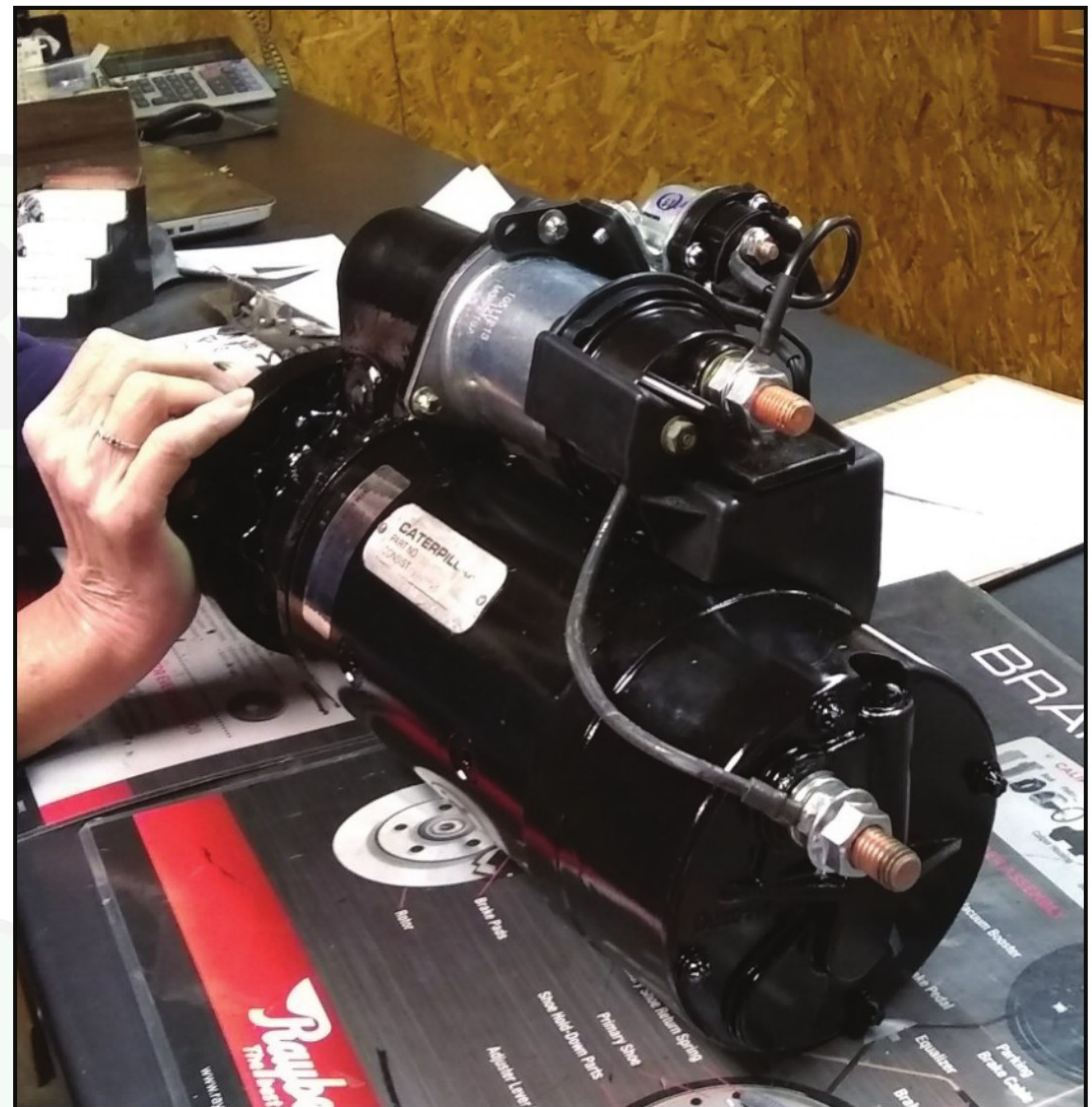
Figure 1 – This is pretty much a standard 42MT starter, except for the plastic cover for the terminals.
