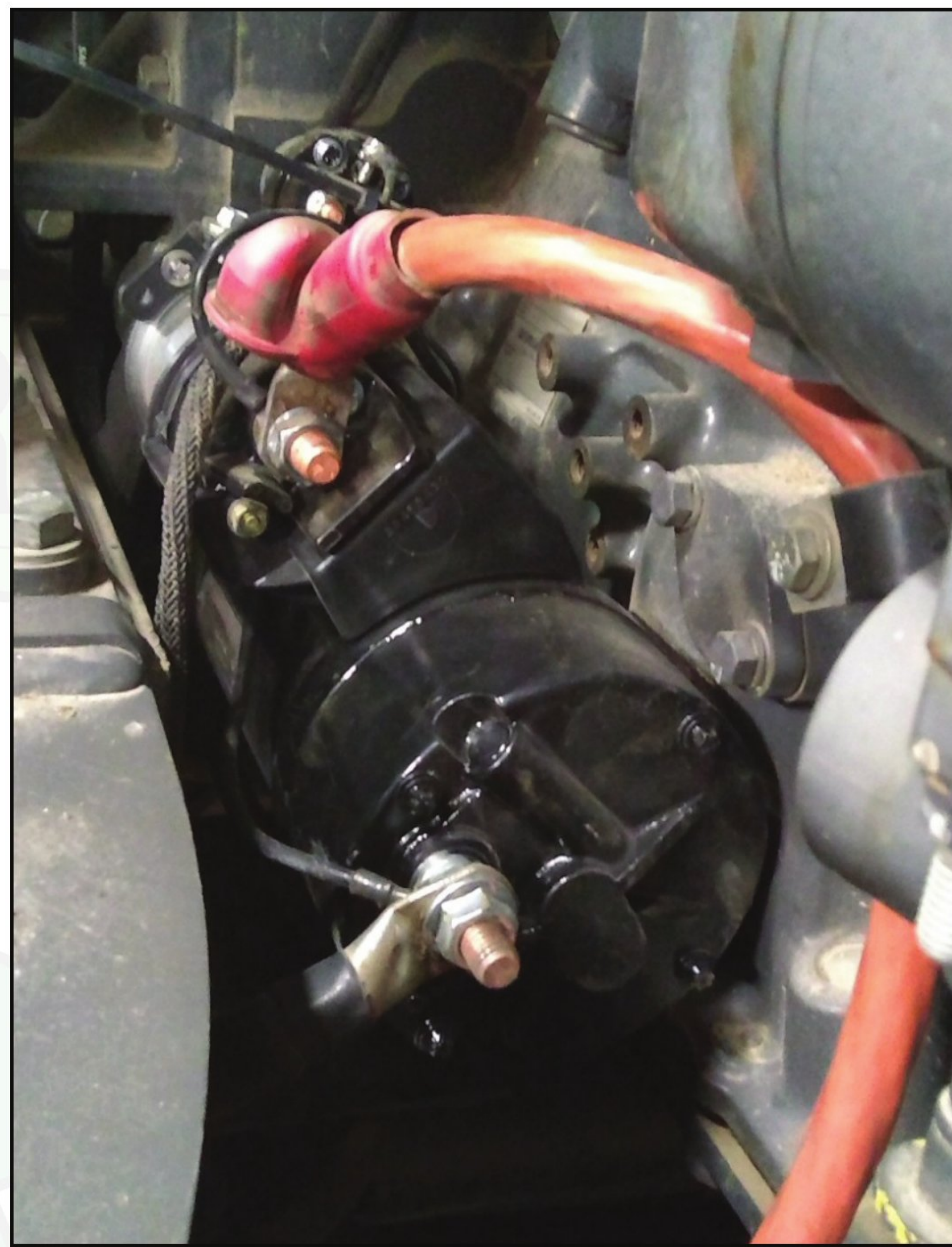
Figure 4 – Here you can see the right side starter mounted on the engine.
