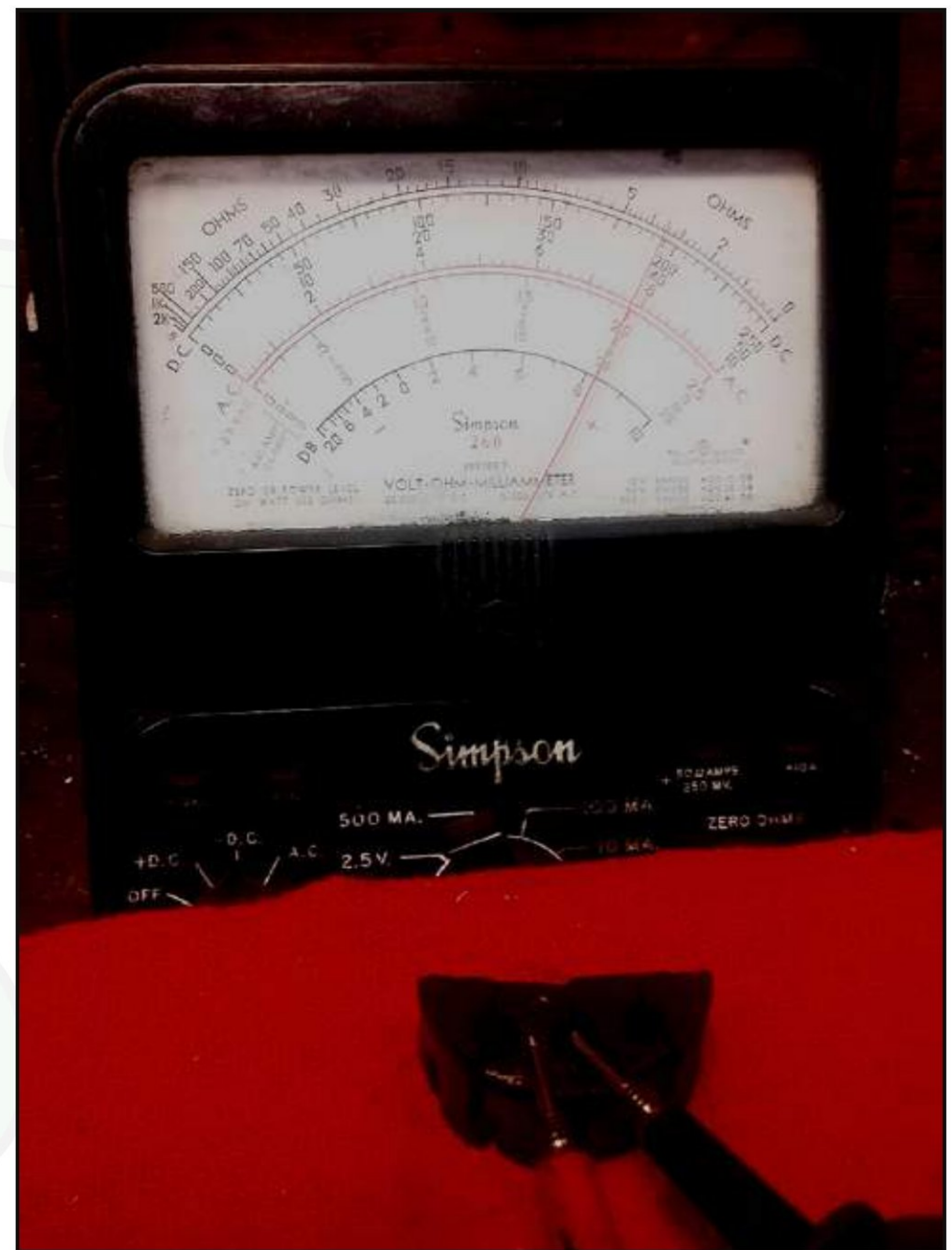
Figure 2 – 30SI insulator being tested for conductivity.
