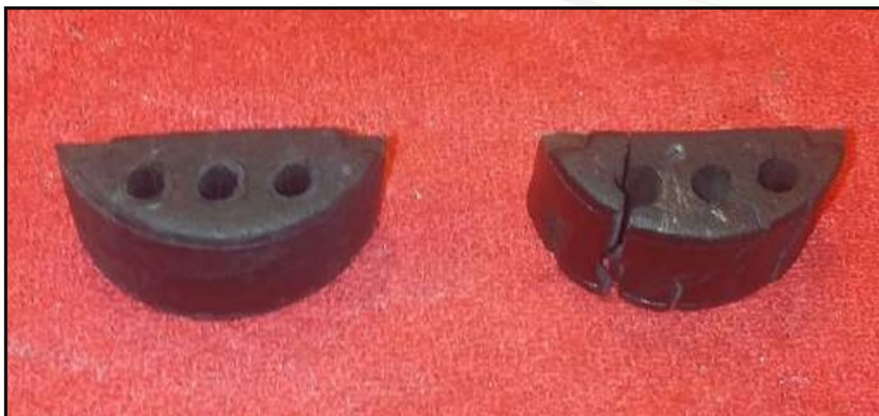
Figure 1 – 30SI stator lead insulators
