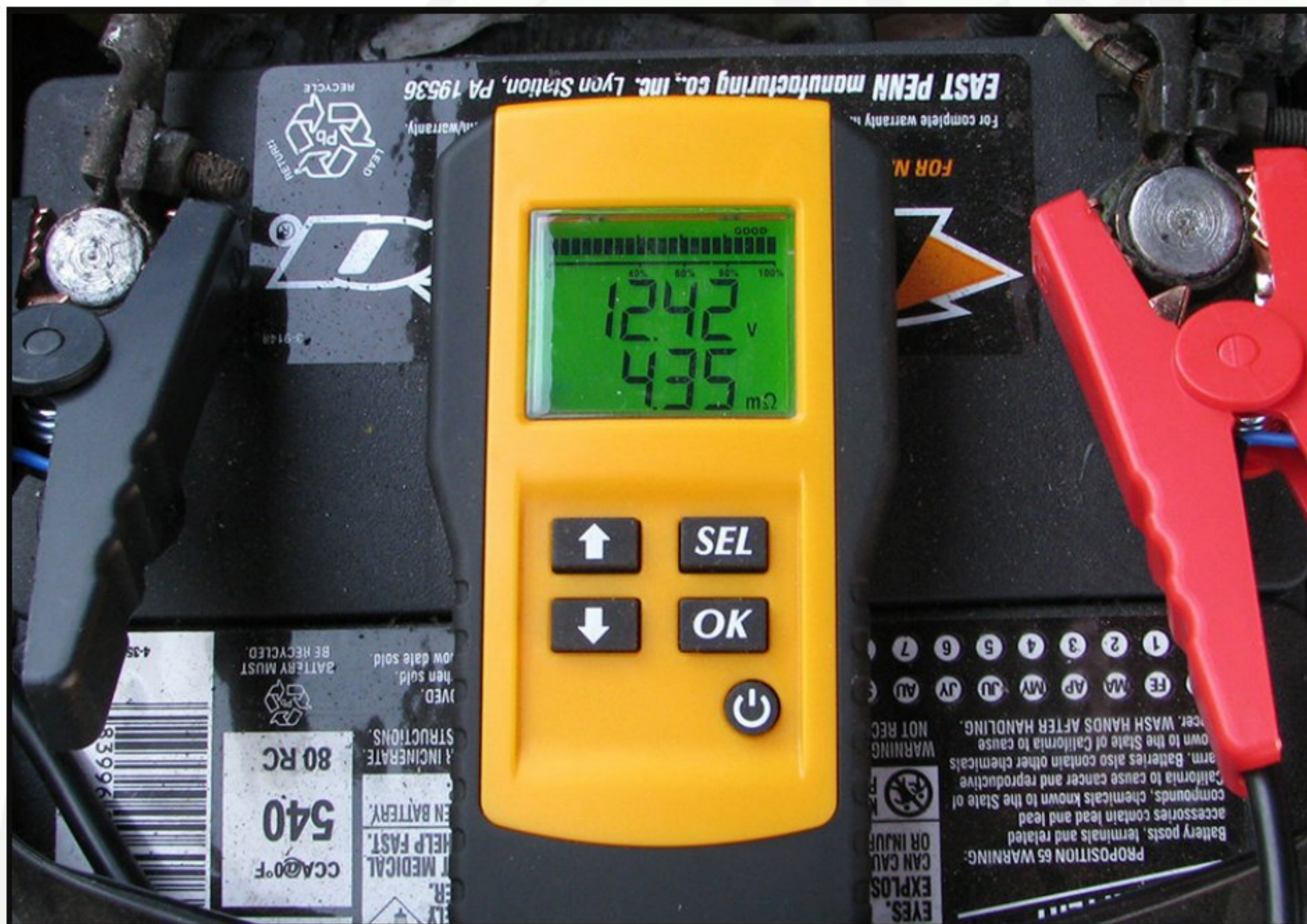
Figure 6 – Suner Power tester's illuminated LCD display screen
