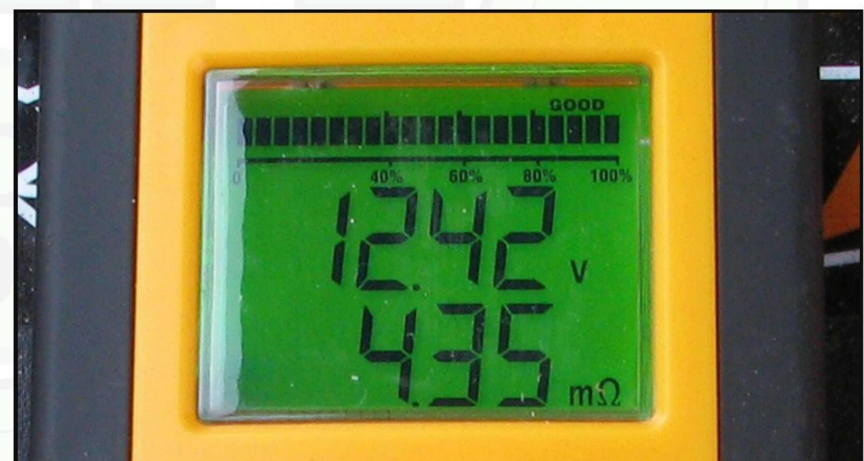
Figure 9 – Suner Power tester display for the Deka battery
