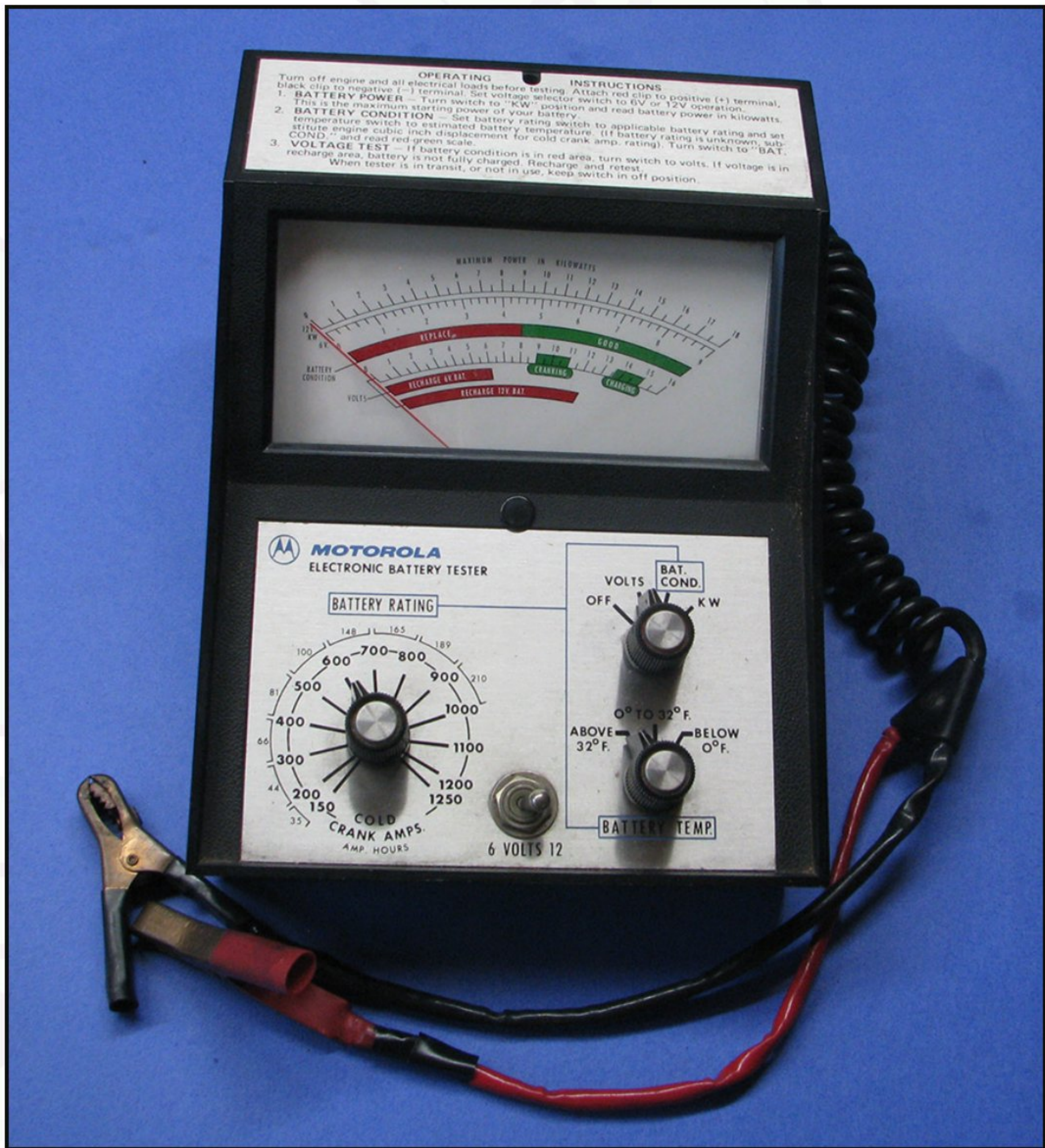
Figure 2 – Motorola Electronic Battery Tester with analog meters from the 1980's.
