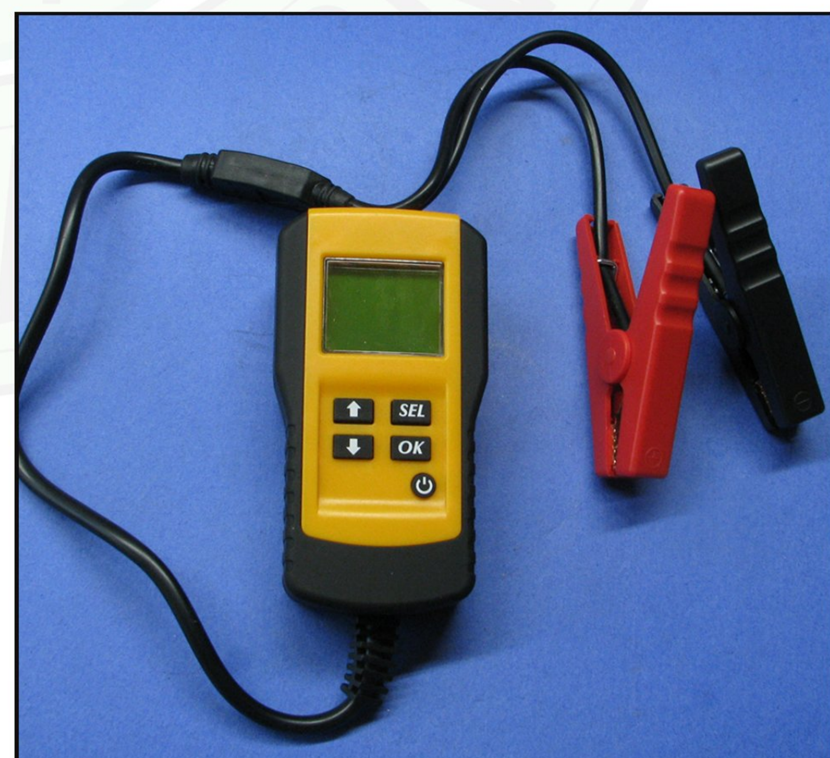
Figure 5 – Suner Power battery tester
