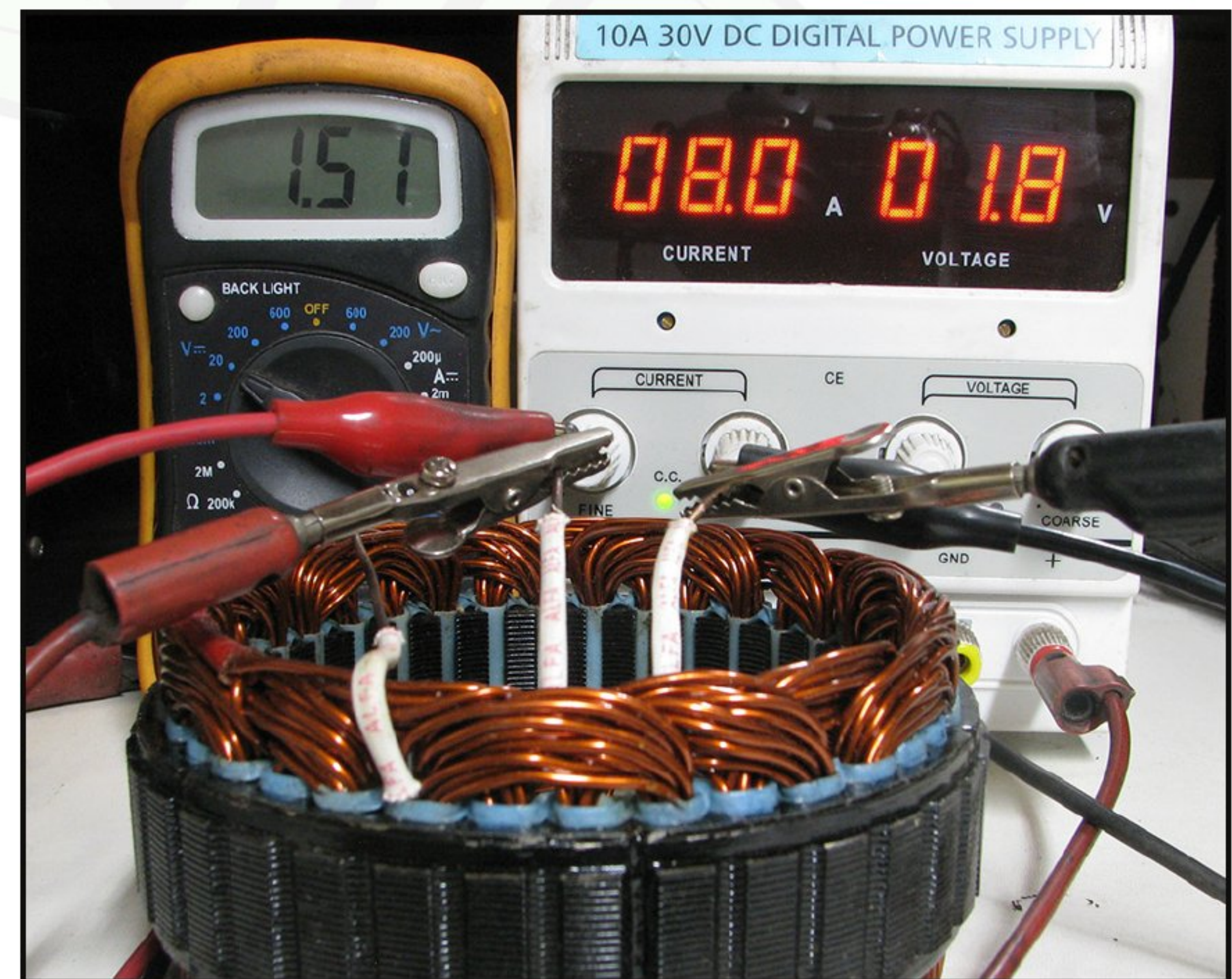
Figure 8 – Using a constant current DC power supply to check for balance between coils.
