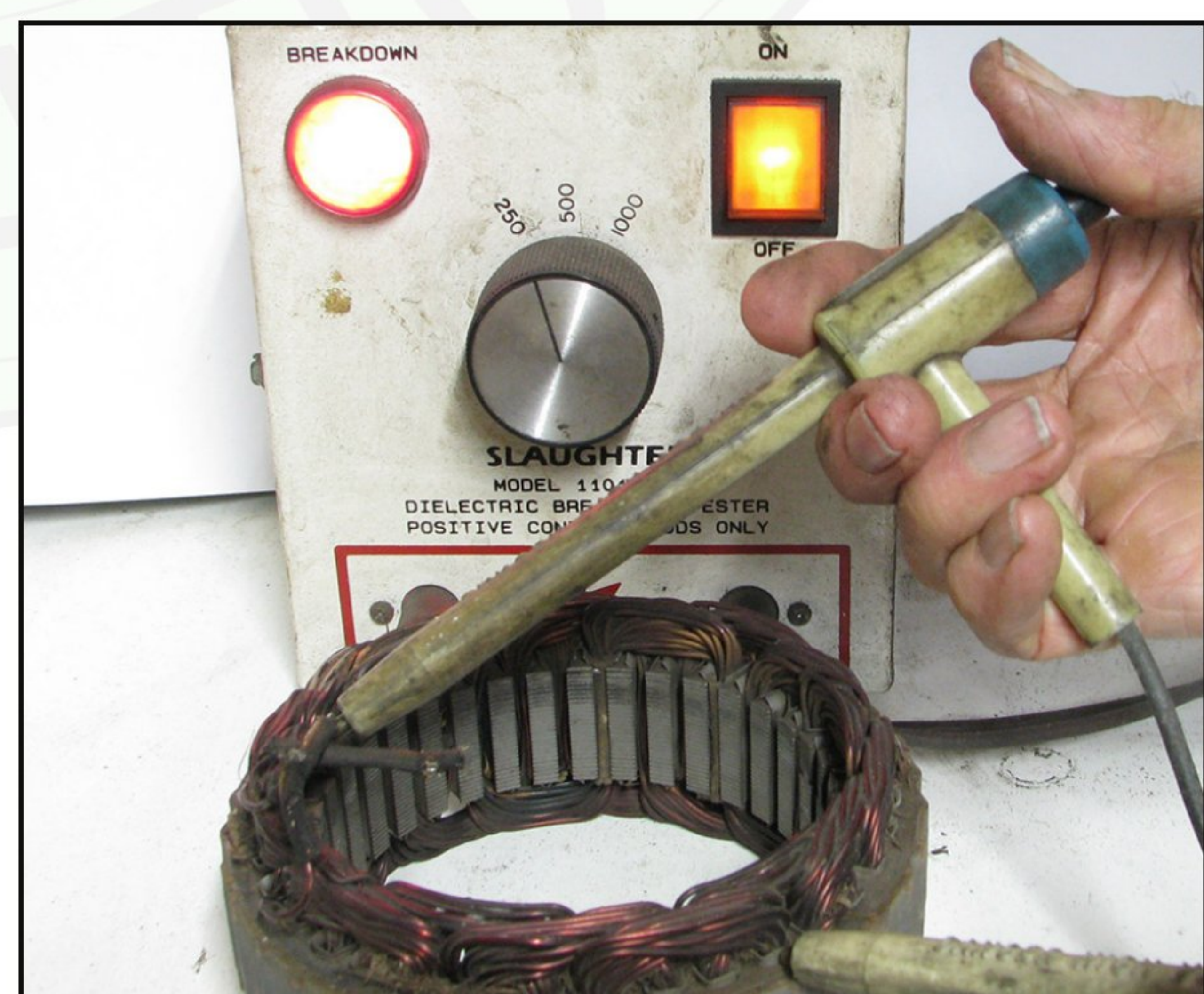
Figure 6 – Testing for a short to ground at 250 volts.
