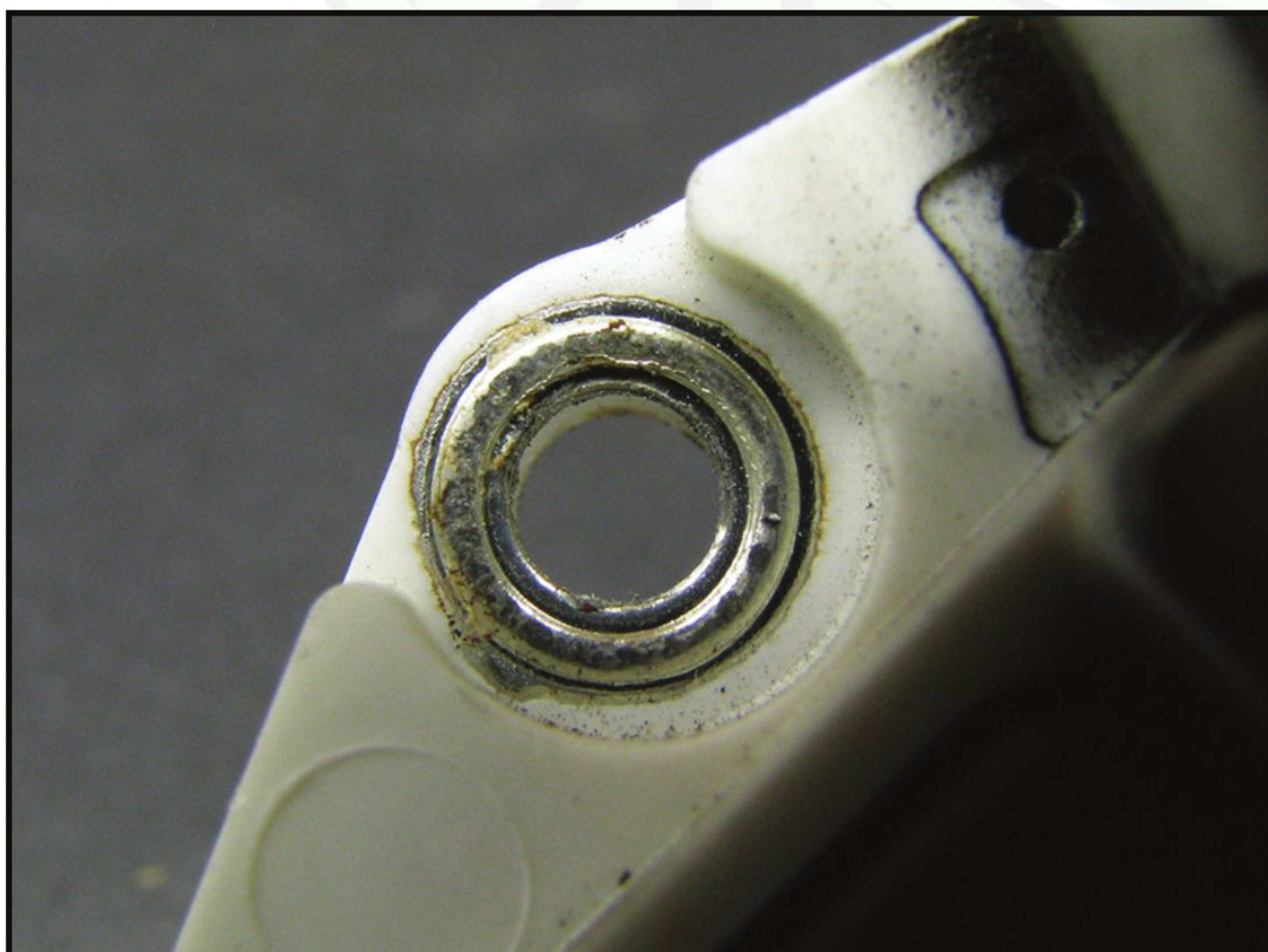
Figure 4 – Here you can clearly see arcing on the regulator's ground tab, caused by a loose mounting screw.
