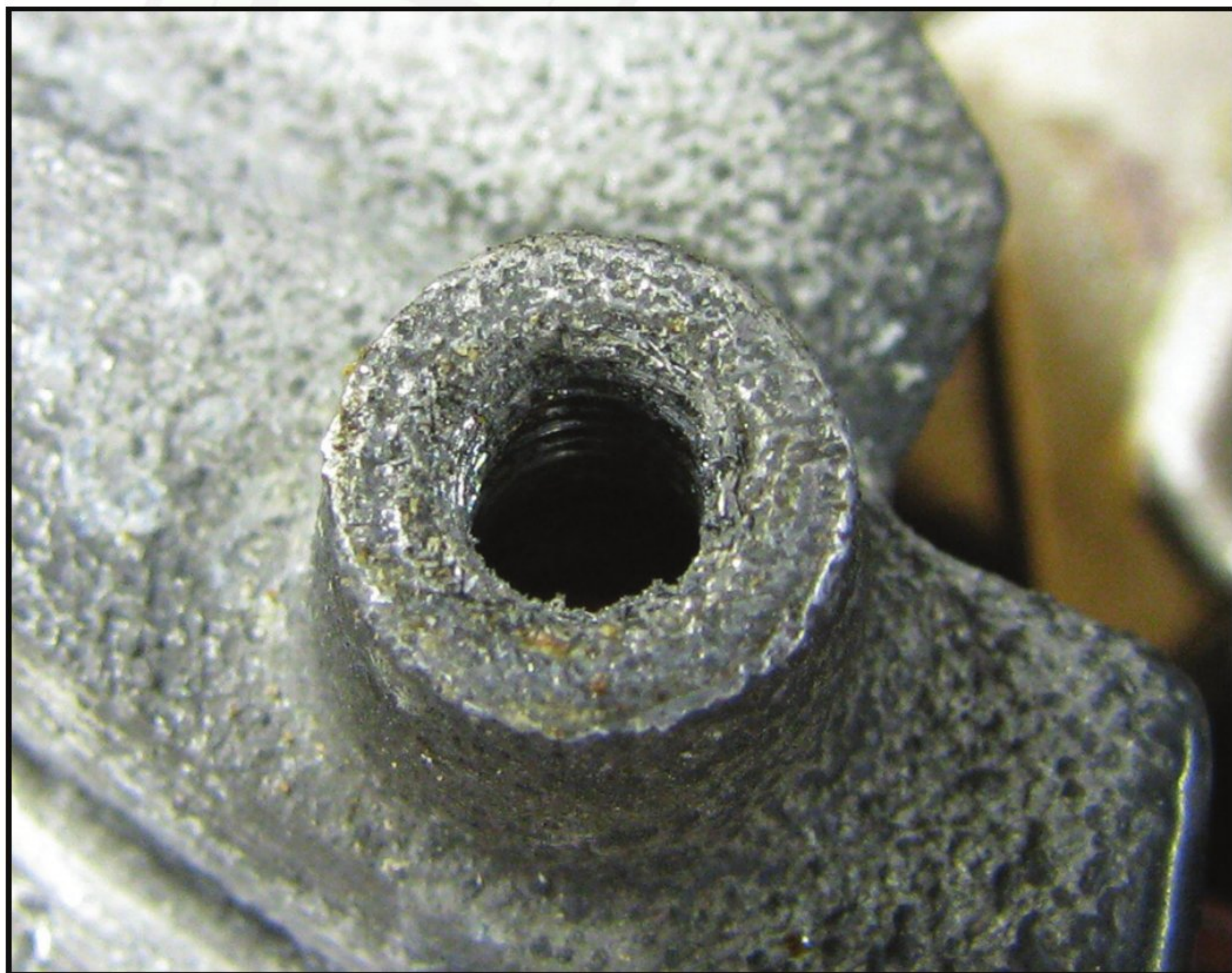
Figure 3 – This is a close up photo of the pitting on the surface of the regulator's ground side mounting post.
