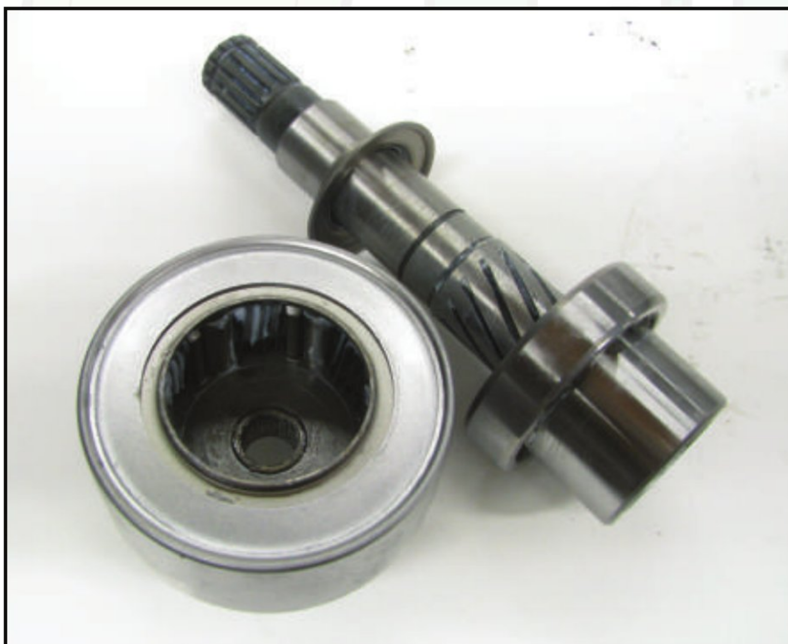
Figure 18 – View of the roller clutch, inner race and shaft.
