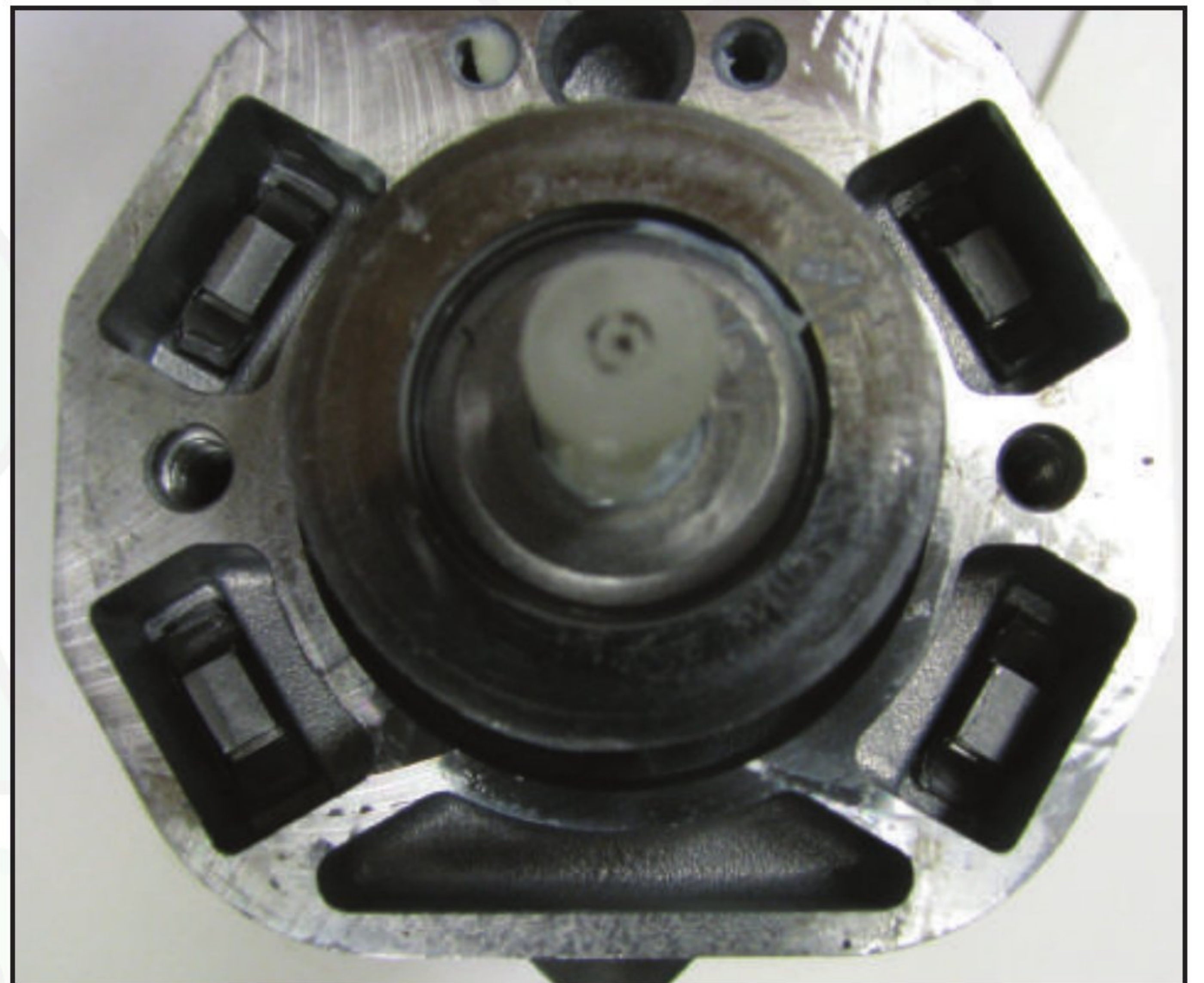
Figure 25 – PA90S solenoid coils are staked in four places for improved reliability.
