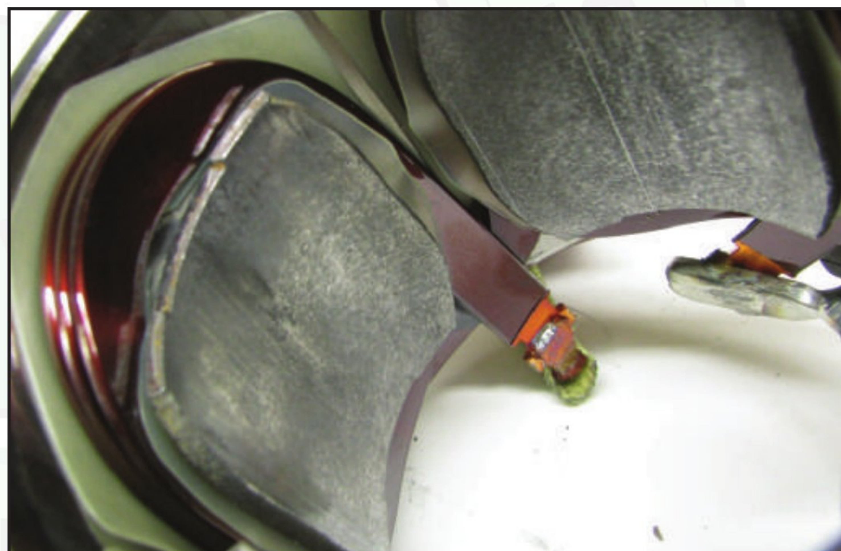
Figure 7 – Note the way that these field coils are wound, the number of turns and the size of the wire.
