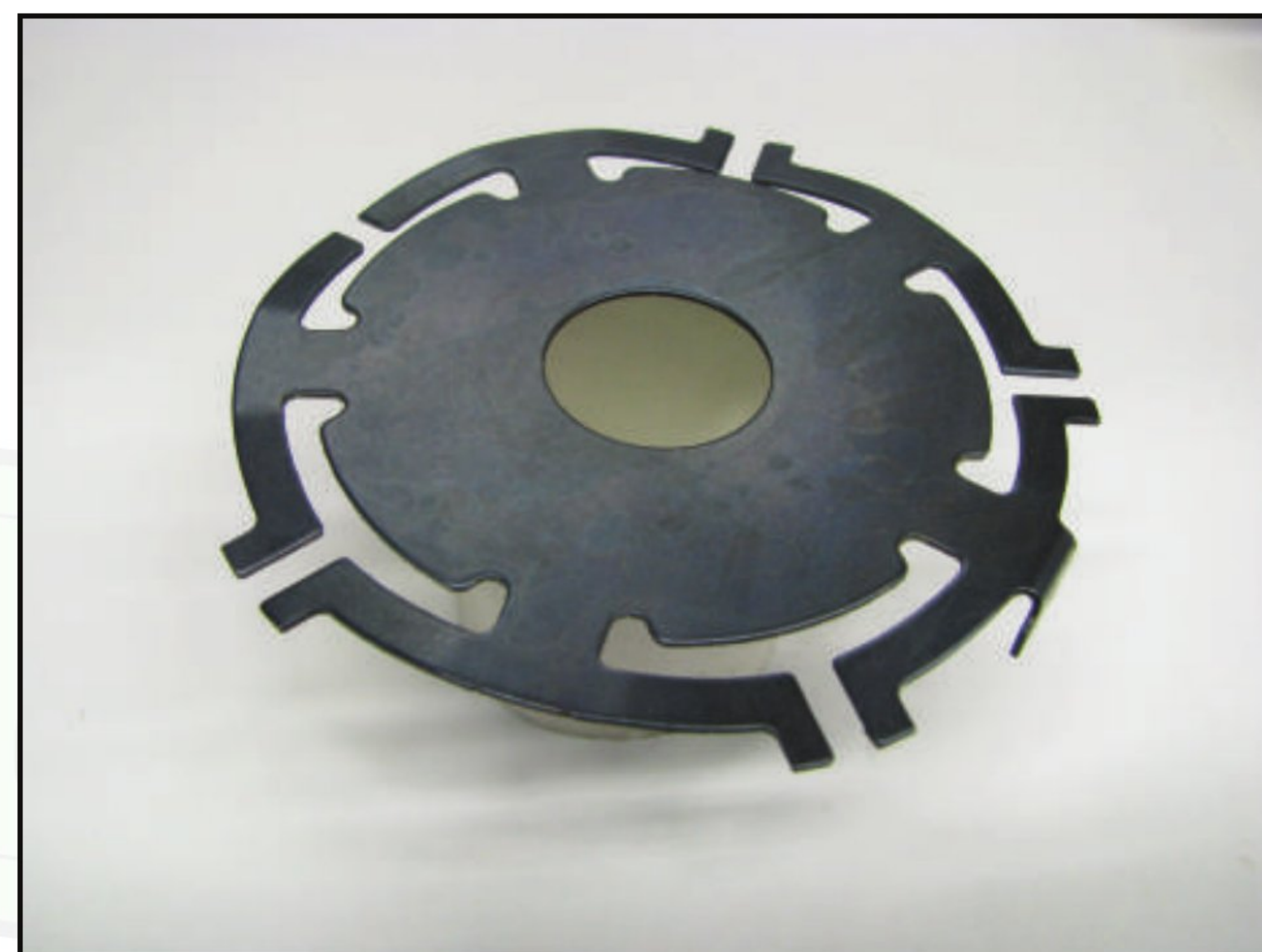
Figure 12 – This odd shaped spring plate is a key part of the PA90S slip disk shock absorber.
