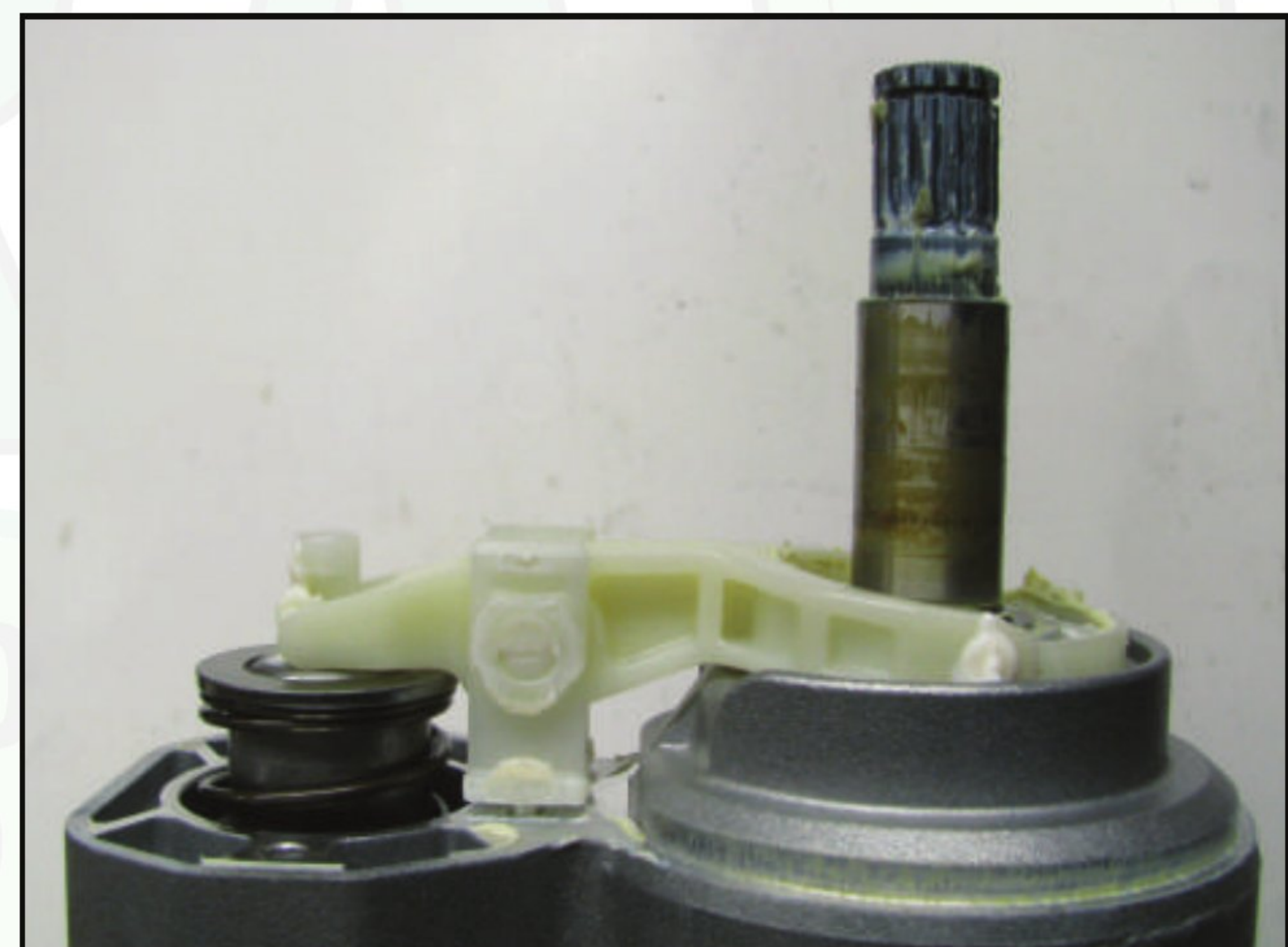
Figure 16 – View of plunger, shift lever and pinion shaft once the DE housing has been removed.
