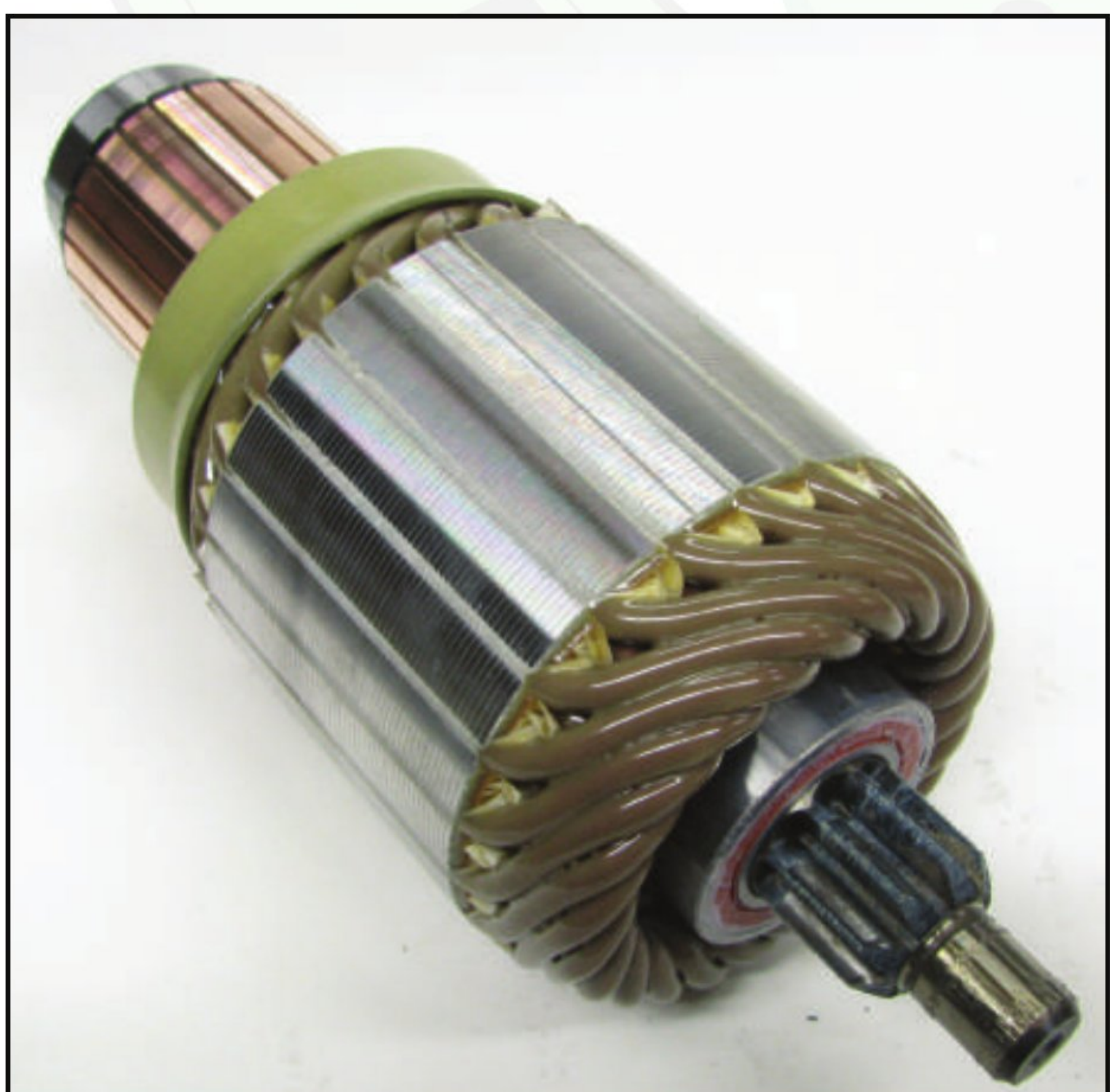
Figure 5 – The PA90S armature's DE bearing will be a challenge to remove.
