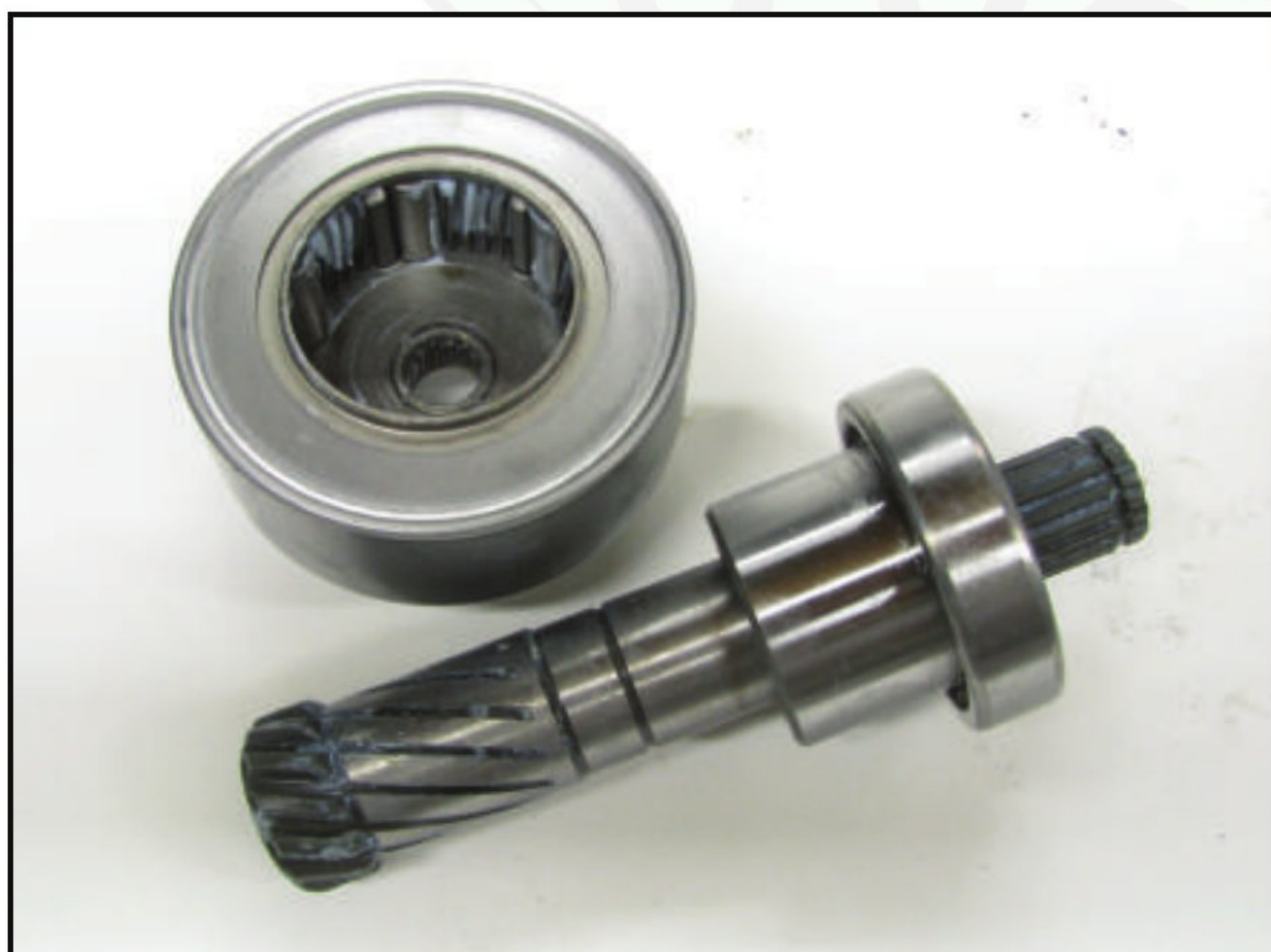
Figure 19 – The clutch's rollers and springs are similar to those on OSGR Denso starters.
