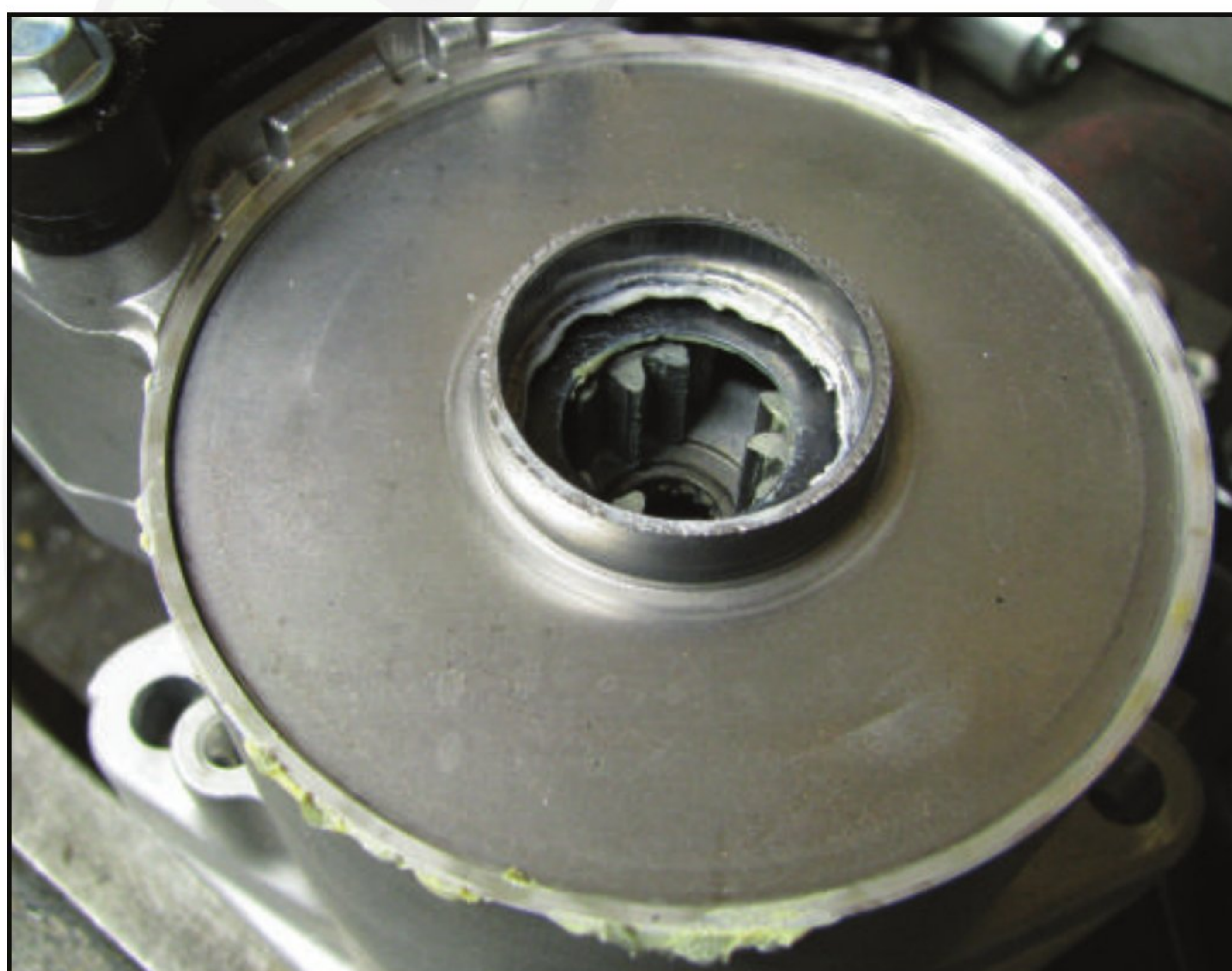
Figure 10 – View of the planetary gear's cover plate once the field case and armature have been removed.
