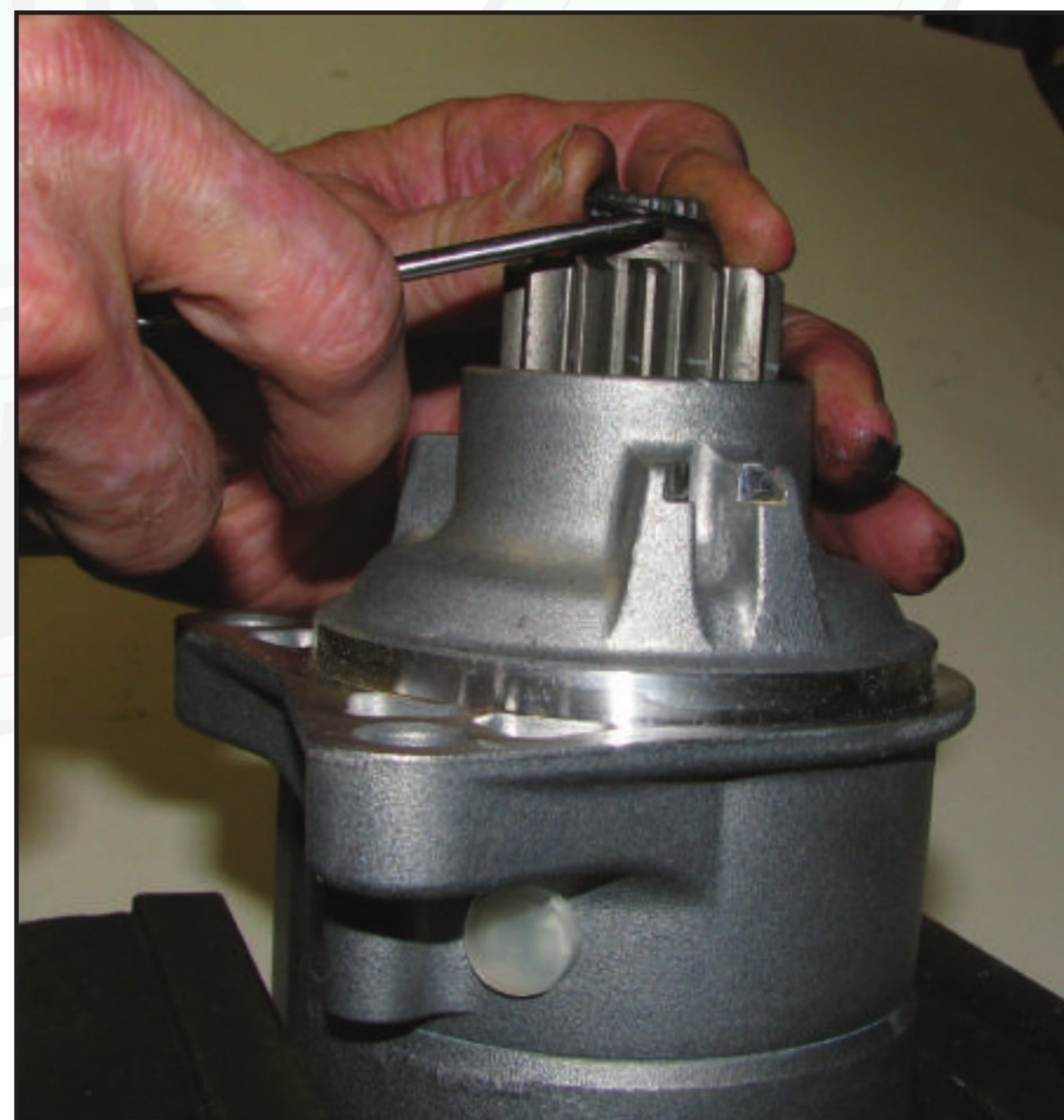
Figure 14 – Snap ring removal is not difficult once the shaft is held extended by a pin punch.
