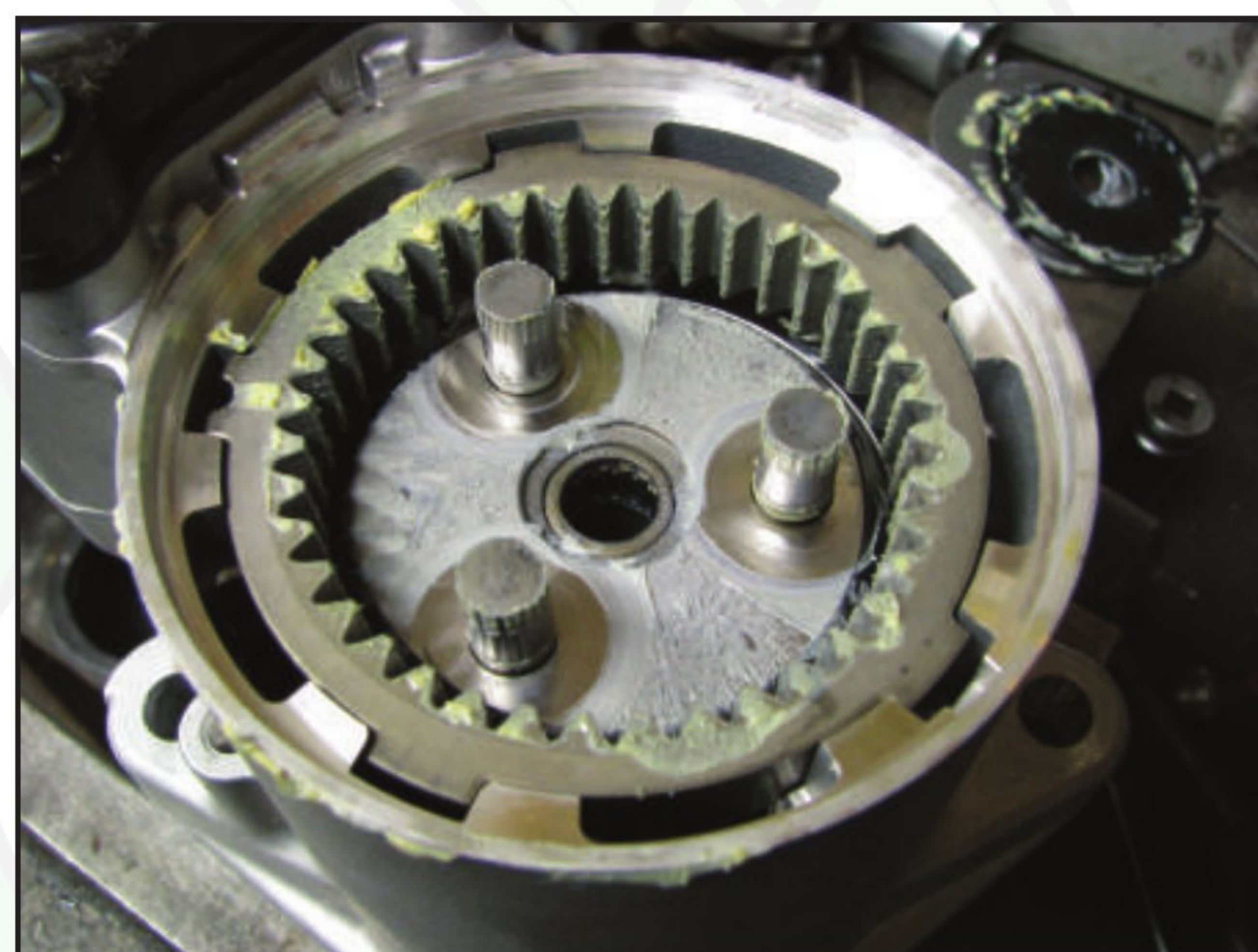
Figure 13 – View of the stationary gear in the housing with drive clutch below it.
