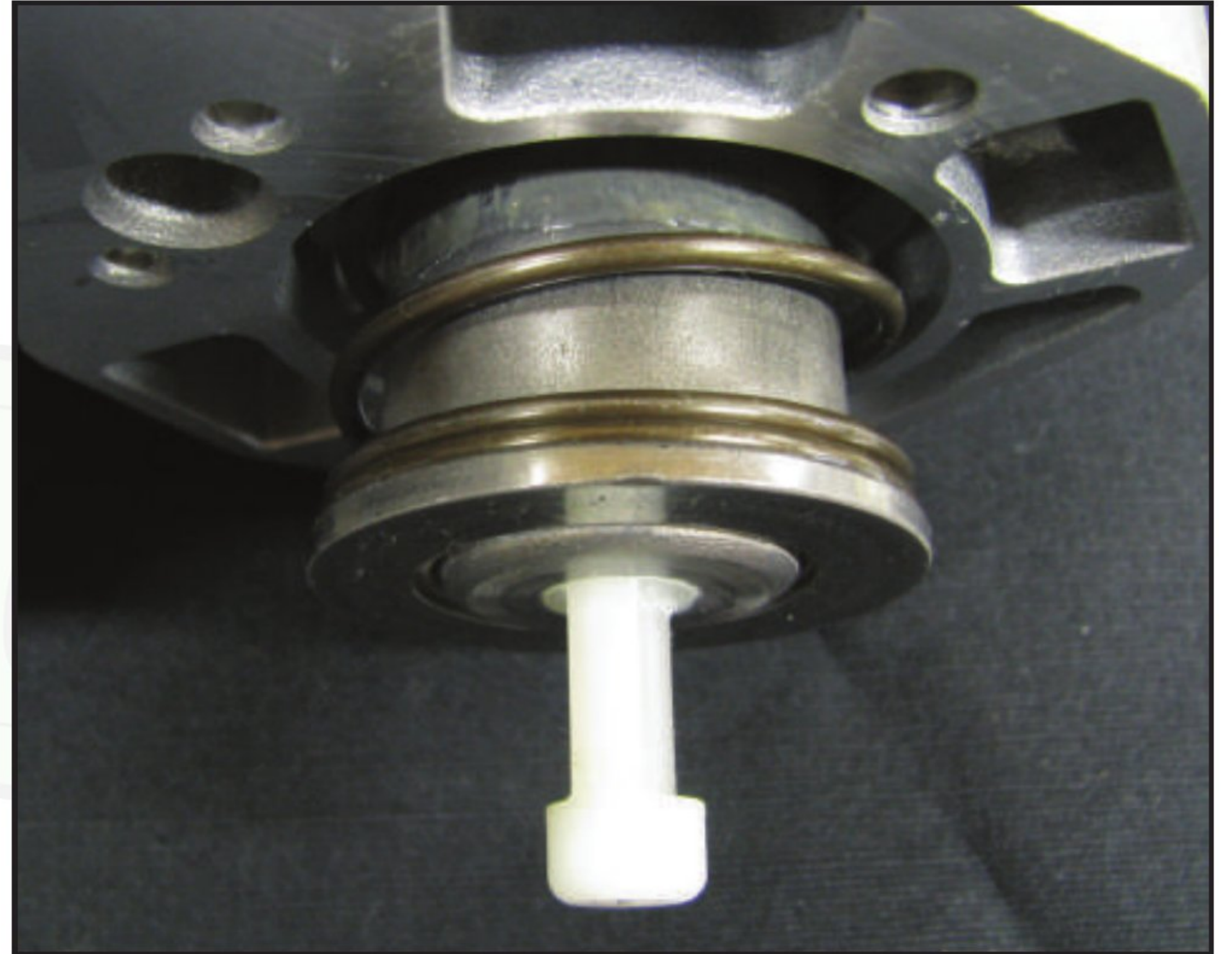
Figure 24 – PA90S plunger in its at rest position.
