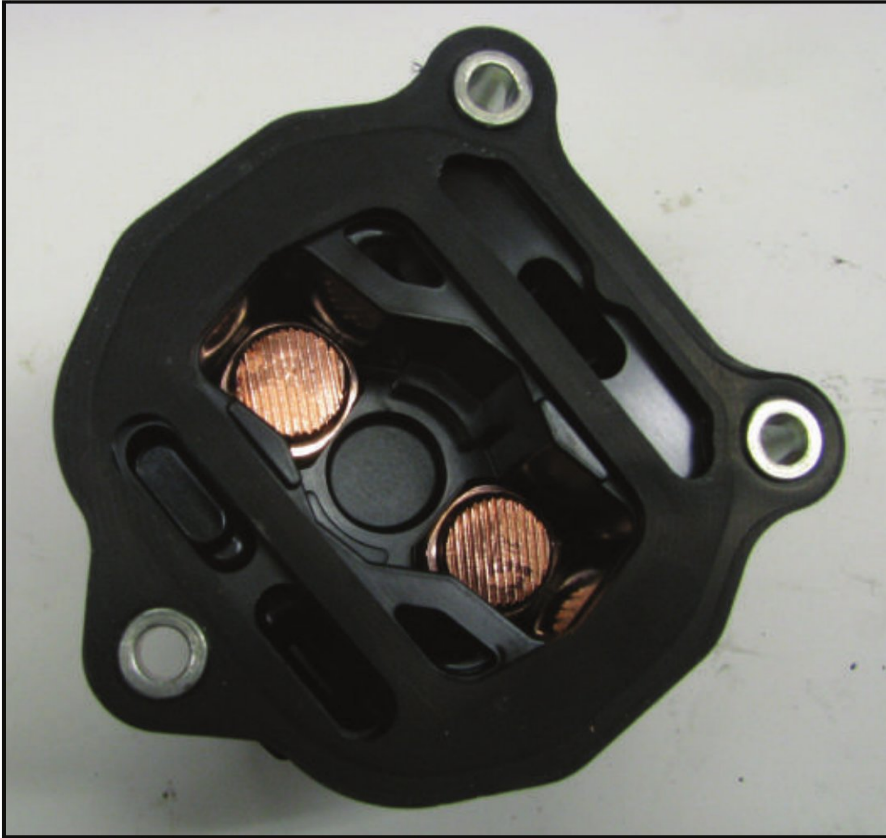
Figure 22 – A view looking inside the solenoid cap.
