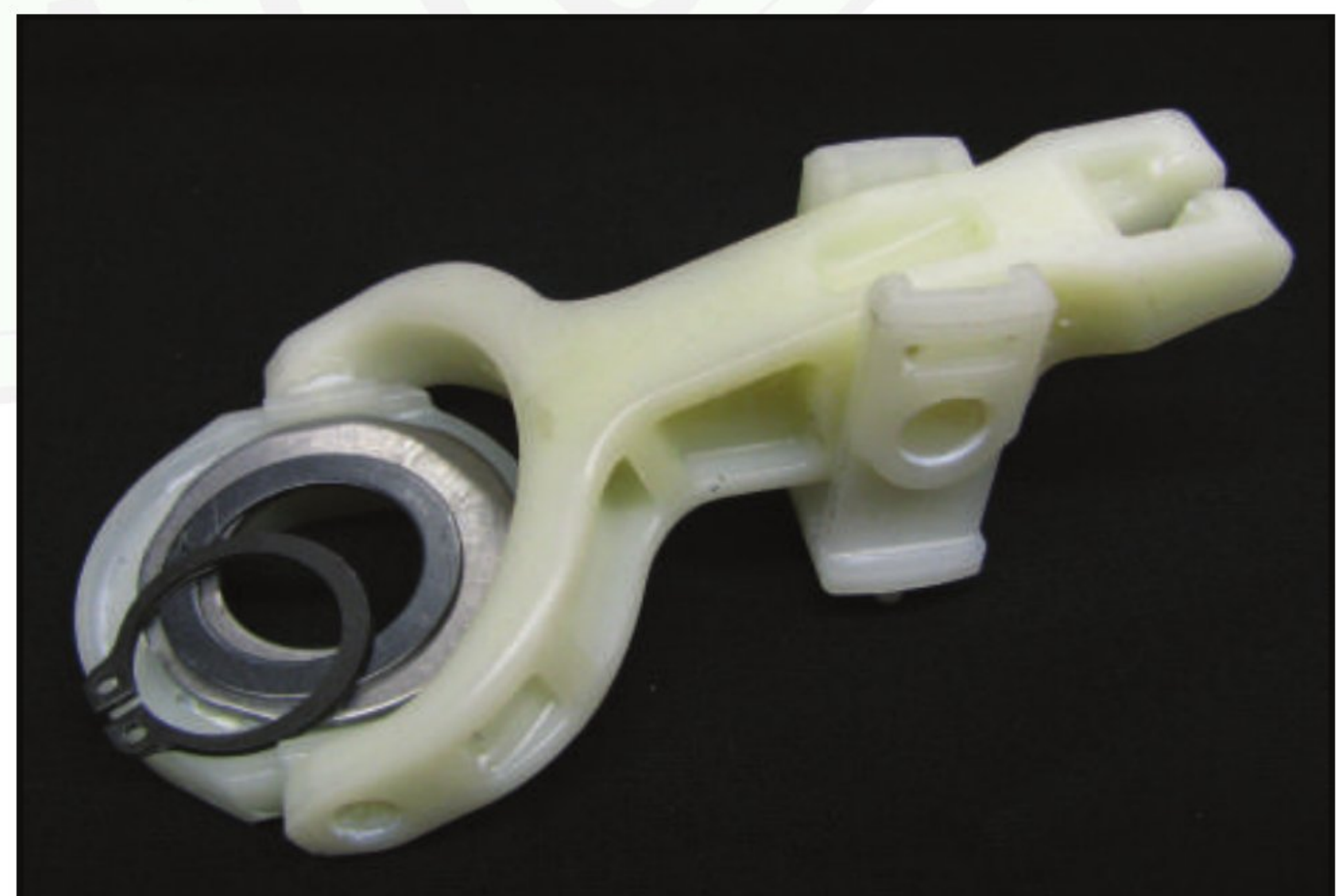
Figure 17 – A close view of the shift lever with washers and retaining ring shown in correct order.
