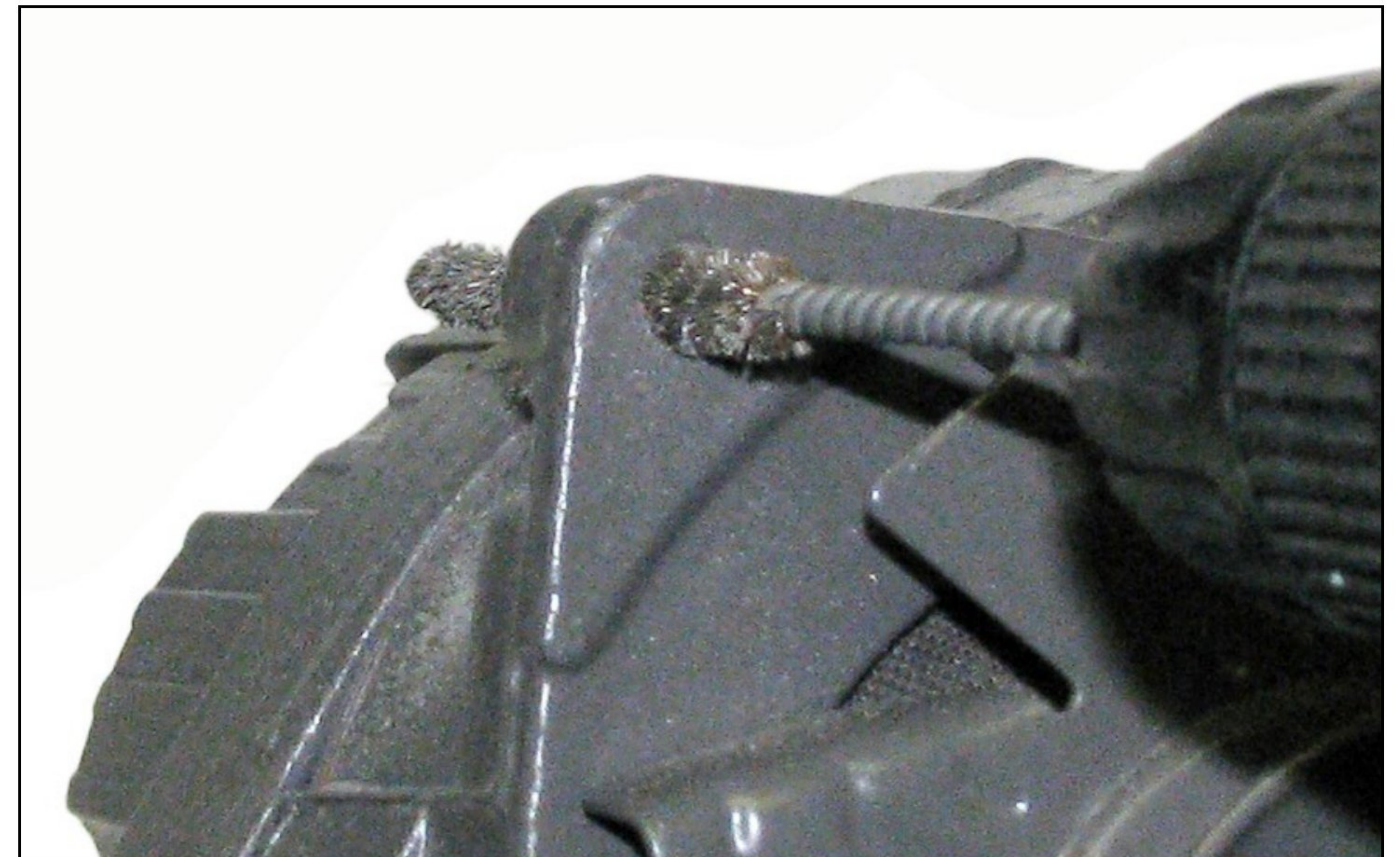
Figure 2—Cleaning a threaded hole
