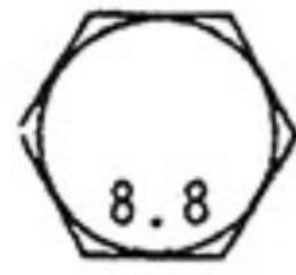
STANDARD THREAD - ZINC PLATED - CLASS 8.8
