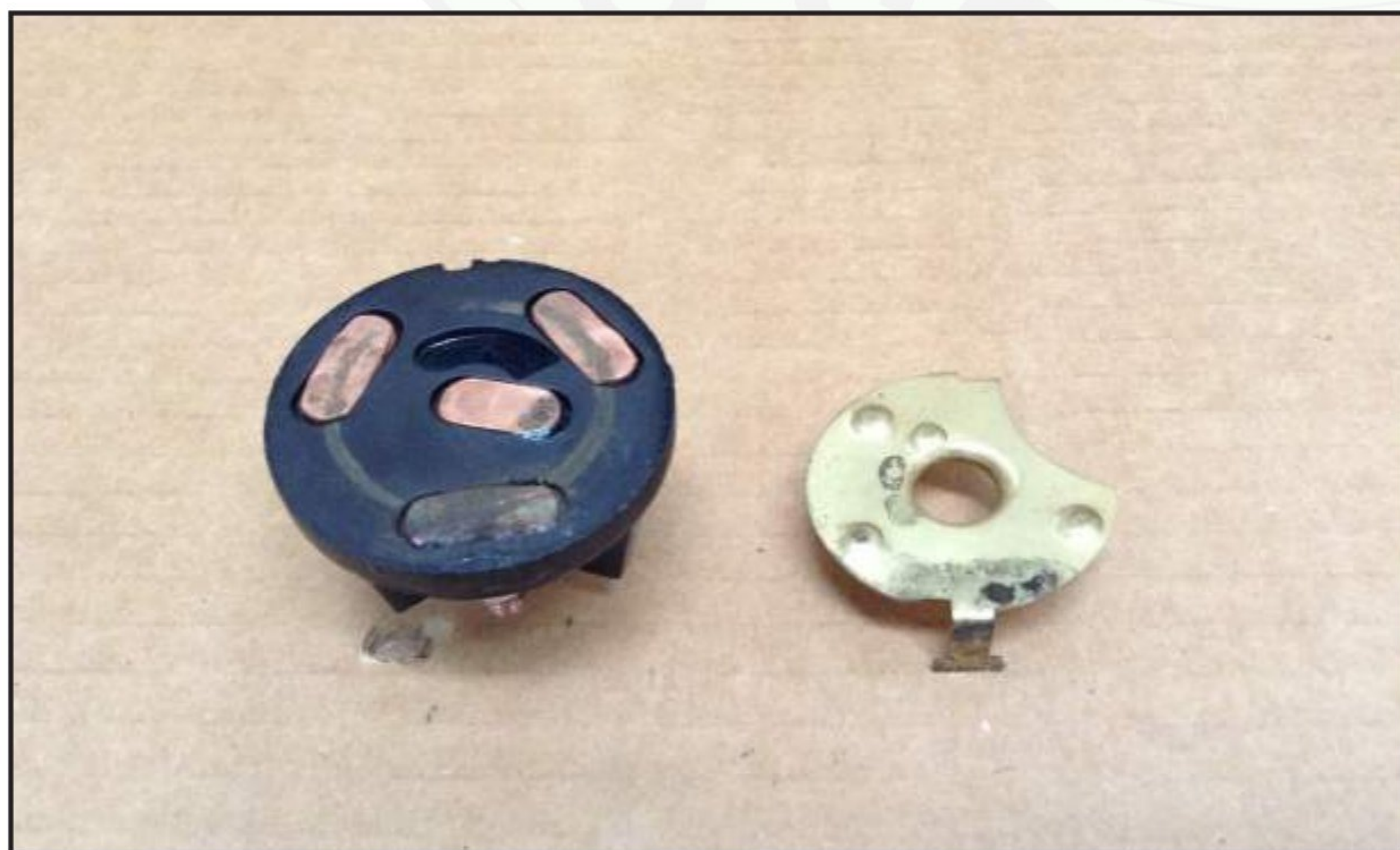
Figure 5 - Corrosion and conductive sludge inside the ignition switch caused the intermittent self cranking.
