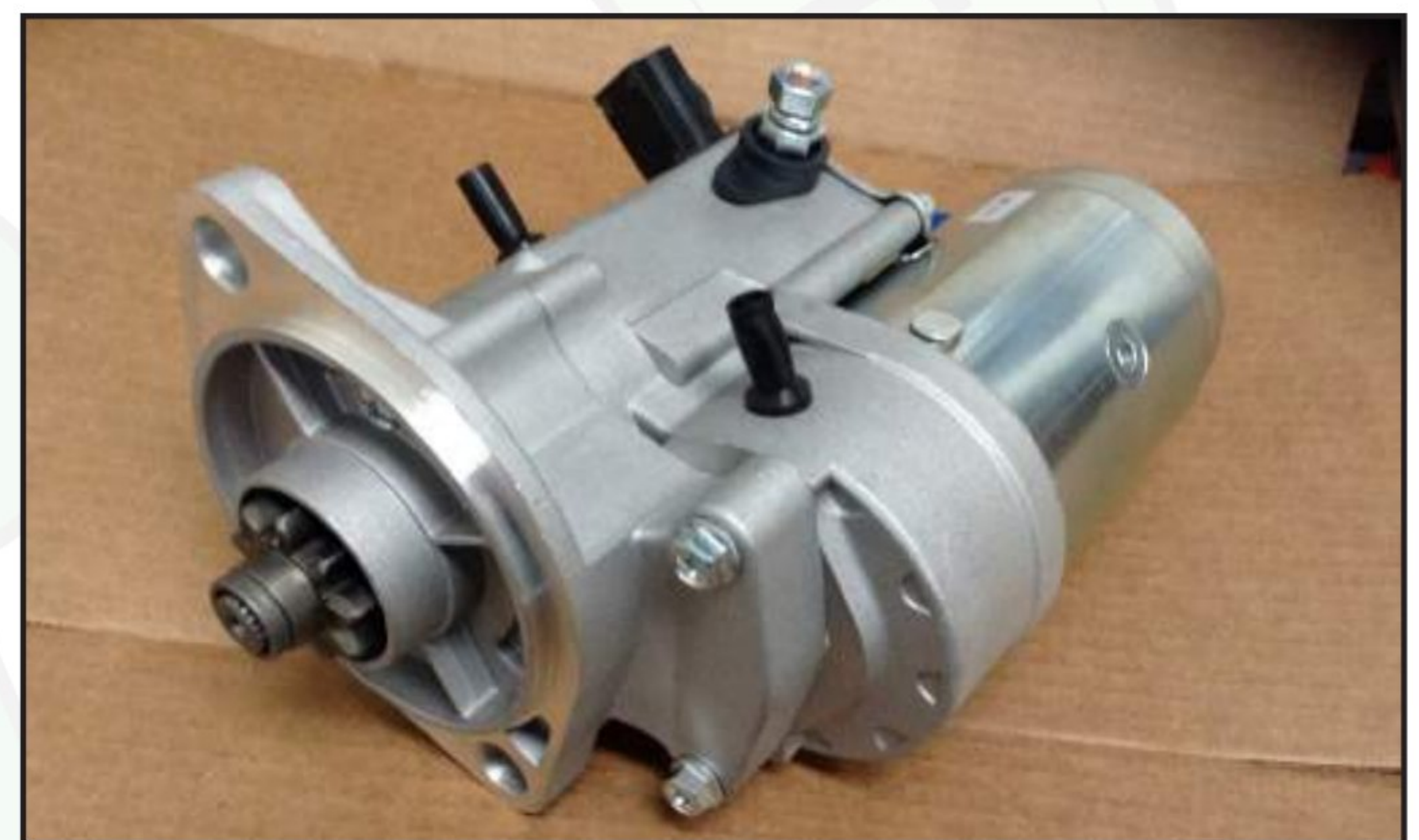
Figure 2 – 2.2kW Denso starter number 228000-9010.
