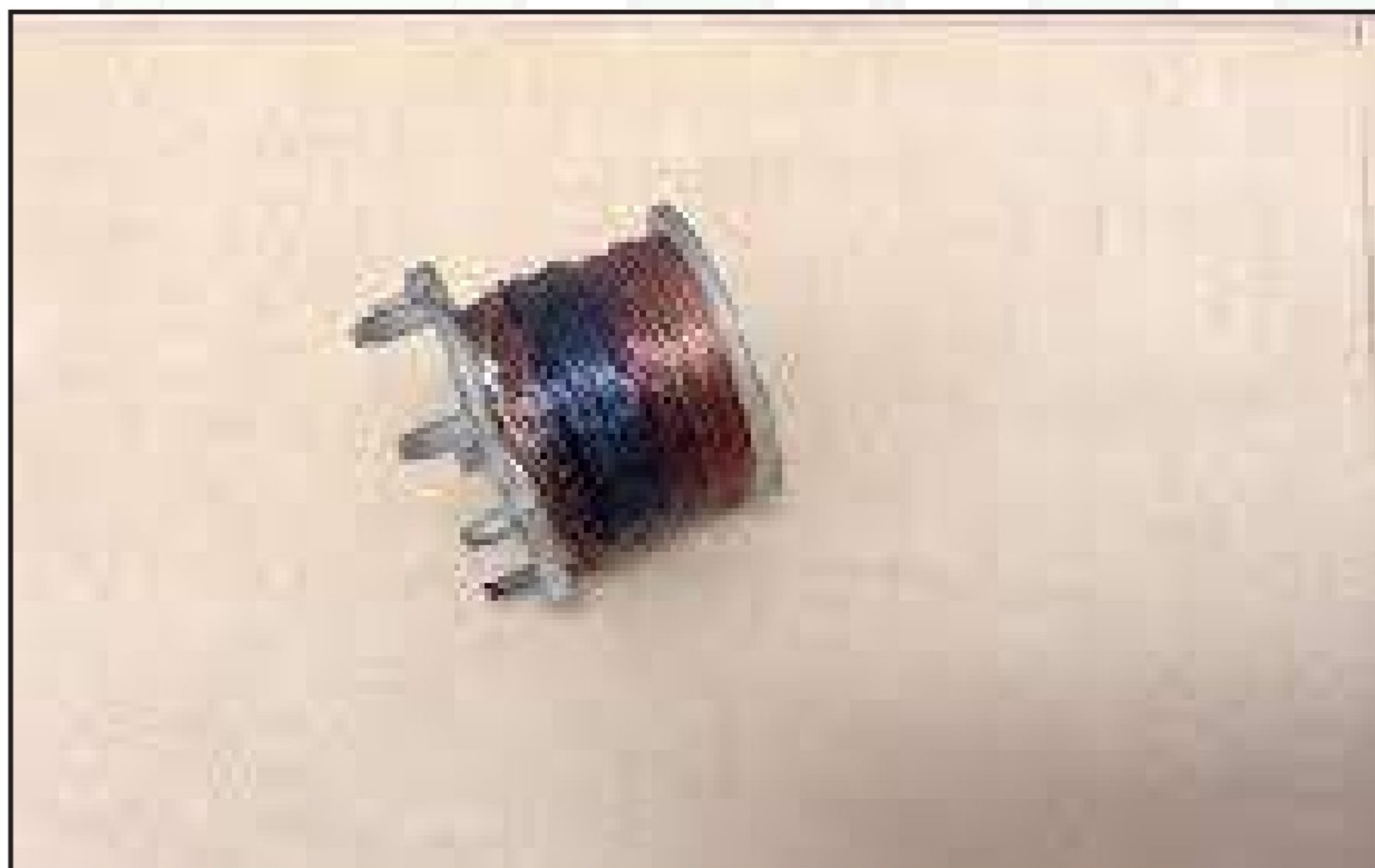
Figure 4 – The burned solenoid coil indicates the switch terminal was powered for an excessive amount of time.
