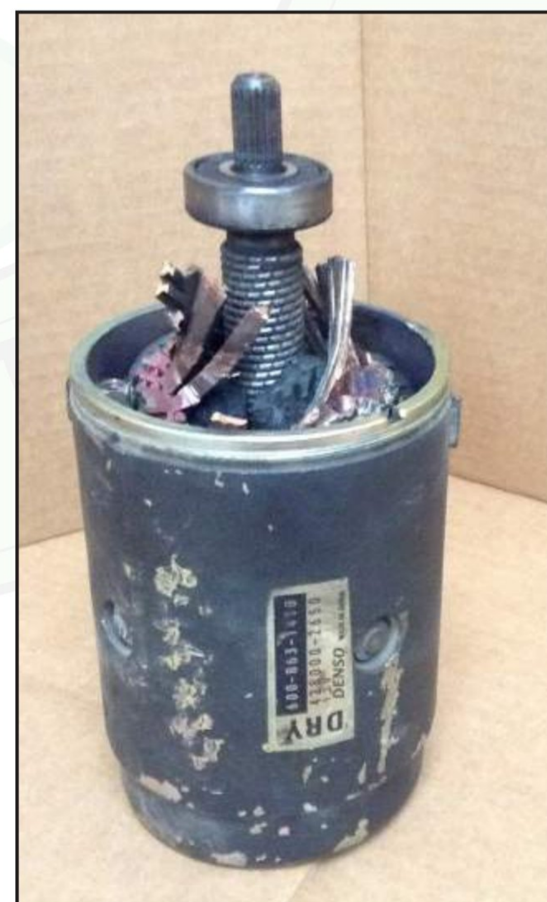
Figure 3 – Exploded commutator is convincing proof that this starter was engaged with engine running.
