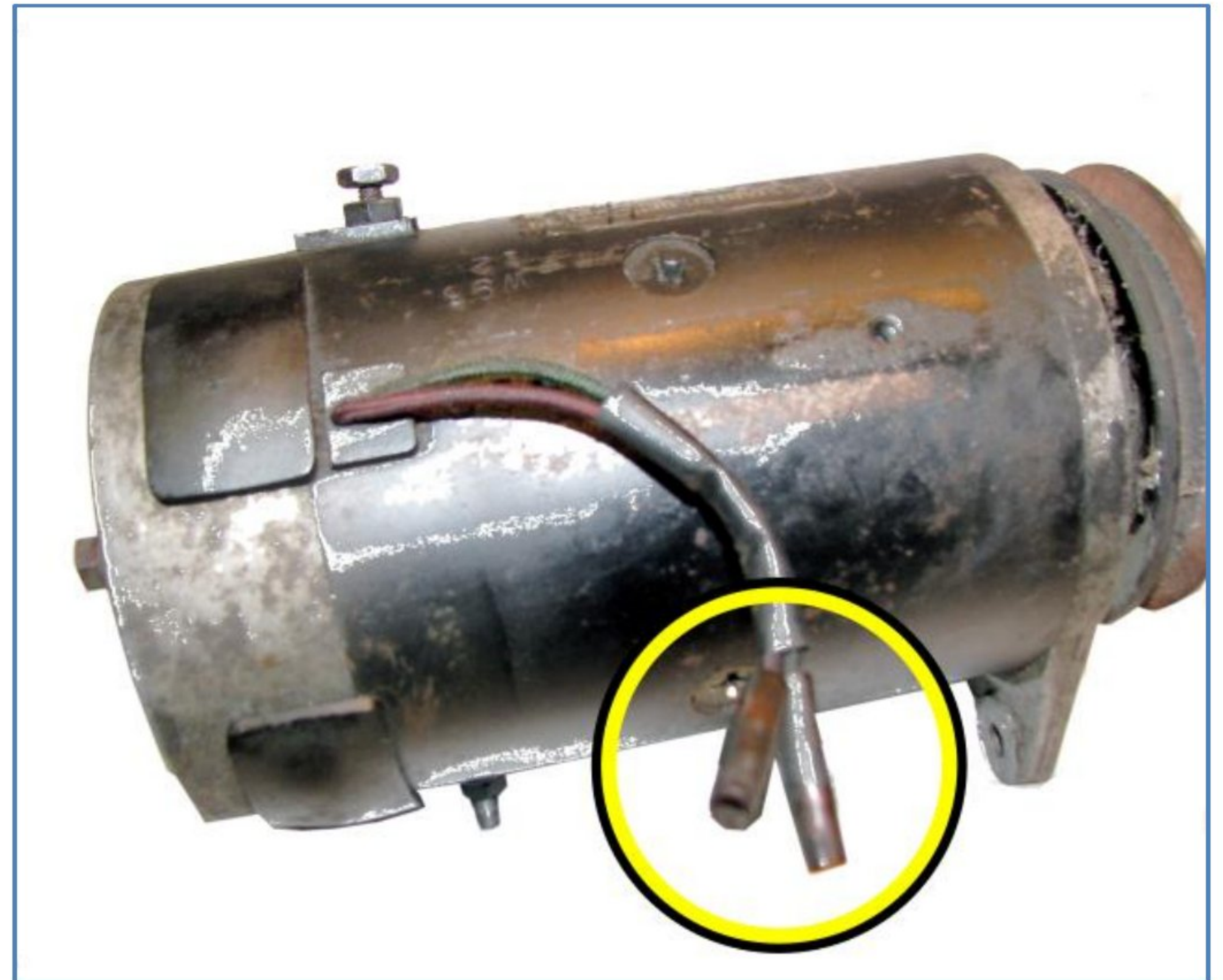
Figure 7—Generator-Coil Bullet Connectors
