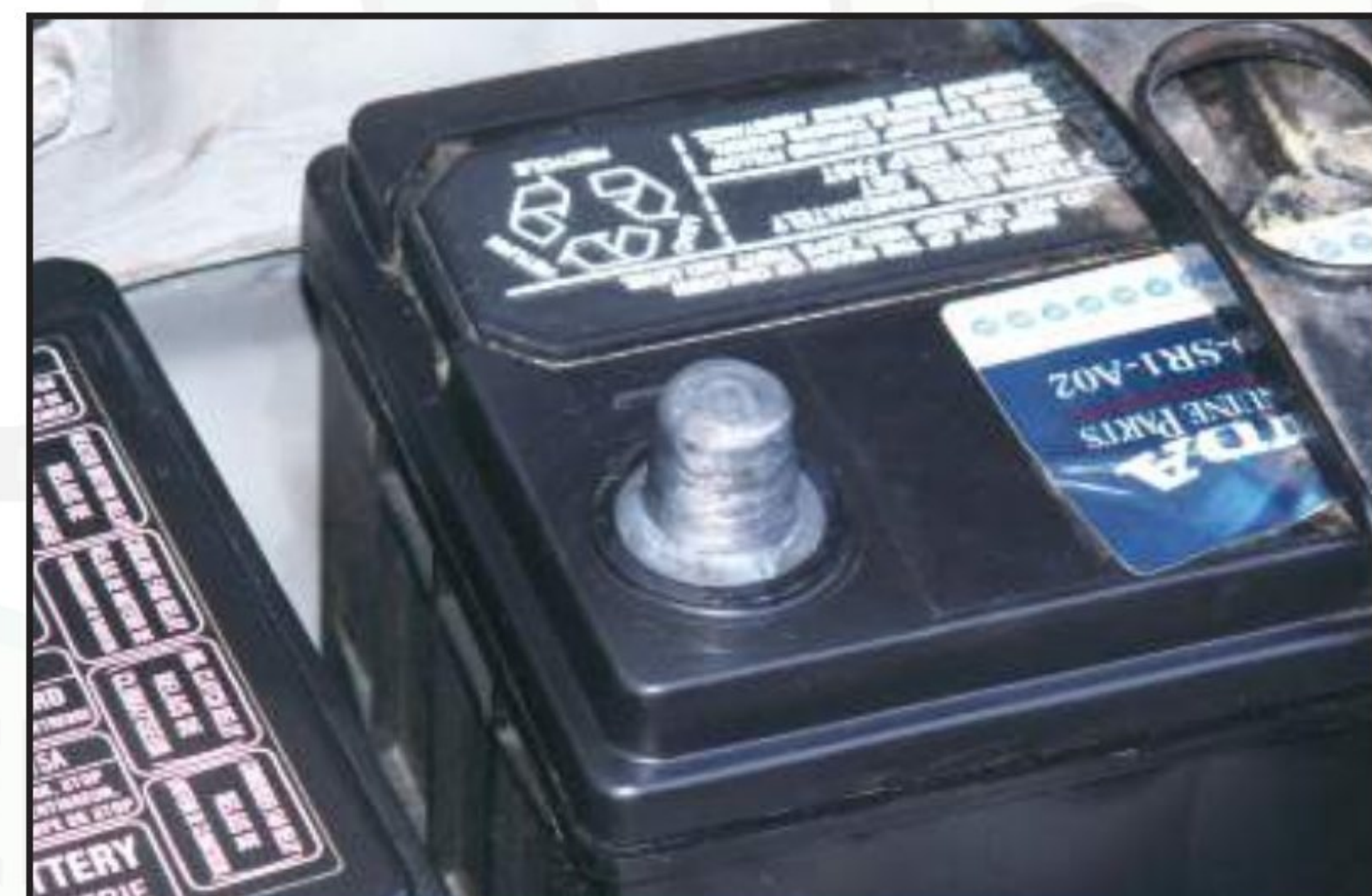
Figure 2 – This is common Honda battery terminal that I have cleaned and treated with a film of silicone paste. Years of experience has shown me that I remove the battery cables from this battery years from now, the battery post will still look just like this one.
