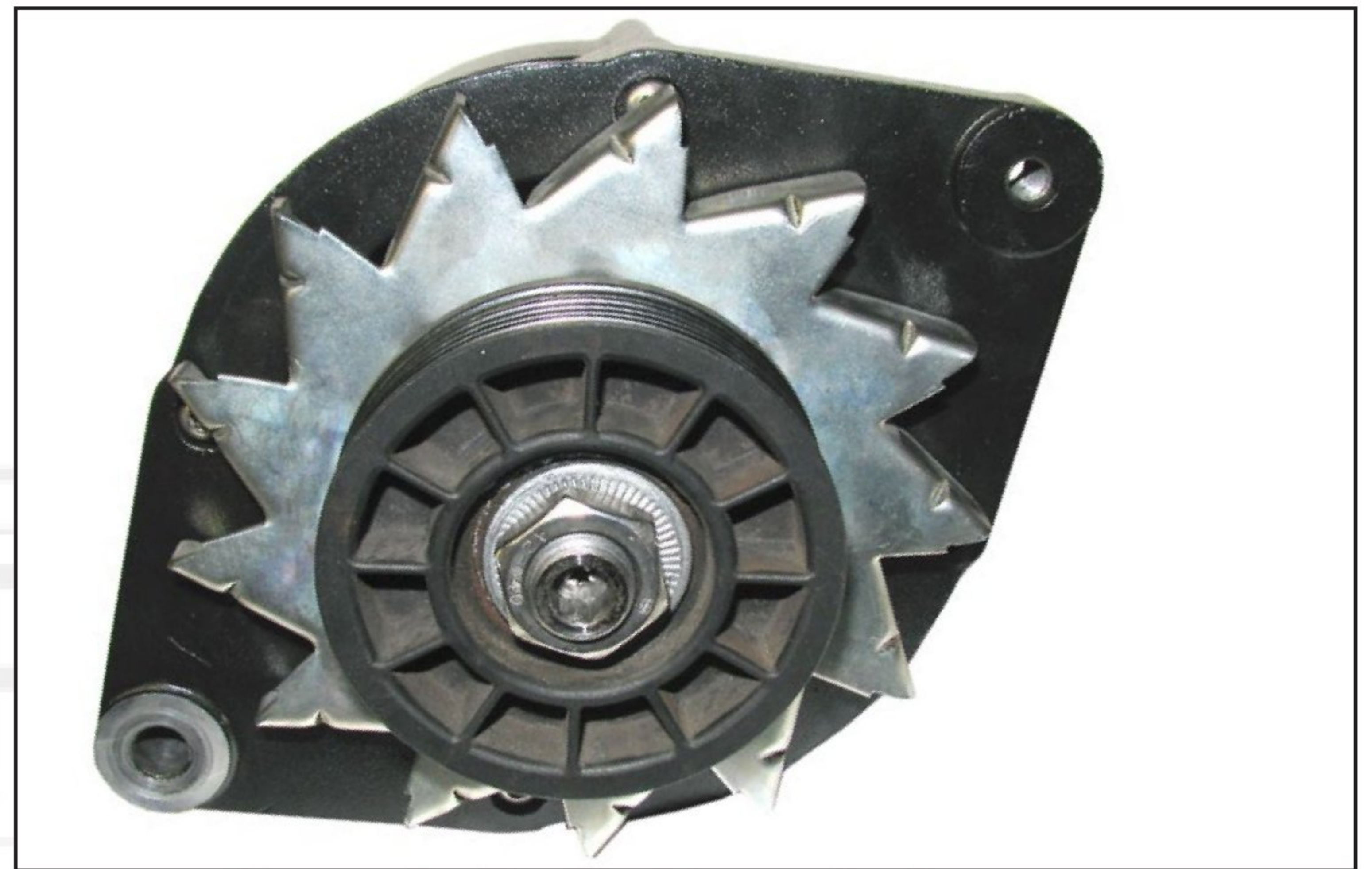
Figure 5—All Thermo King TriPac™ APU alternators must have a CCW fan for proper cooling.
