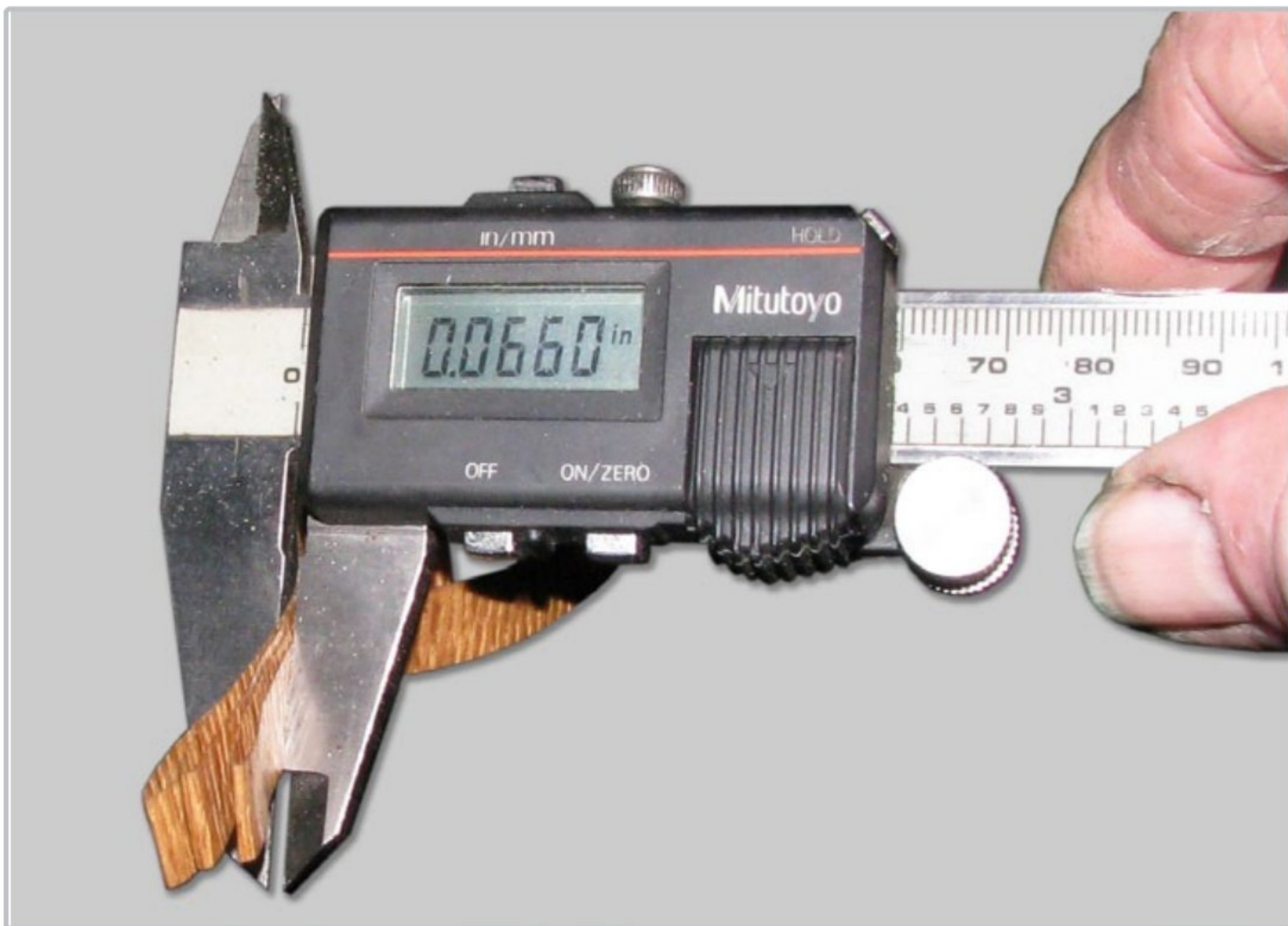
Figure 7—Measuring Six Layers of Coil Wrap
