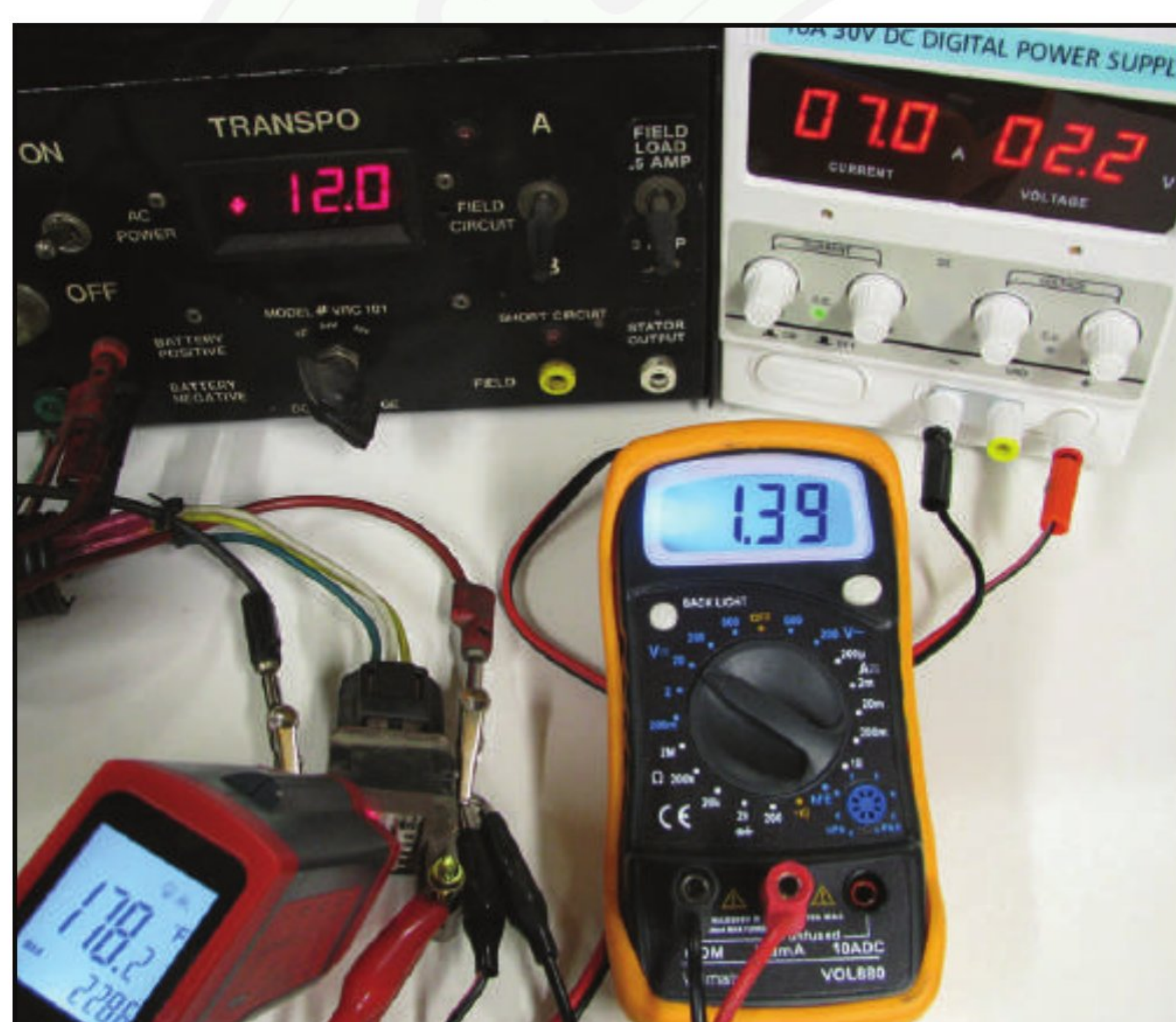
Figure 7 – After heating the regulator to 178 F, the Vsat increased to 1.39v.
