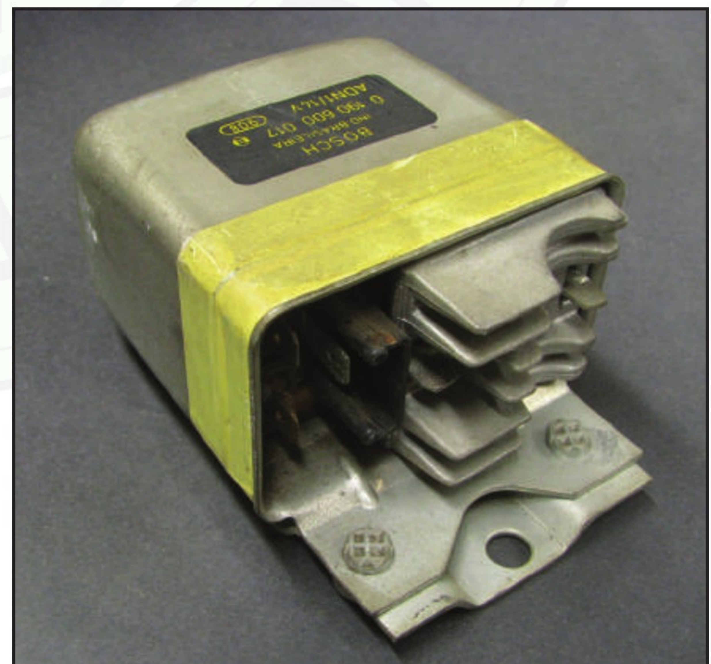
Figure 3 – This Bosch electronic regulator was cutting edge technology 50 years ago. The size of its heat sink is telling of early transistor efficiency.
