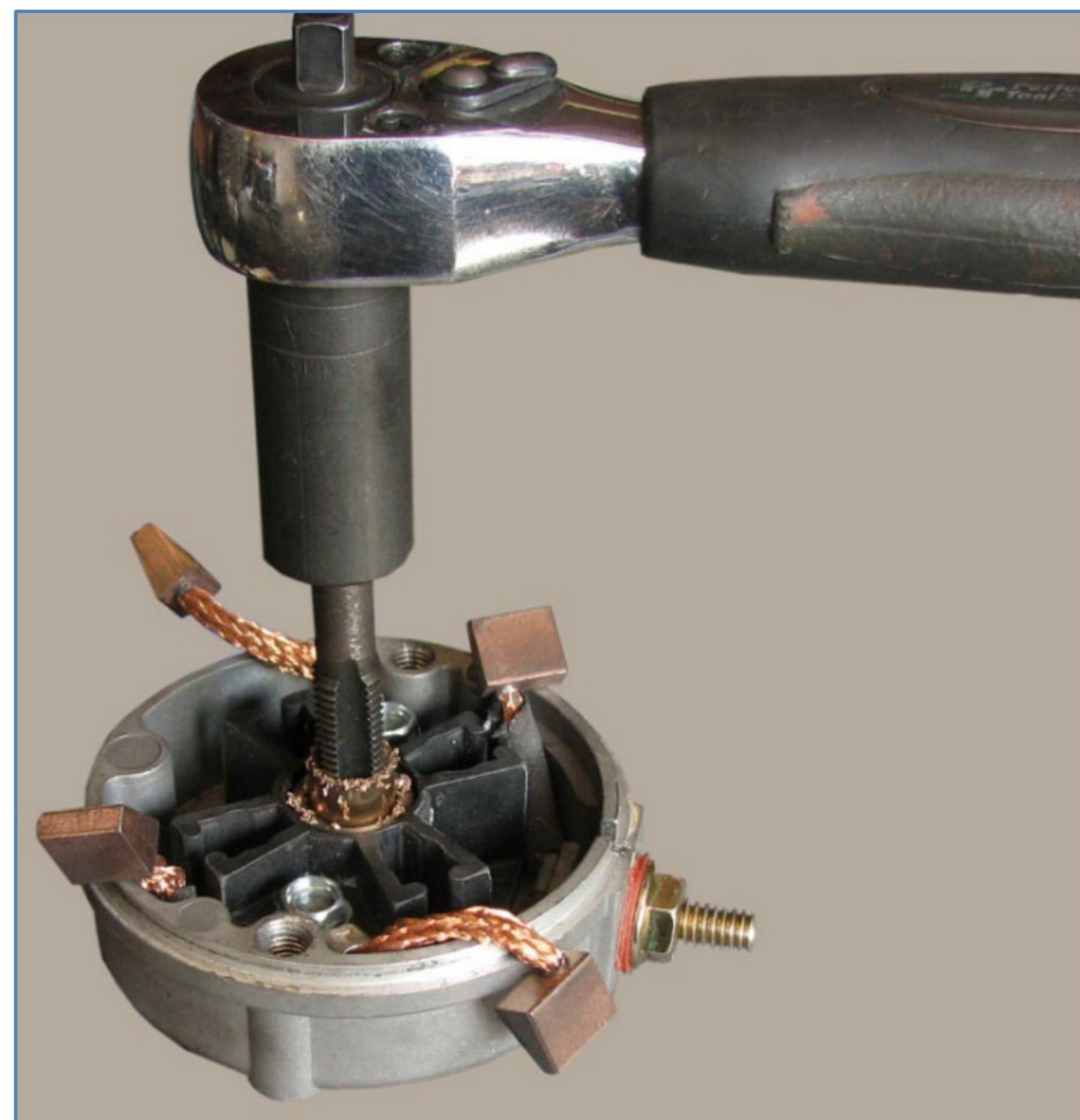
Figure 1—Bushing Is Starting To Come Out
