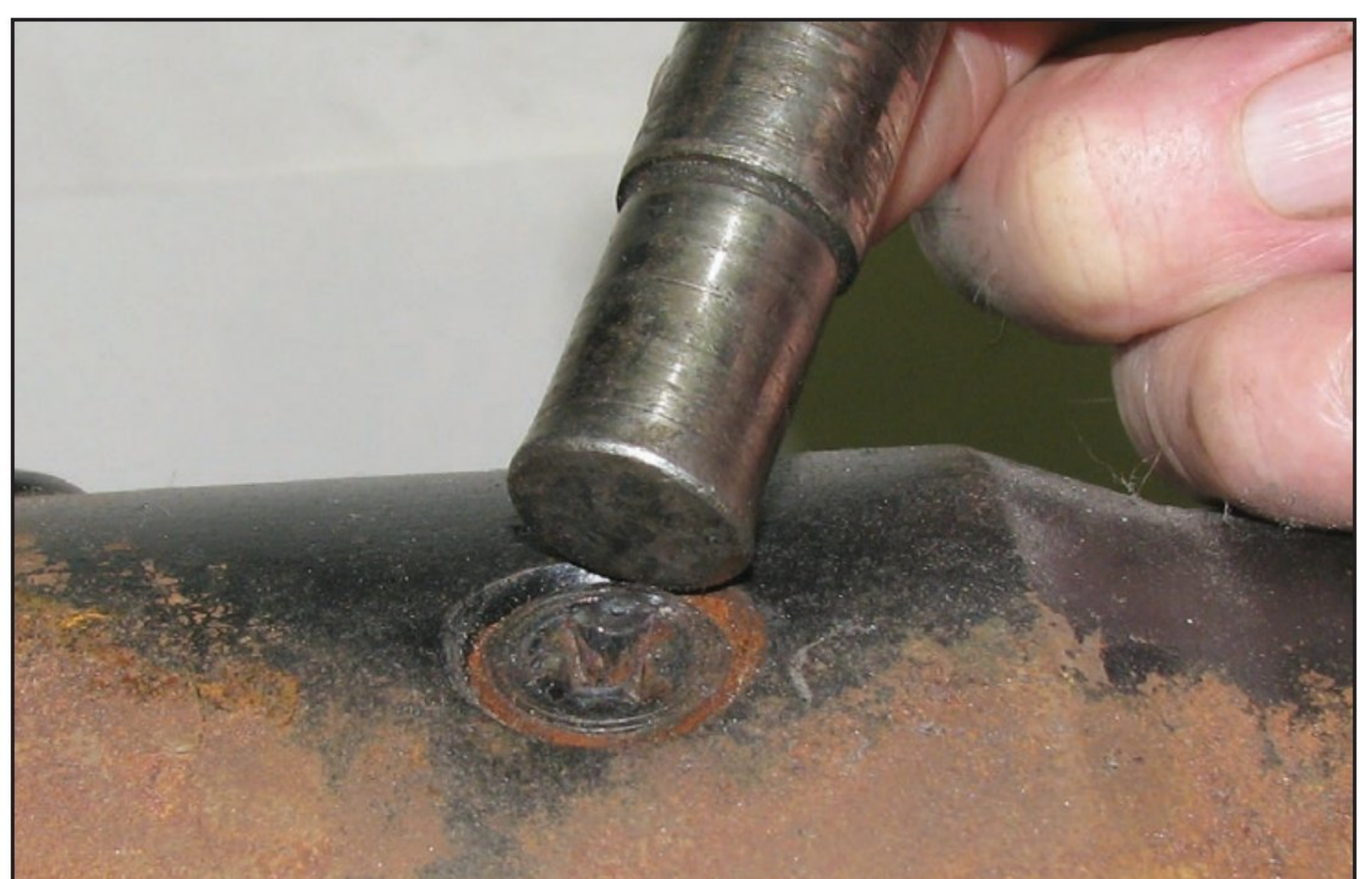
Figure 5—Tool made from armature shaft
