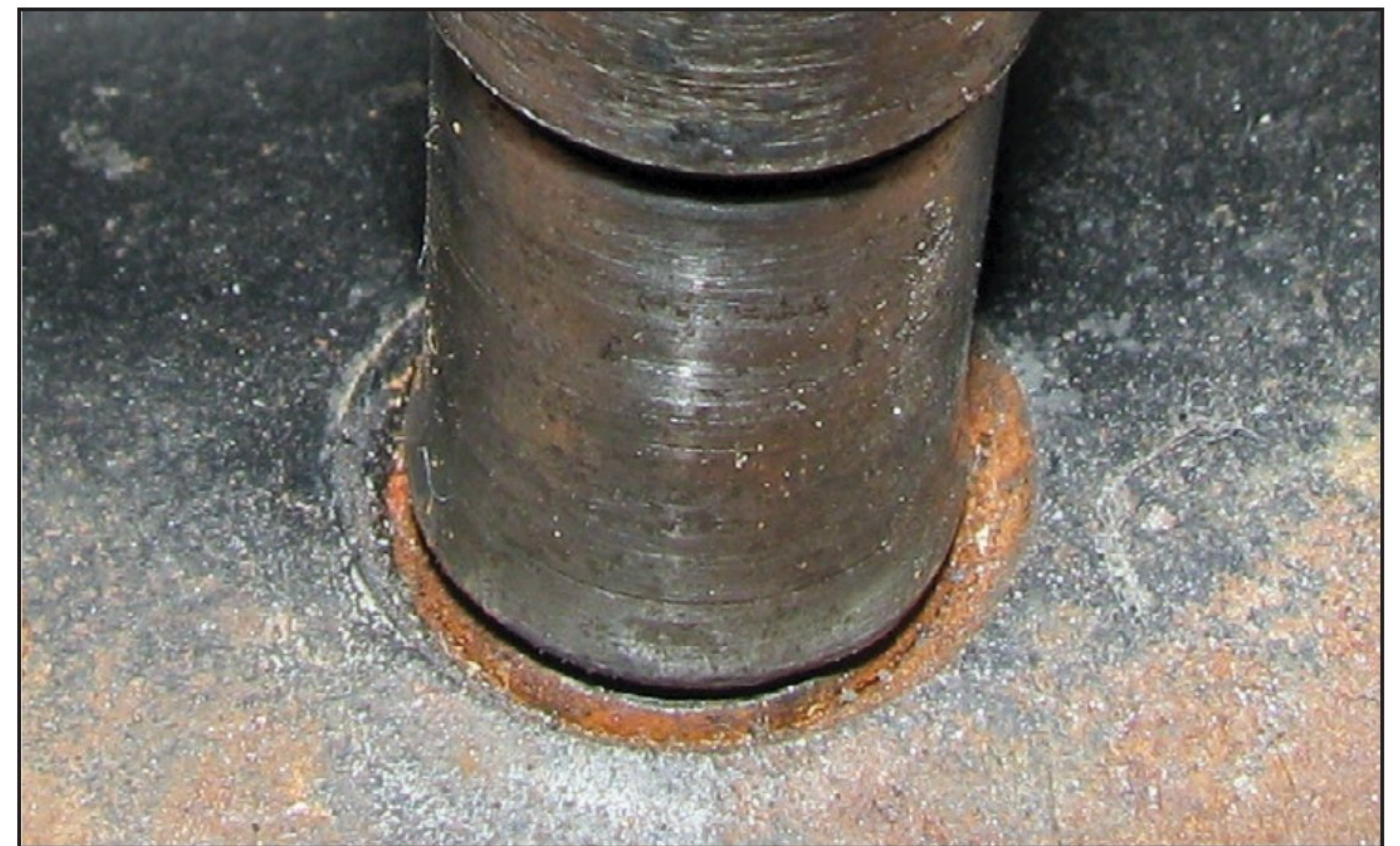
Figure 6—The tool is slightly smaller than the screw head.
