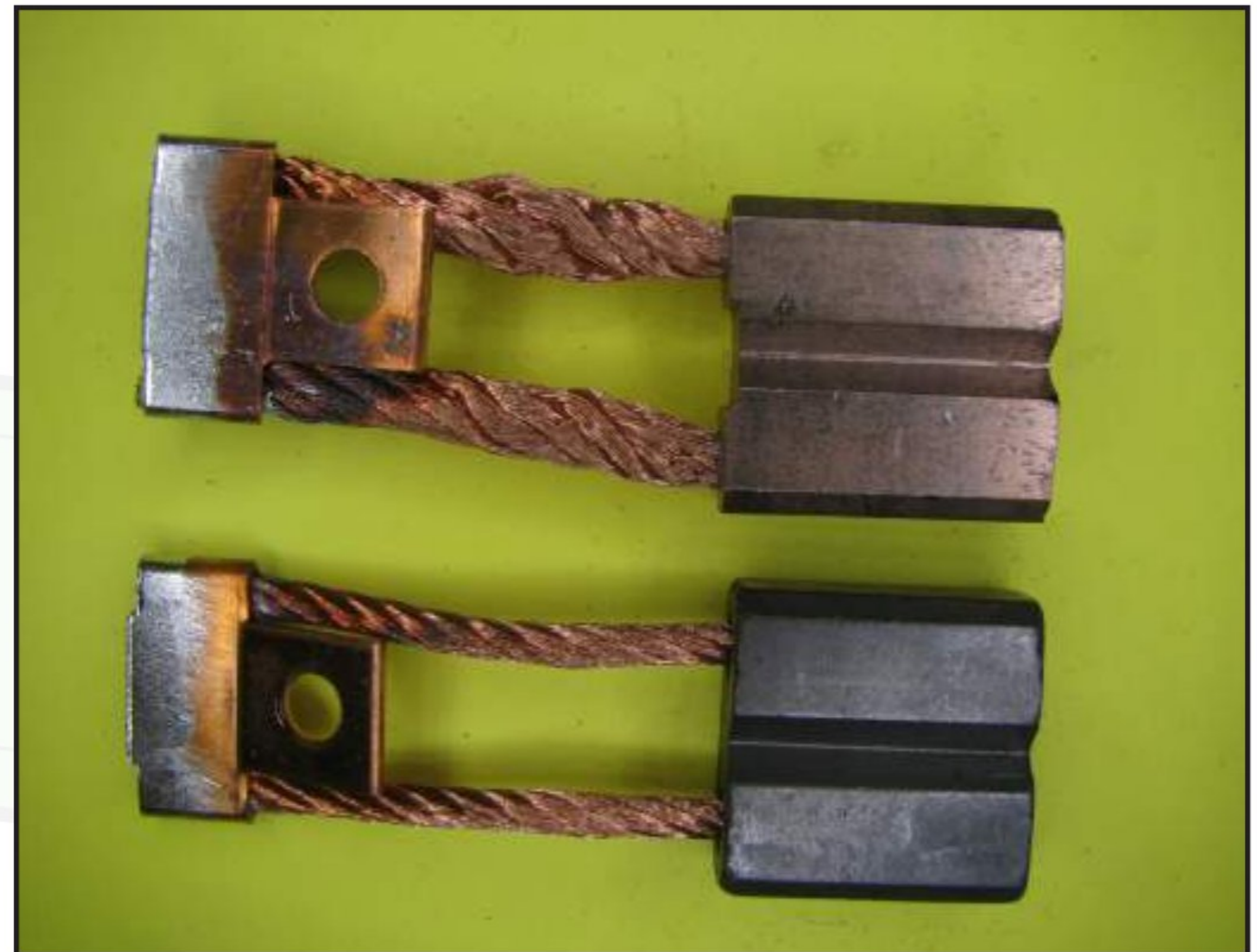
Figure 6 – These 40MT brushes are for different voltages - less copper and smaller wire for 32 volts - more copper and heavier wire for 12 volts.
