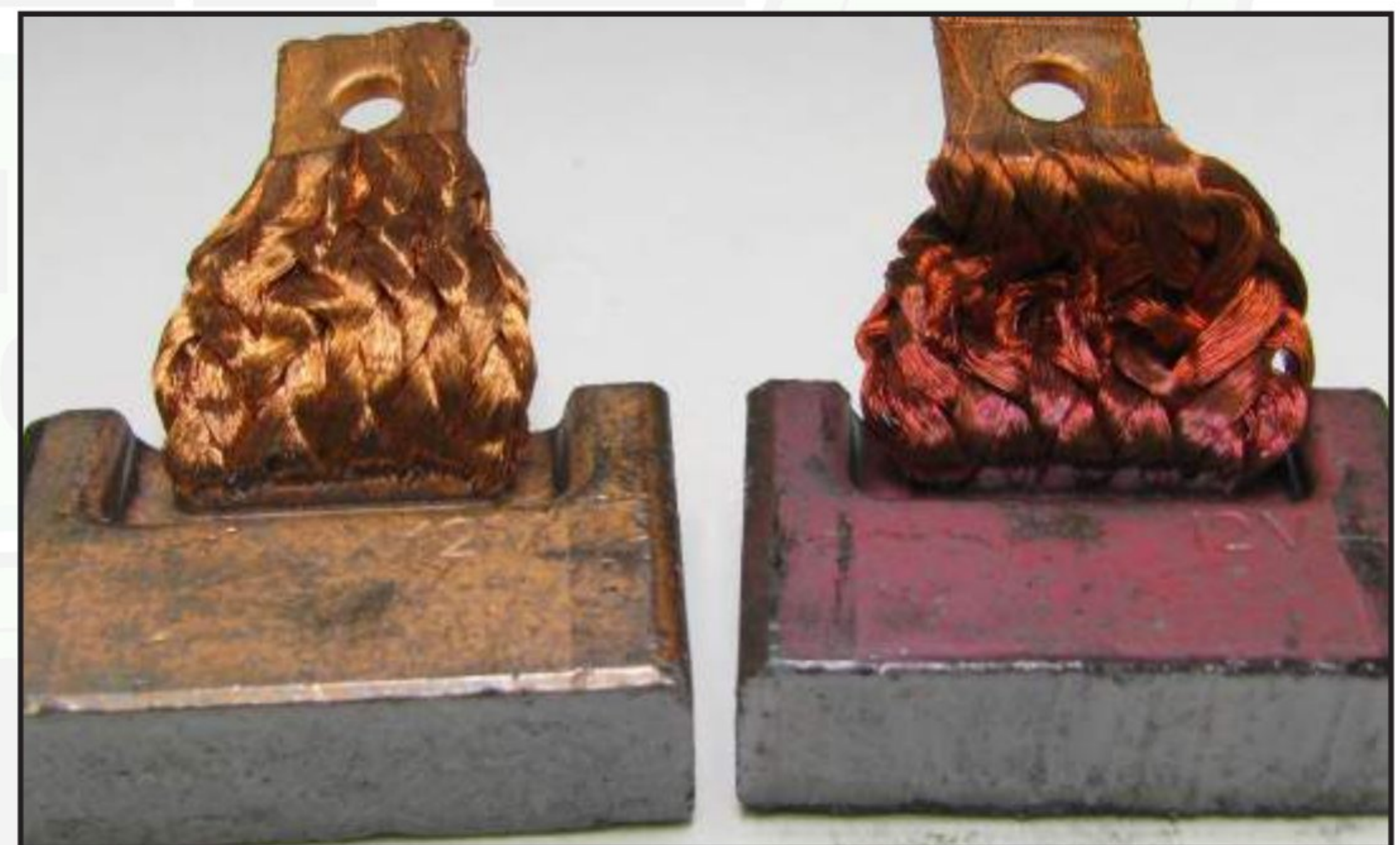
Figure 10 – Notice the reddish discoloration of the used brush on the right, caused by extended over-cranking.
