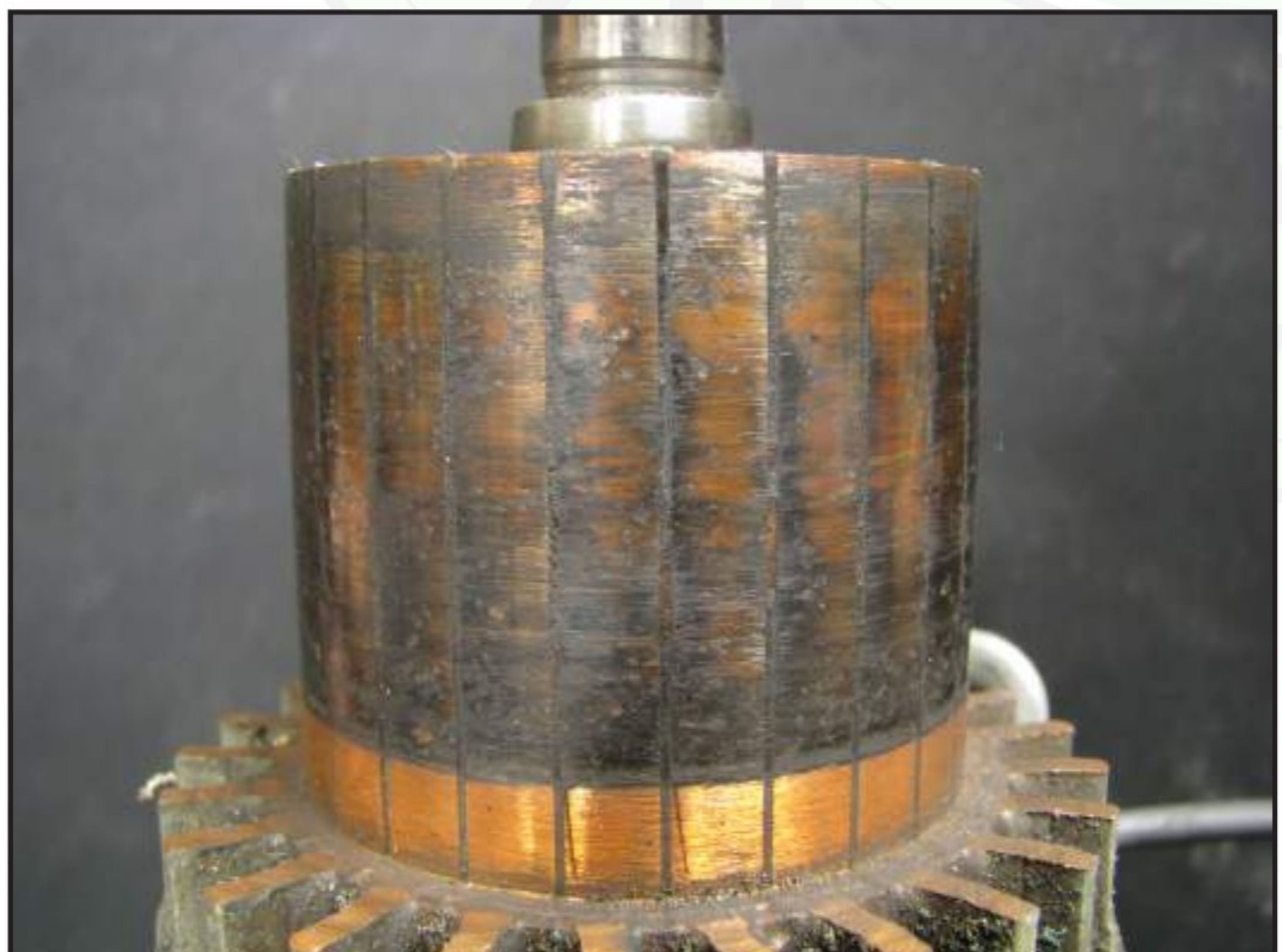
Figure 4 – This 42MT commutator shows damage by reactance voltage in addition to excessive arcing from over cranking.
