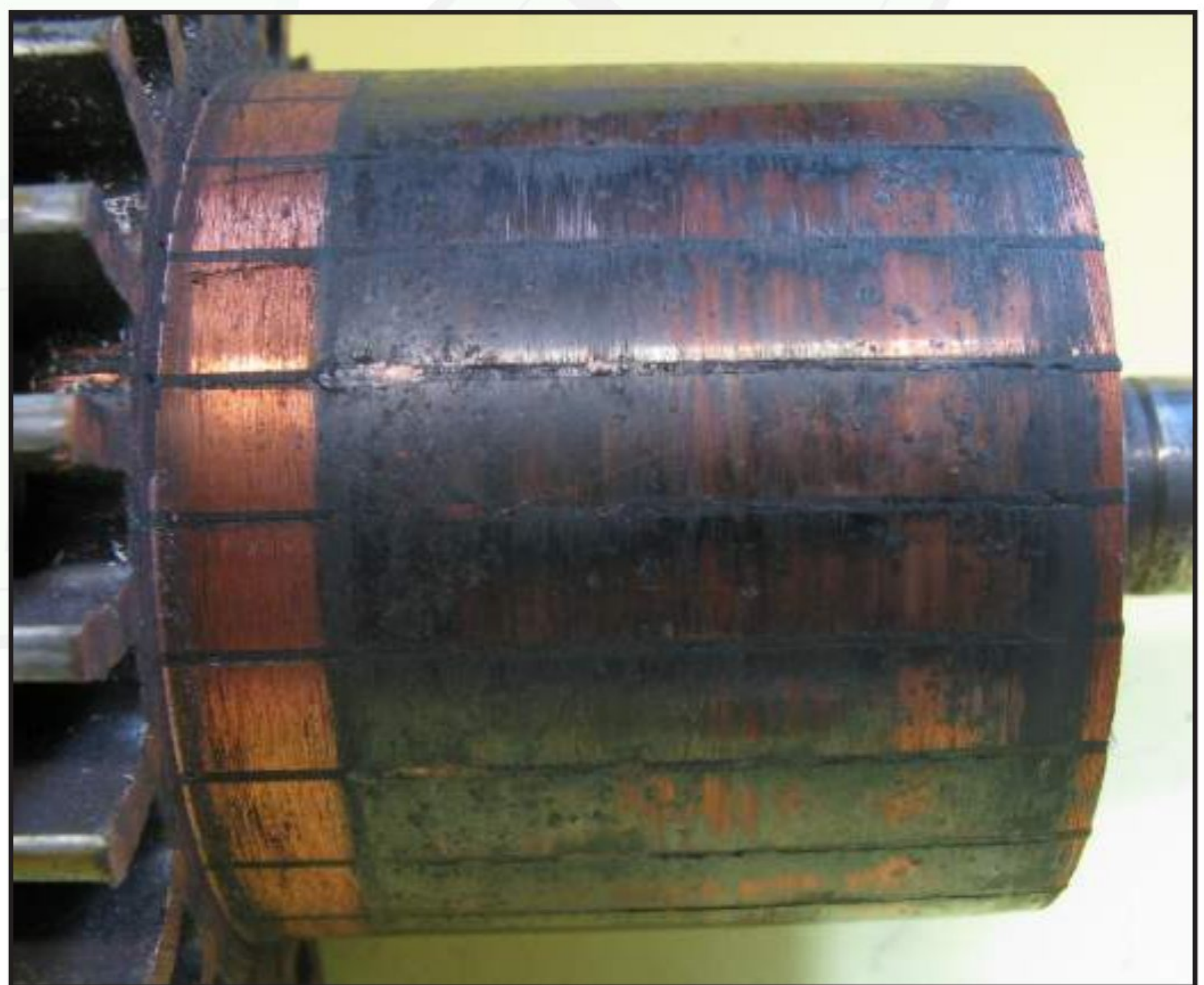
Figure 8 – This 42MT commutator shows evidence of extended over-cranking. The discoloration indicates extreme over heating. The burn marks are from arcing.
