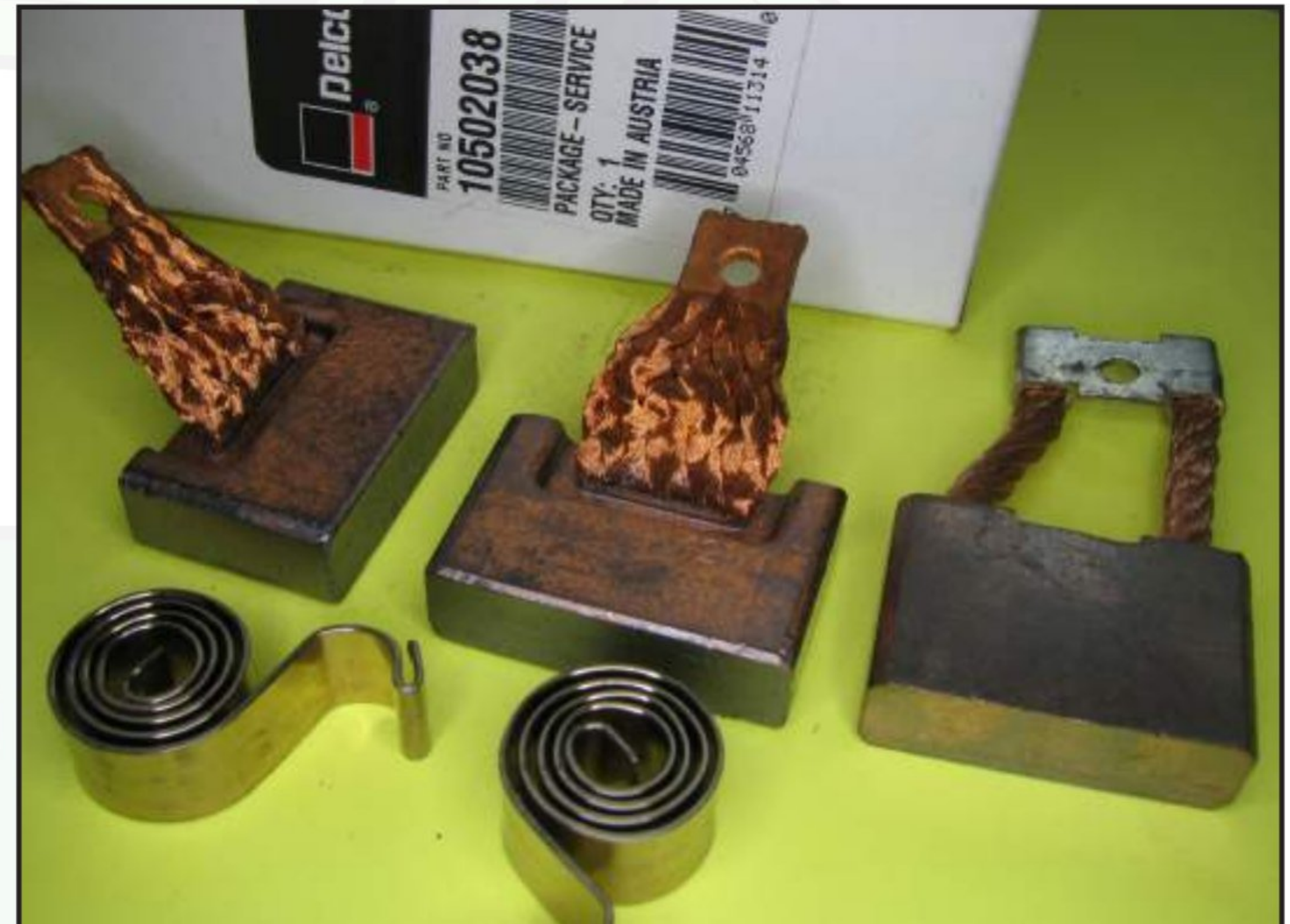
Figure 9 – Notice the difference in the shunts between the latest version and the original on the right.
