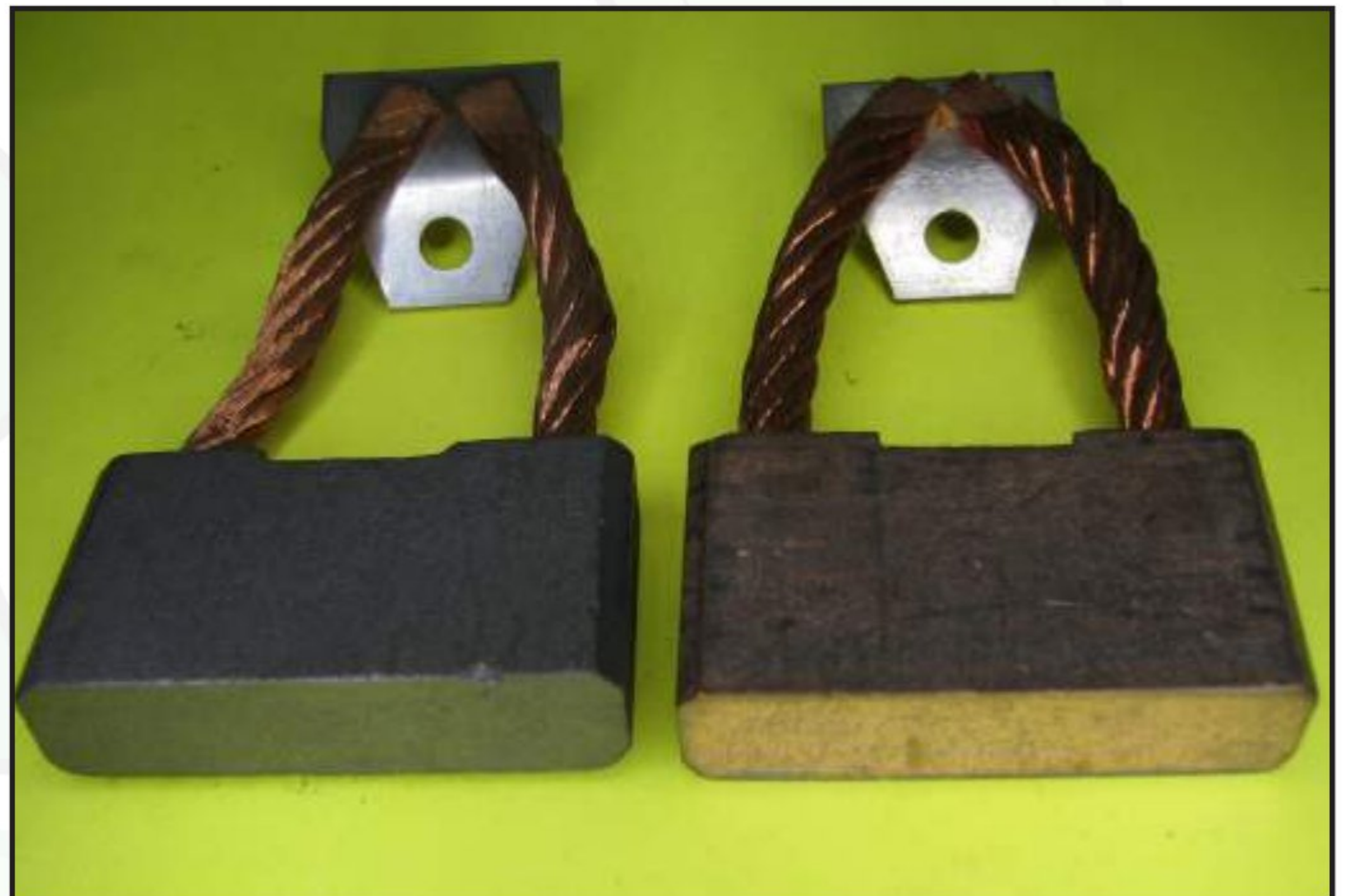
Figure 7 – The early style 42MT brush on the left is 24 volts while the one on the right is 12 volts.
