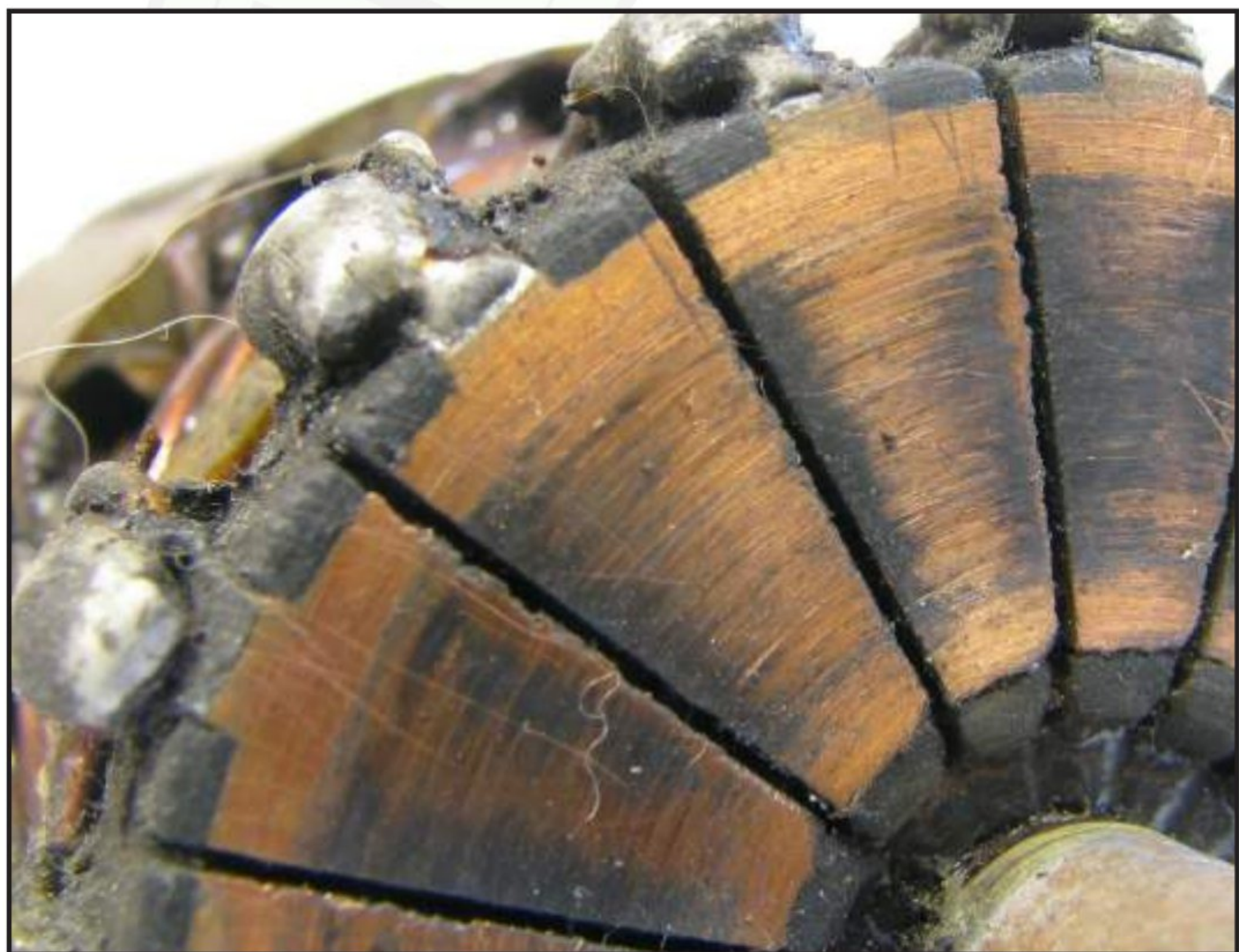
Figure 3 – The darkened areas along the trailing edge of the bars on this flat commutator were caused by reactance voltage. It is normal.
