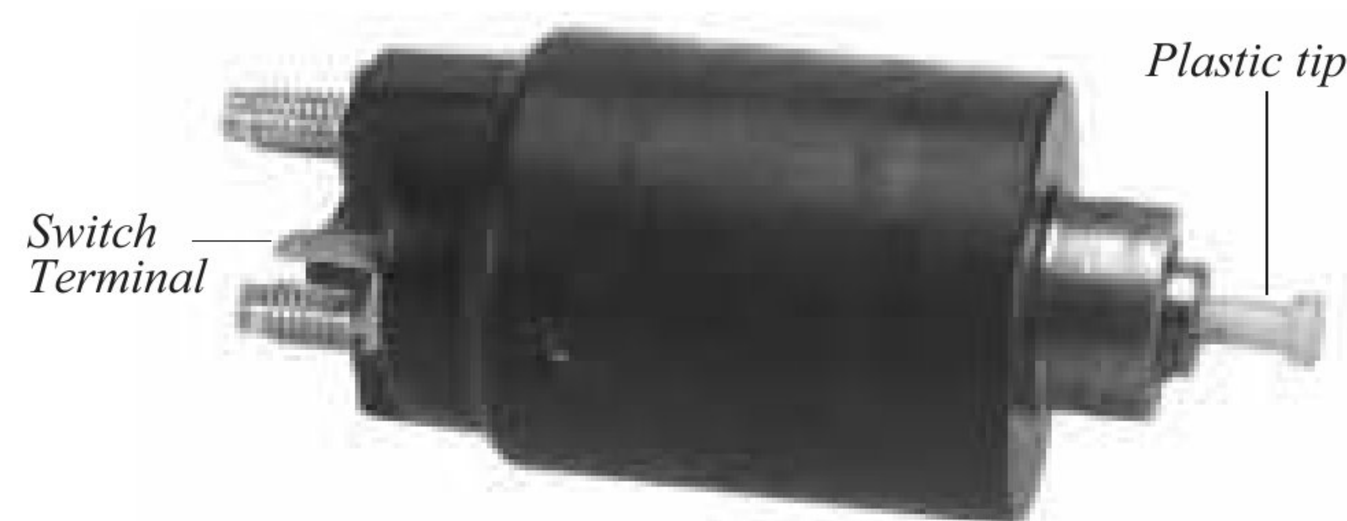
Figure 1. Pressing on the plastic plunger tip will destroy it.
