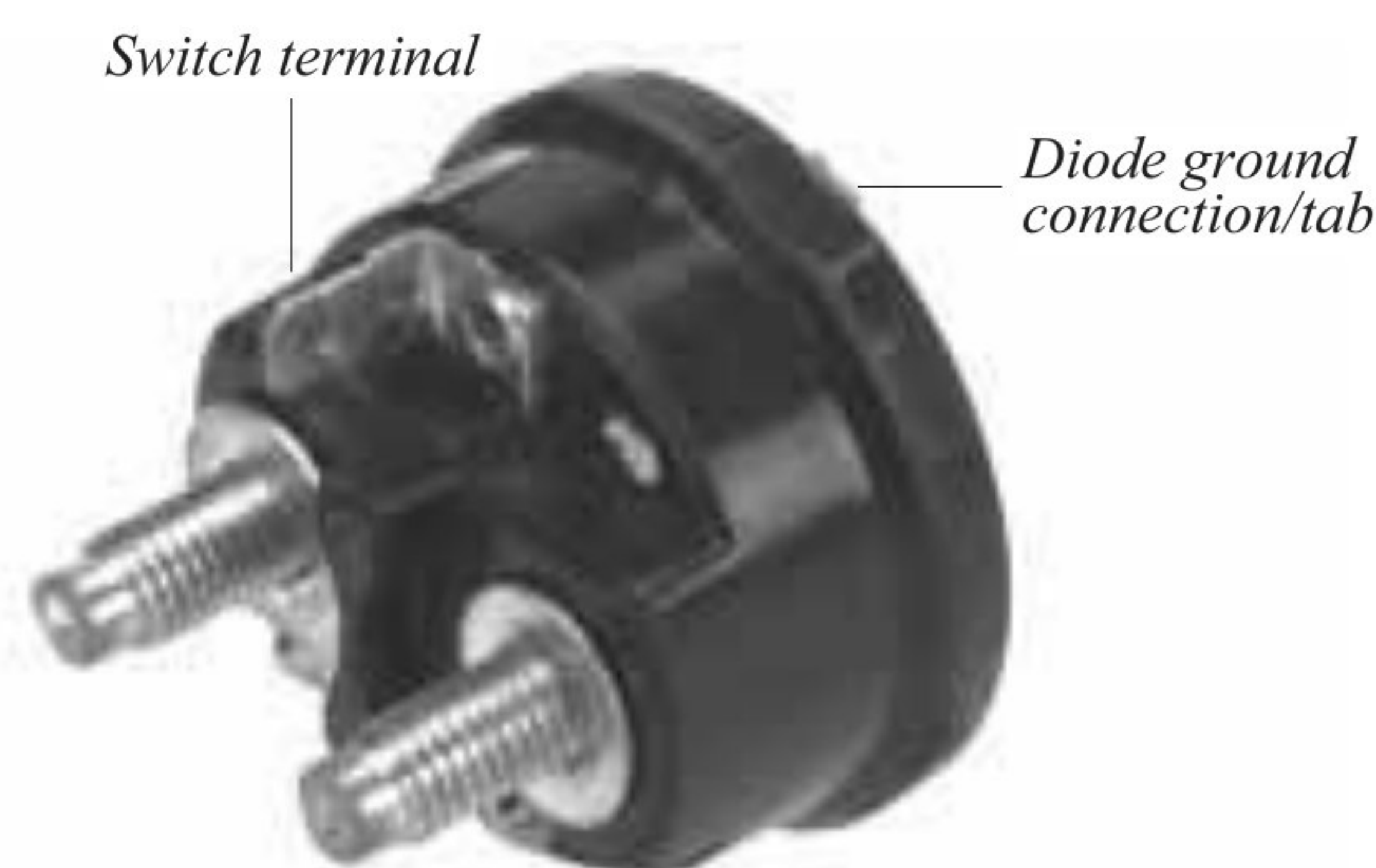
Figure 2. Some Ford solenoids have a diode molded into the cap.
