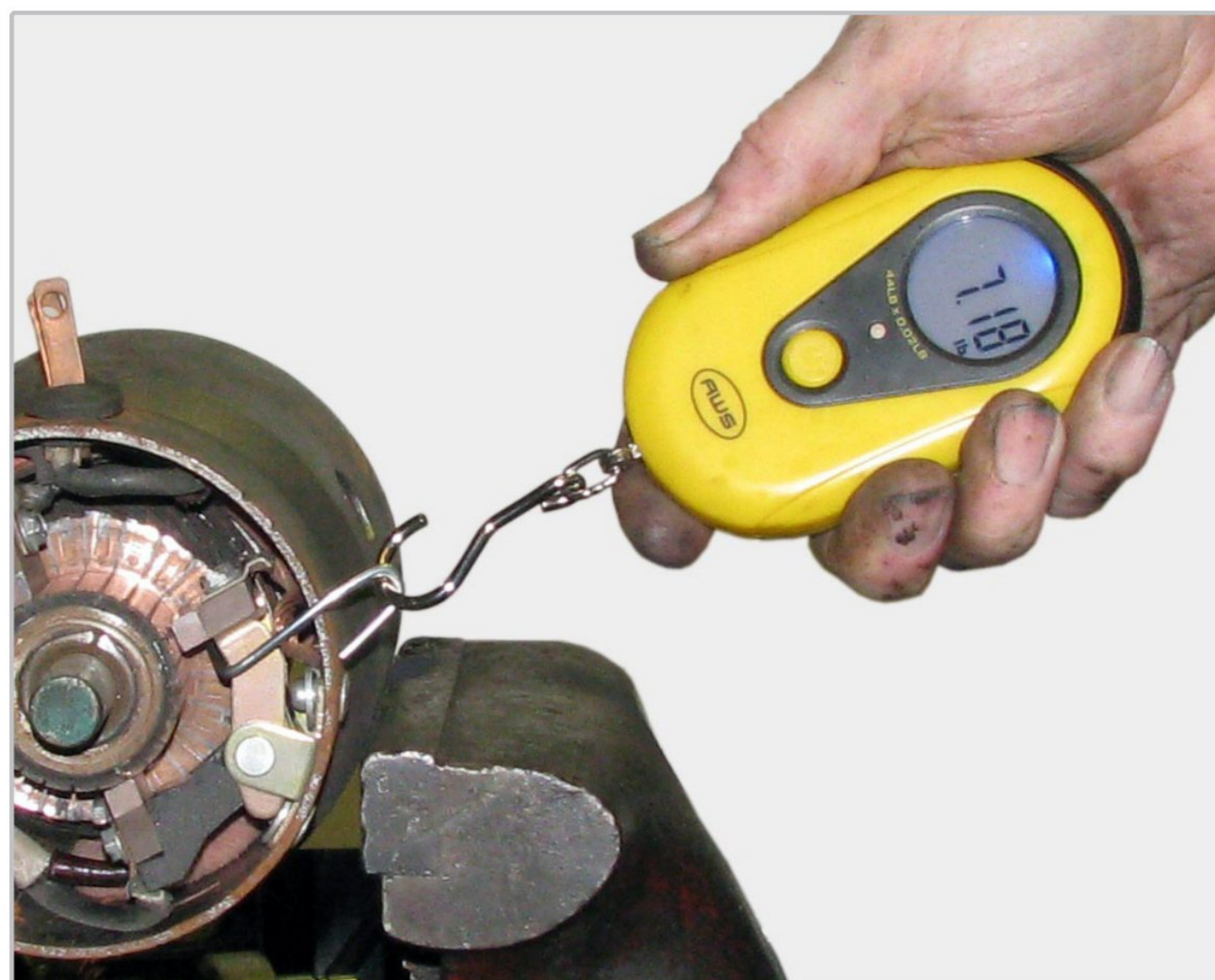
Figure 12—Testing a flat starter torsion-spring
