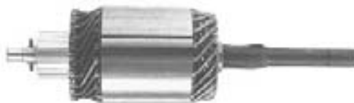
61-9202 Armature 12 Volt, CW Rotation, 17° Helix
