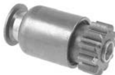
54-129 (Ref# 4-461) Starter Drive 11-T, CCW, 19-SPL, Positive Engagement
