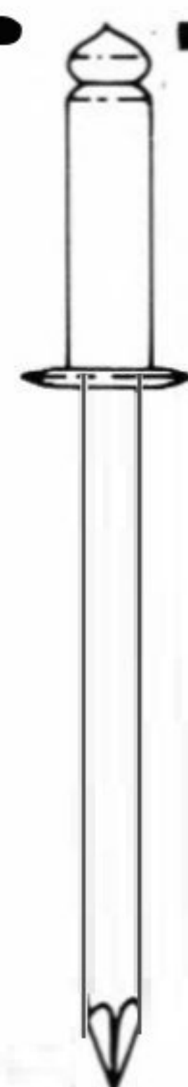
S-676 No. 7 .514 (33/64) Truss Carbon Steel
