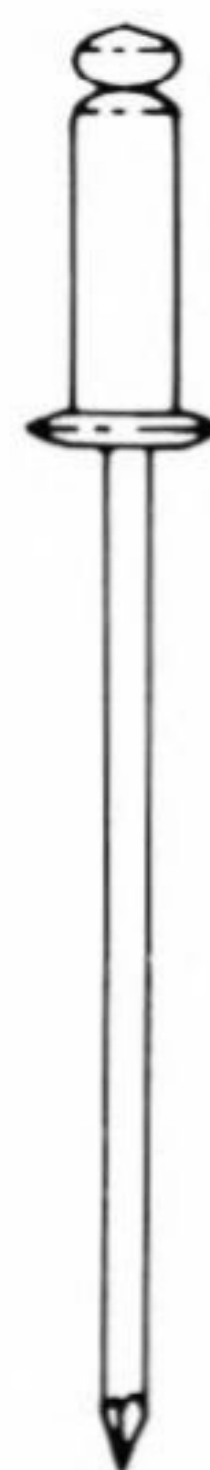
S-675 No. 5 .374 (3/8) Truss Carbon Steel
