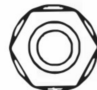
S-2545 10-24 x 3/8 Hex with attached Conical Washer .184 Thk. Cadmium Plated
