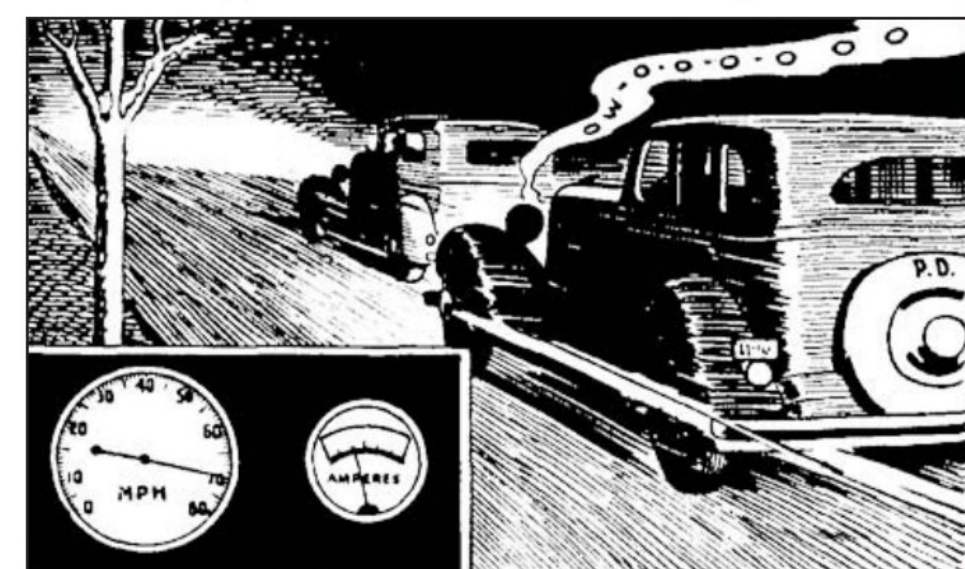
Figure 5a—Ammeter shows discharge at 70 M.P.H. with standard equipment generator
