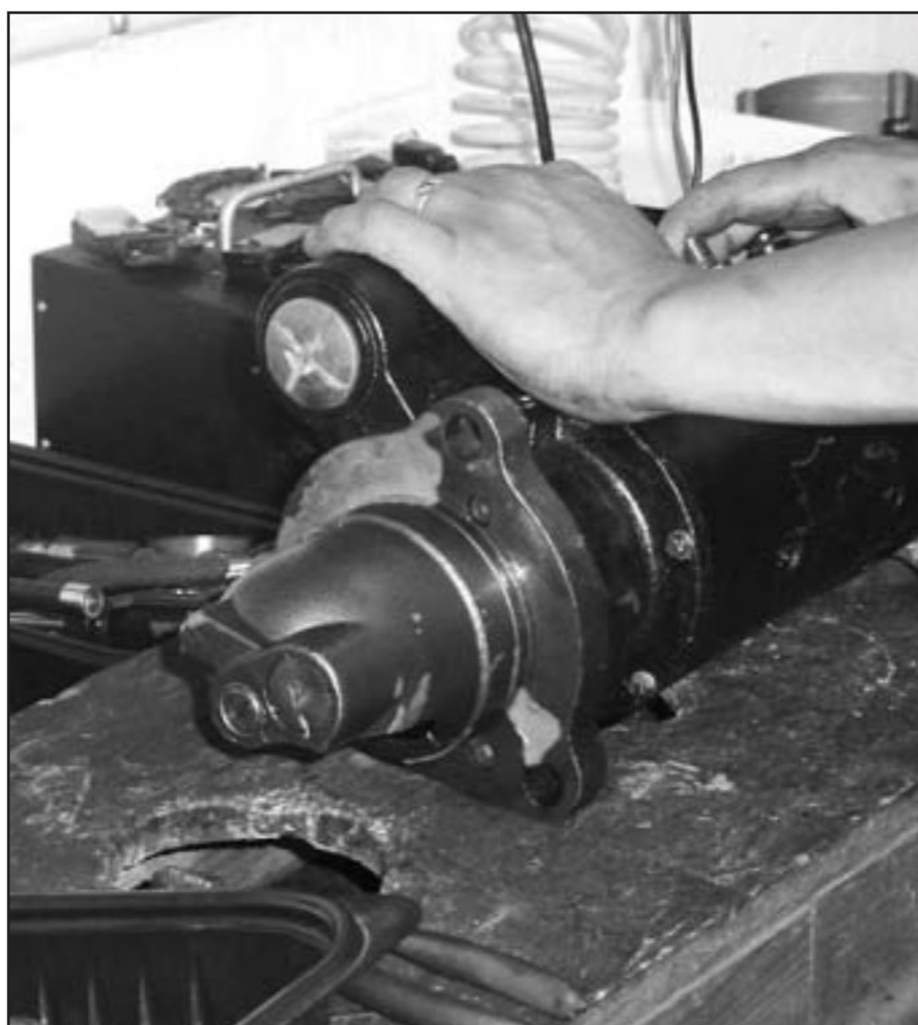
Enrique Olvera rebuilds a 40MT starter.
