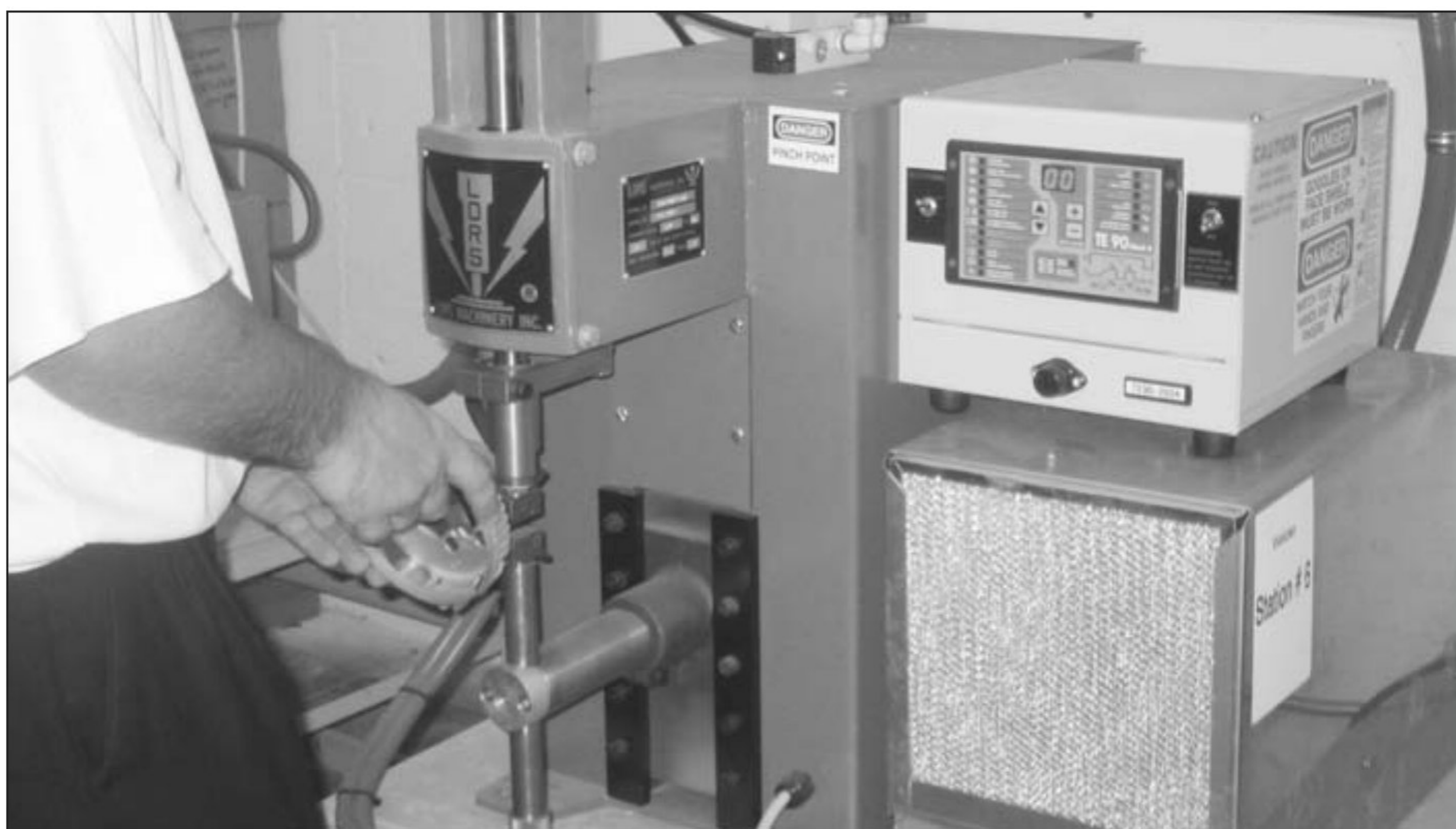
A Rand employee demonstrates rectifier welding at their electronics business.
