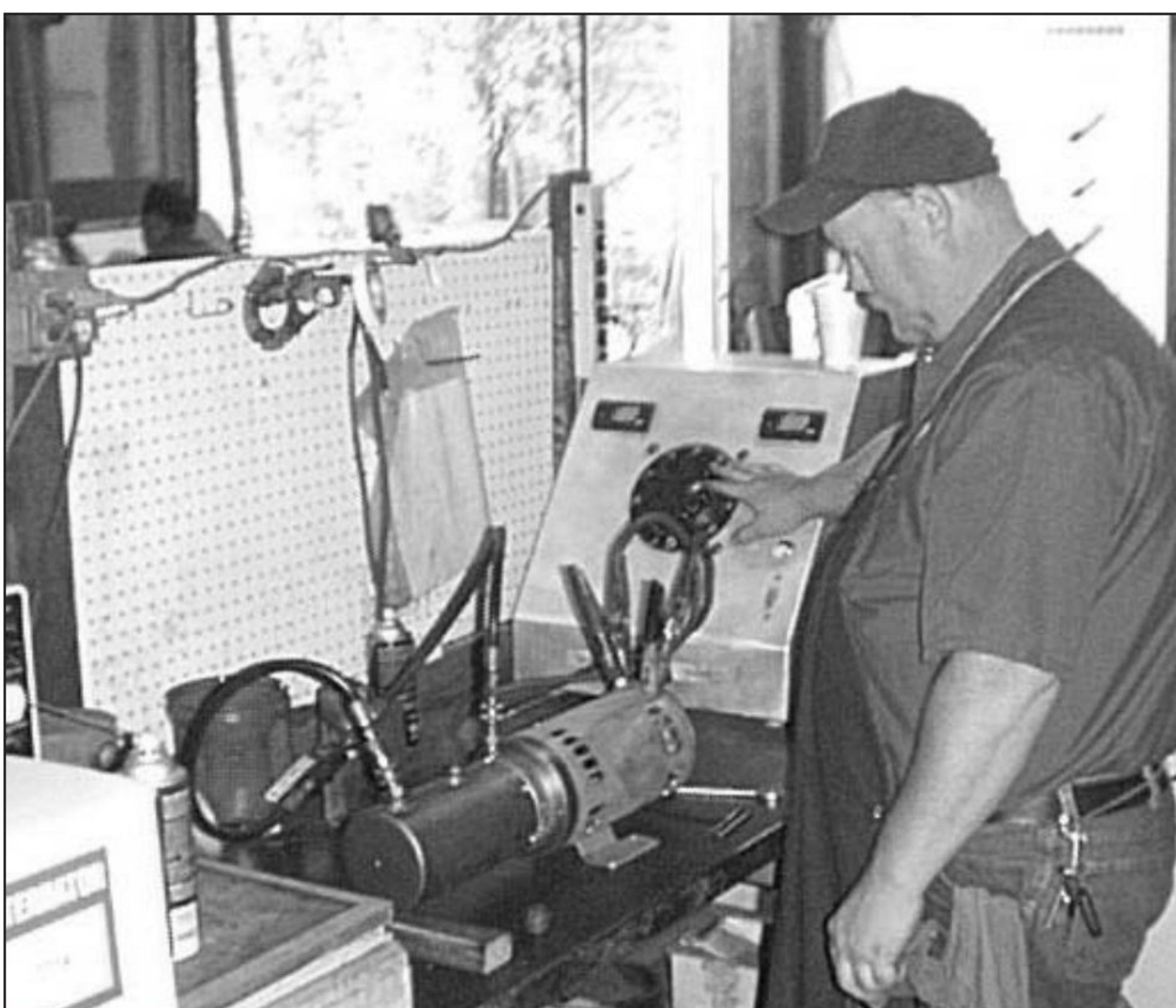
Tracy Duke tests 90-volt DC hydraulic pump motors when he's not rebuilding motors, heavy duty starters, alternators, and everything else when needed.
