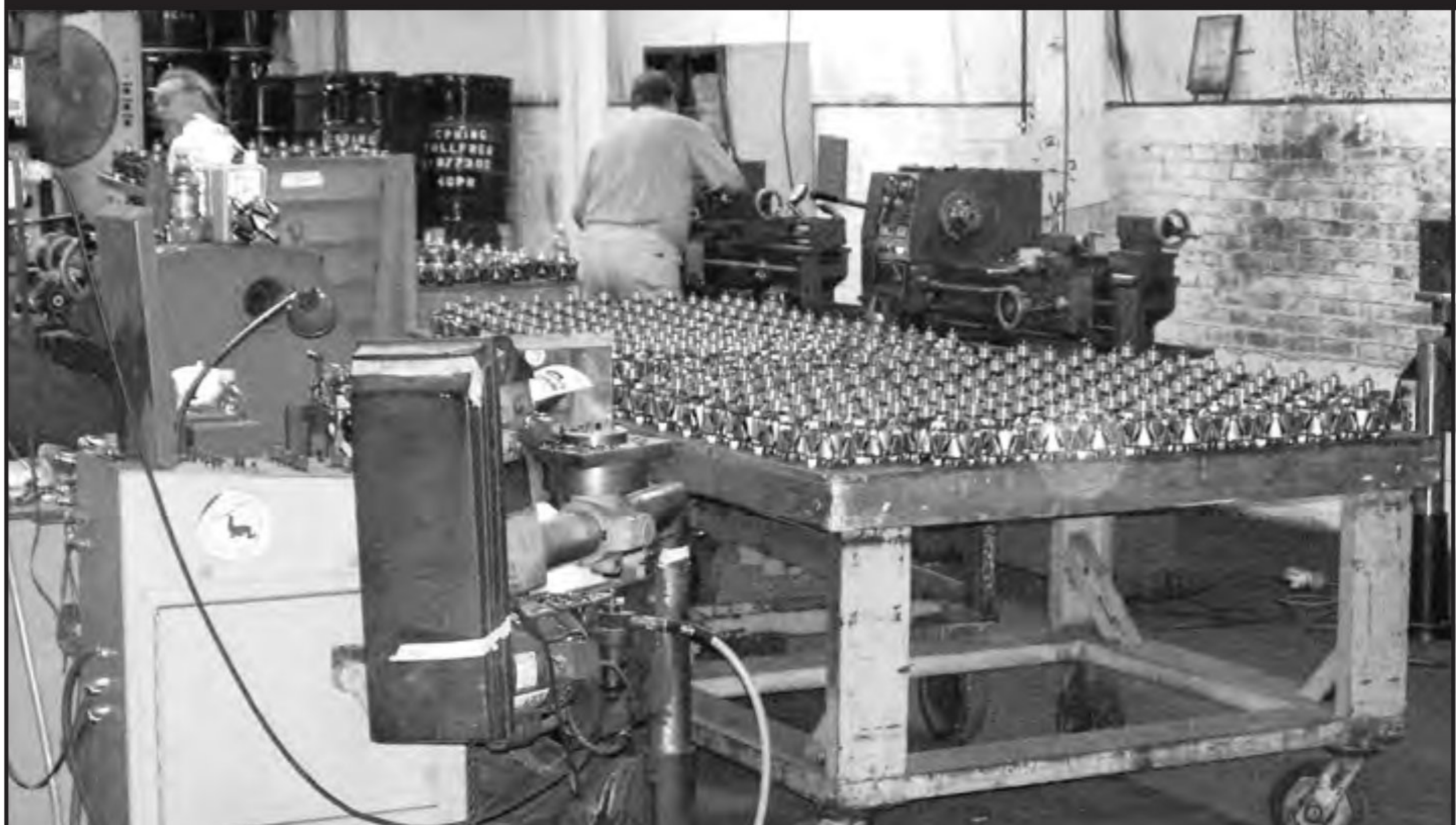
Component Production & Recovery racks up the rotors on their rotor finishing line, showing their balancer, drill press and lathe.
