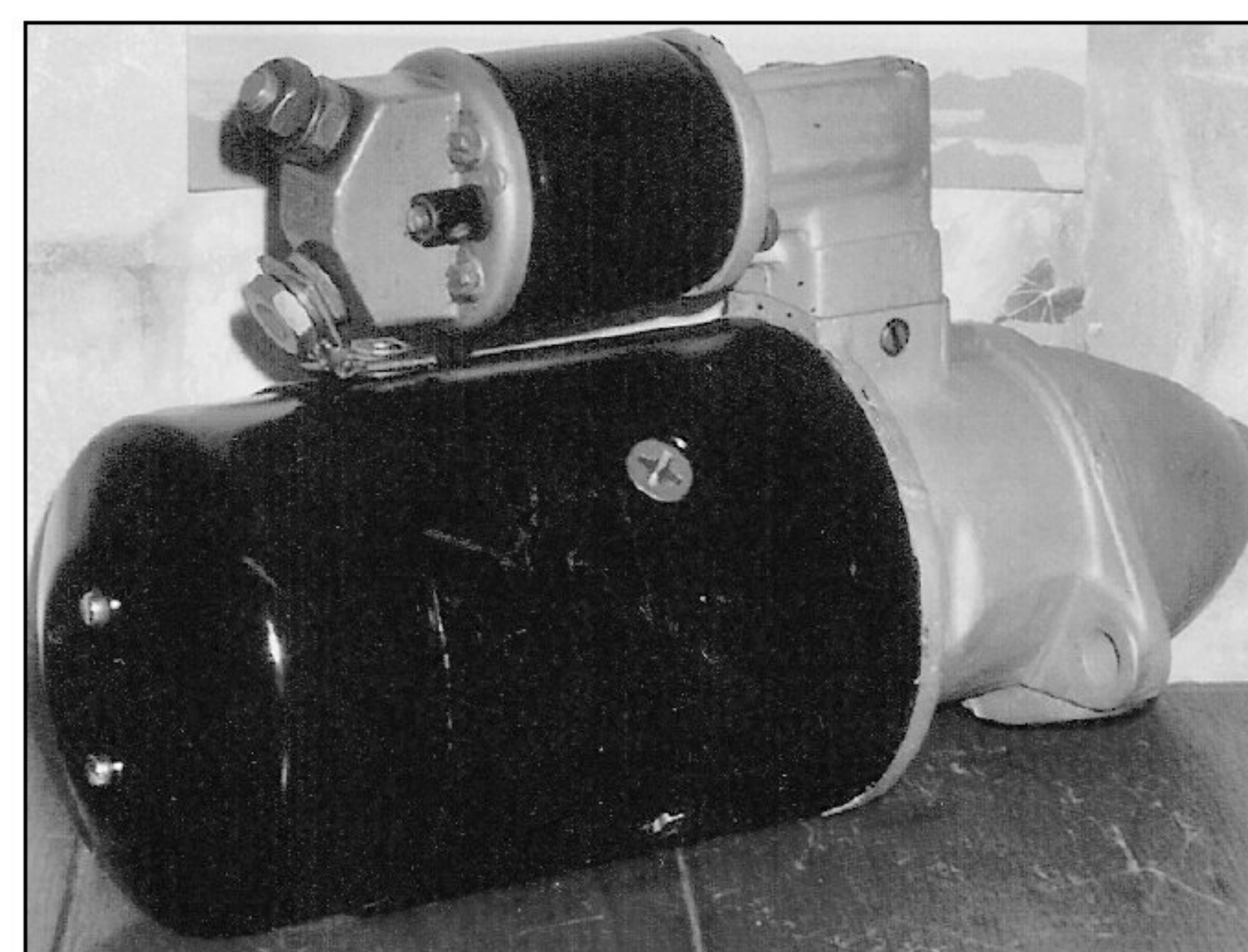
Marelli starter no. MT21F-18/12D9 for 1962 Ferrari Series II.
